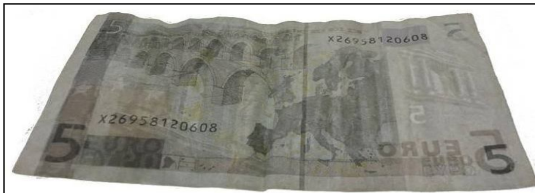
Figure 232: Paper banknote; five Euro (5 €) after coating by 3 rd layer of 1% carboxymethyl cellulose (CMC) after thermal ageing at 140 0 C through transmitted light (back side).
