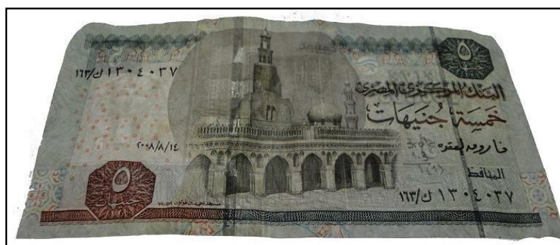
Figure 127: Paper banknote; Egyptian five pounds (5 EGP) after coating by 3 rd layer of 0.1% of carboxymethyl cellulose (CMC) after thermal ageing at 140 °C through transmitted light (front side).
