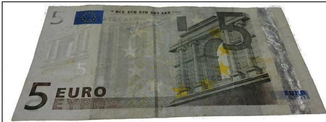
Figure 223: Paper banknote; five Euro (5 €) before treatment after thermal ageing at 140 °C through transmitted light (front side).
