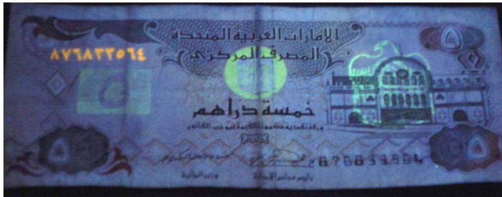
Figure 315: Paper banknote; 5 Dirham "AED" after coating by 3 rd layer of 1% of carboxymethyl cellulose (CMC) under UV radiation ( \lambda_2 = 336 \text{ nm} ) at 25 0 C through UV radiation (front side).
