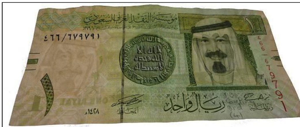
Figure 197: Paper banknote; one riyal (1 SAR) after coating by 3 rd layer of 1% carboxymethyl cellulose (CMC) through transmitted light (front side).
