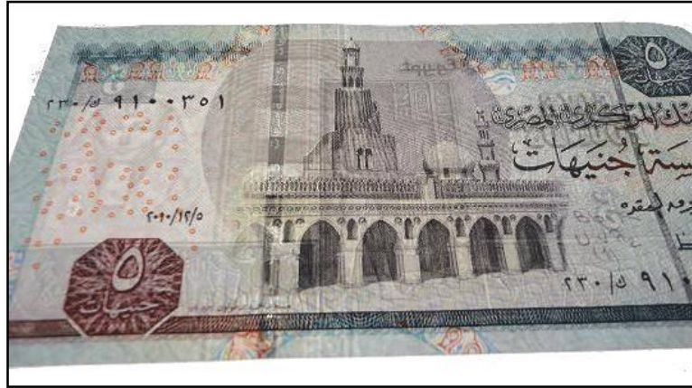
Figure 124: Paper banknote; Egyptian five pounds (5 EGP) before treatment under UV radiation ( \lambda_2 = 336 \text{ nm} ) at 25^\circ\text{C} through transmitted light (front side).
