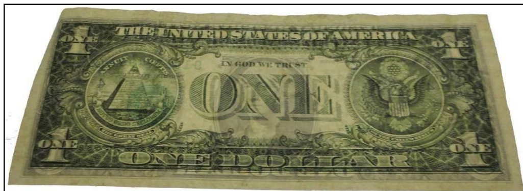
Figure 182: Paper banknote; one dollar (1U$) after coating by 3 rd layer of 1% of Carboxymethyl cellulose (CMC) through transmitted light (back side).
