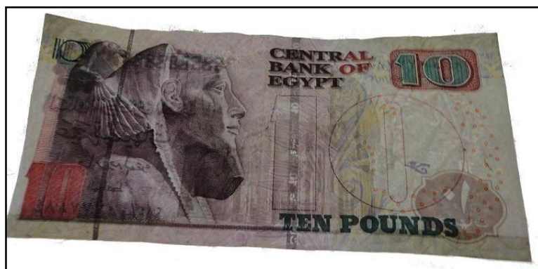
Figure 160: Paper banknote; Egyptian ten pounds (10 EGP) after coating by 3 rd layer of 1% of carboxymethyl cellulose (CMC) after thermal ageing at 140 °C through transmitted light (back side).
