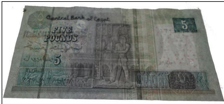
Figure 123: Paper banknote; Egyptian five pounds (5 EGP) before treatment under UV radiation ( \lambda_1 = 256 \text{ nm} ) at 25^{\circ}\text{C} through transmitted light (back side).
