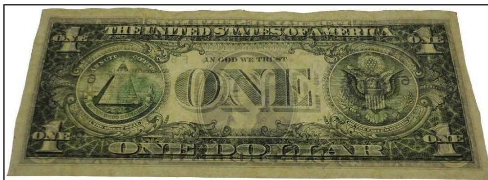
Figure 178: Paper banknote; one dollar (1U$) after coating by 3 rd layer of 0.1% of Carboxymethyl cellulose (CMC) under UV radiation ( \lambda_1 = 256 nm) through transmitted light (back side).
