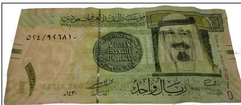
Figure 199: Paper banknote; one riyal (1 SAR) after coating by 3 rd layer of 1% carboxymethyl cellulose (CMC) after thermal ageing at 140 °C through transmitted light (front side).
