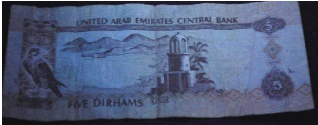
Figure 314: Paper banknote; 5 Dirham "AED" after coating by 3 rd layer of 1% of carboxymethyl cellulose (CMC) under UV radiation ( \lambda_1 = 256 \text{ nm} ) at 25 0 C through UV radiation (back side).
