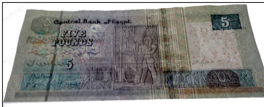
Figure 134: Paper banknote; Egyptian five pounds (5 EGP) after coating by 3 rd layer of 1% of carboxymethyl cellulose (CMC) through transmitted light (back side).
