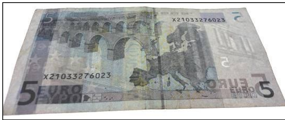
Figure 228: Paper banknote; five Euro (5 €) before treatment under UV radiation ( \lambda_2 = 336 \text{ nm} ) at 25^{\circ}\text{C} through transmitted light (back side)
