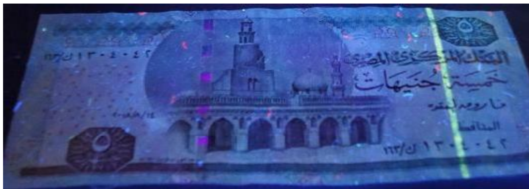
Figure 251: Paper banknote; Egyptian five pounds (5 EGP) after coating by 3 rd layer of 1% of carboxymethyl cellulose (CMC) under UV radiation ( \lambda_2 = 336 \text{ nm} ) at 25 0 C through UV radiation (front side)
