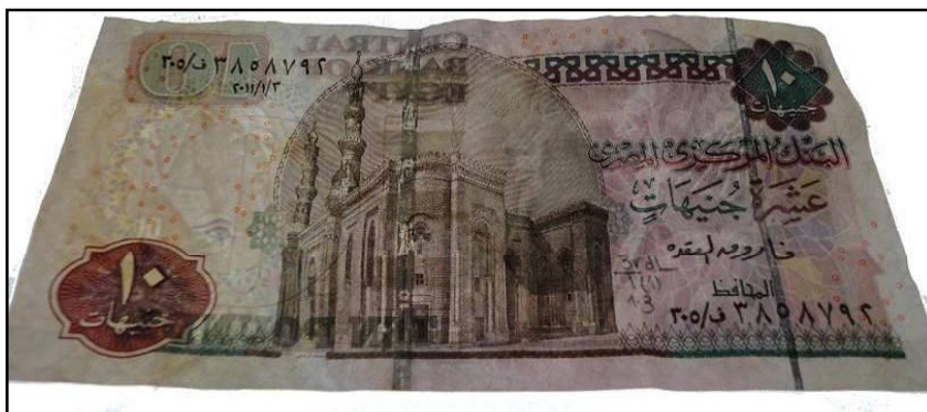
Figure 151: Paper banknote; Egyptian ten pounds (10 EGP) after coating by 3 rd layer of 0.1% of carboxymethyl cellulose (CMC) after thermal ageing at 140 °C through transmitted light (front side).
