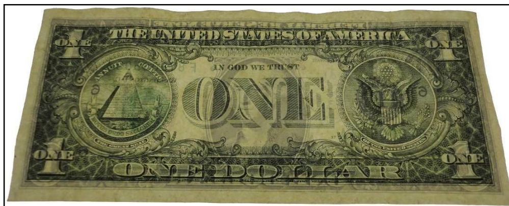
Figure 188: Paper banknote; one dollar (1U$) after coating by 3 rd layer of 1 % of Carboxymethyl cellulose (CMC) under UV radiation ( \lambda_2 = 336 nm) through transmitted light (back side).
