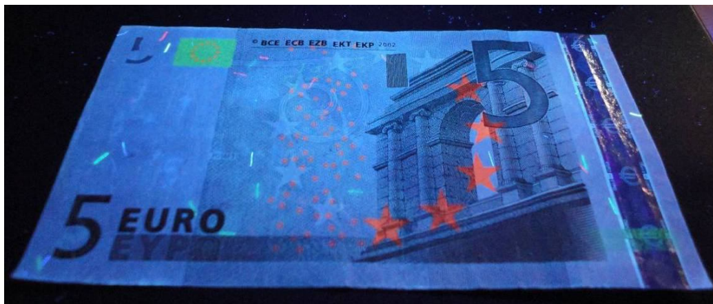
Figure 323: Paper banknote; 5 Euro "€" before treatment under UV radiation ( \lambda_2 = 336 nm) at 25^0 C through UV radiation (front side).
