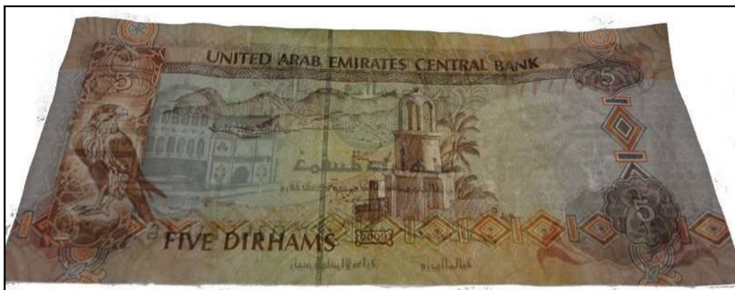
Figure 218: Paper banknote; five Dirhams (5 AED) after coating by 3 rd layer of 1% carboxymethyl cellulose (CMC) of 1% under UV radiation ( \lambda_1 = 256 nm) through transmitted light (back side).
