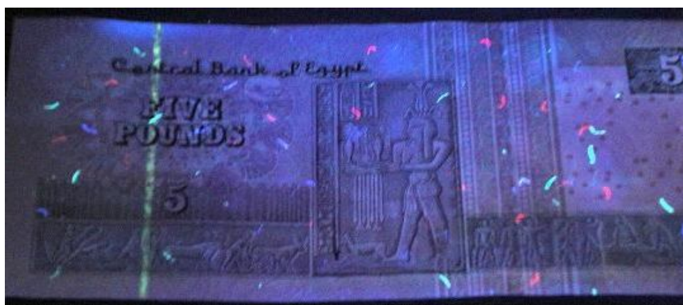
Figure 250: Paper banknote; Egyptian five pounds (5 EGP) after coating by 3 rd layer of 1% of carboxymethyl cellulose (CMC) under UV radiation ( \lambda_1 = 256 \text{ nm} ) at 25 °C through UV radiation (back side).
