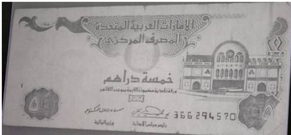
Figure 411: Paper banknote; 5 Dirham "AED" after coating by 3 rd layer of 1% of carboxymethyl cellulose (CMC) under IR radiation ( \lambda_2 = 336 \text{ nm} ) at 25 o C through IR radiation (front side).
