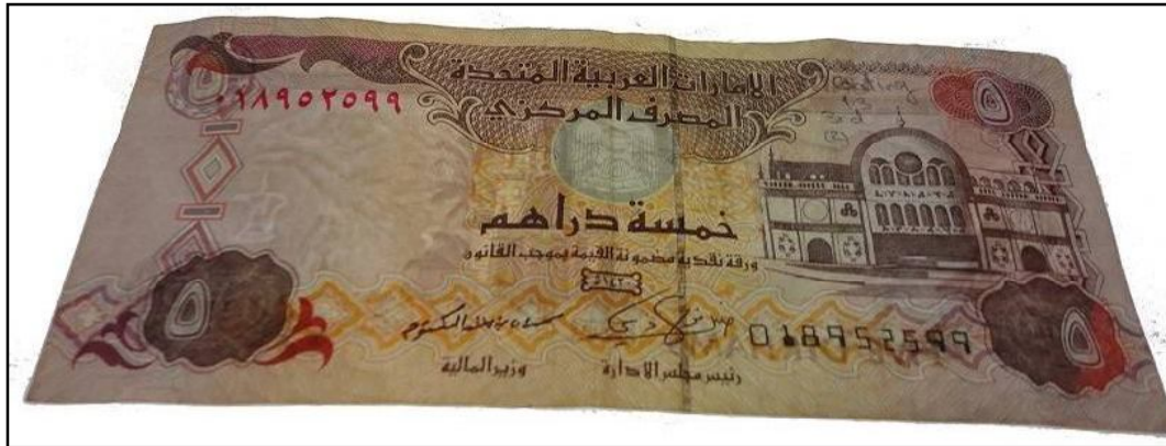
Figure 219: Paper banknote; five Dirhams (5 AED) after coating by 3 rd layer of 1% carboxymethyl cellulose (CMC) of 1% under UV radiation ( \lambda_2 = 336 nm) through transmitted light (front side).
