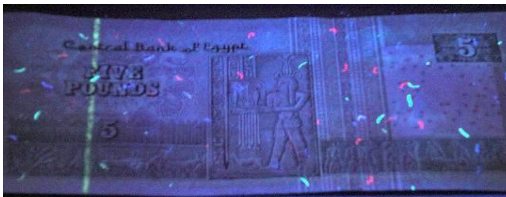
Figure 246: Paper banknote; Egyptian five pounds (5 EGP) after coating by 3 rd layer of 1% of carboxymethyl cellulose (CMC) through UV radiation (back side).
