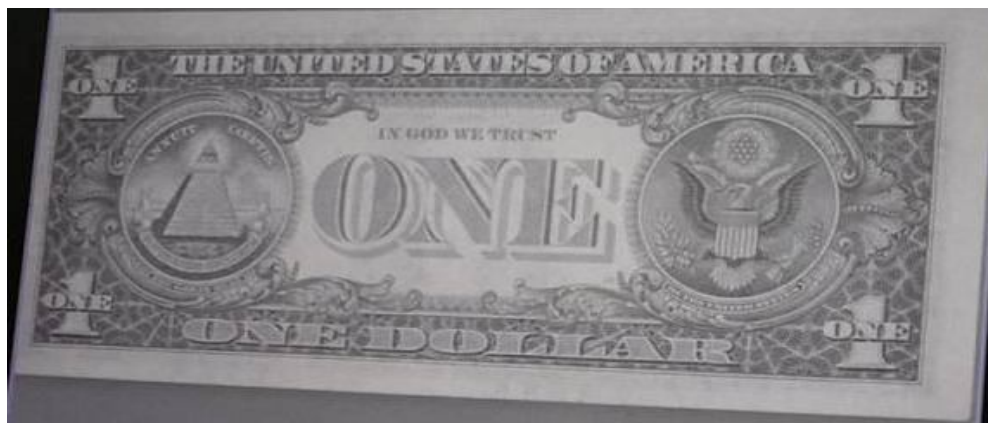
Figure 376: Paper banknote; One dollar (1U$) after coating by 3 rd layer of 1% of carboxymethyl cellulose (CMC) after thermal ageing at 140 °C through IR radiation (back side).
