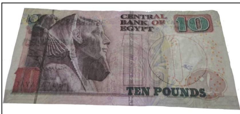
Figure 146: Paper banknote; Egyptian ten pounds (10 EGP) before treatment under UV radiation ( \lambda_1 = 256\text{ nm} ) at 25^{\circ}\text{C} through transmitted light (back side).
