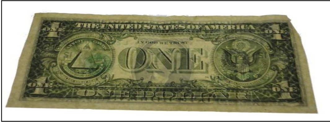
Figure 168: Paper banknote; One dollar (1U$) before treatment after thermal ageing at 140^{\circ}\text{C} through transmitted light (back side)
