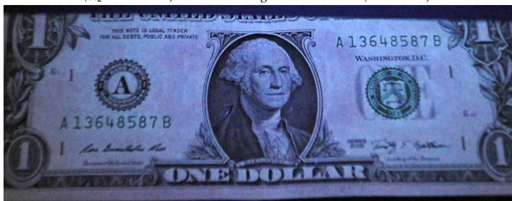
Figure 277: Paper banknote; One dollar (1U$) after coating by 3 rd layer of 1% of carboxymethyl cellulose (CMC) through UV radiation (front side).
