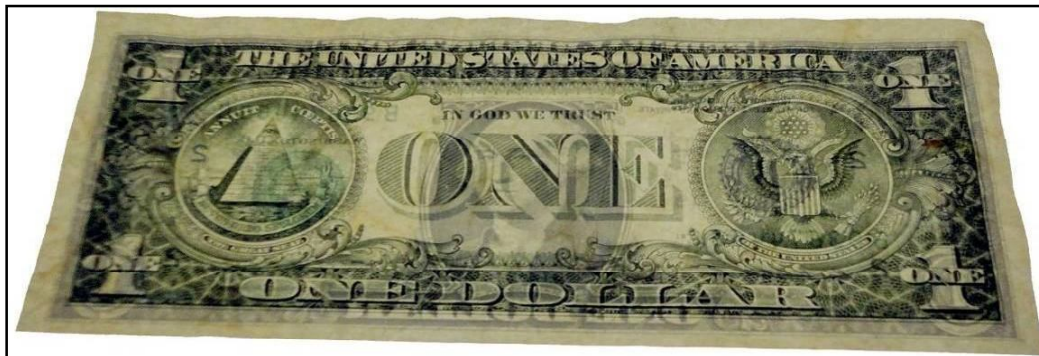
Figure 180: Paper banknote; one dollar (1U$) after coating by 3 rd layer of 0.1% of Carboxymethyl cellulose (CMC) under UV radiation ( \lambda_2 = 336 nm) through transmitted light (back side).
