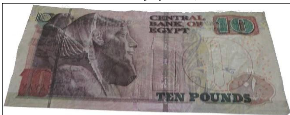
Figure 164: Paper banknote; Egyptian ten pounds (10 EGP) after coating by 3 rd layer of 1% of carboxymethyl cellulose (CMC) under UV radiation ( \lambda_2 = 336 nm) through transmitted light (back side).
