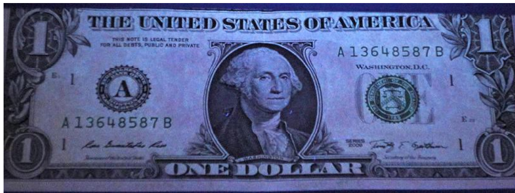
Figure 281: Paper banknote; One dollar (1U$) after coating by 3 rd layer of 1% of carboxymethyl cellulose (CMC) under UV radiation ( \lambda_1 = 256 \text{ nm} ) at 25 o C through UV radiation (front side).
