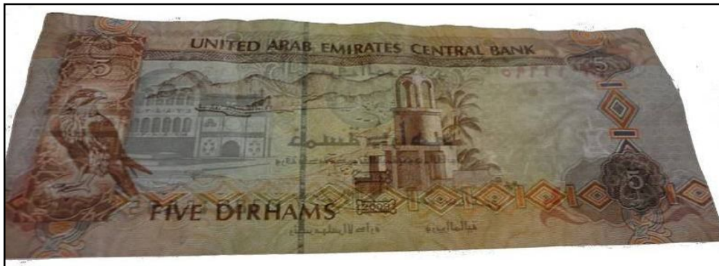
Figure 216: Paper banknote; five Dirhams (5 AED) after coating by 3 rd layer of 1% of carboxymethyl cellulose (CMC) after thermal ageing at 140 °C through transmitted light (back side).
