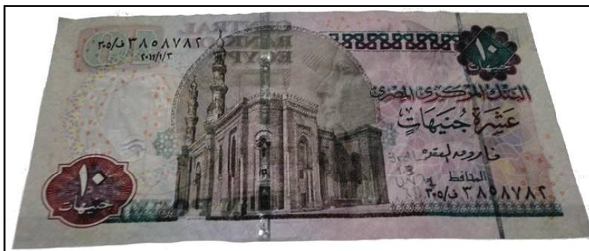
Figure 149: Paper banknote; Egyptian ten pounds (10 EGP) after coating by 3 rd layer of 0.1% of carboxymethyl cellulose (CMC) through transmitted light (front side).
