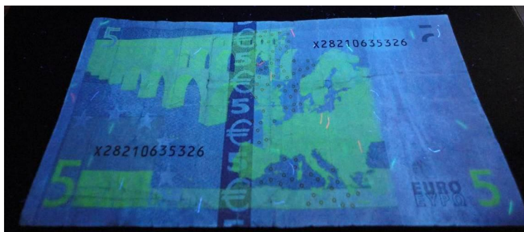
Figure 322: Paper banknote; 5 Euro "€" before treatment under UV radiation ( \lambda_1 = 256 nm) at 25^{\circ}\text{C} through UV radiation (back side).
