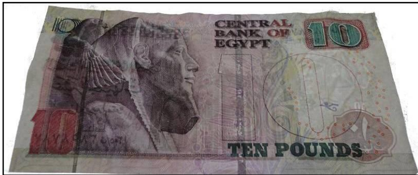
Figure 154: Paper banknote; Egyptian ten pounds (10 EGP) after coating by 3 rd layer of 0.1% of carboxymethyl cellulose (CMC) under UV radiation ( \lambda_1 = 256 \text{ nm} ) at 25 °C through transmitted light (back side).
