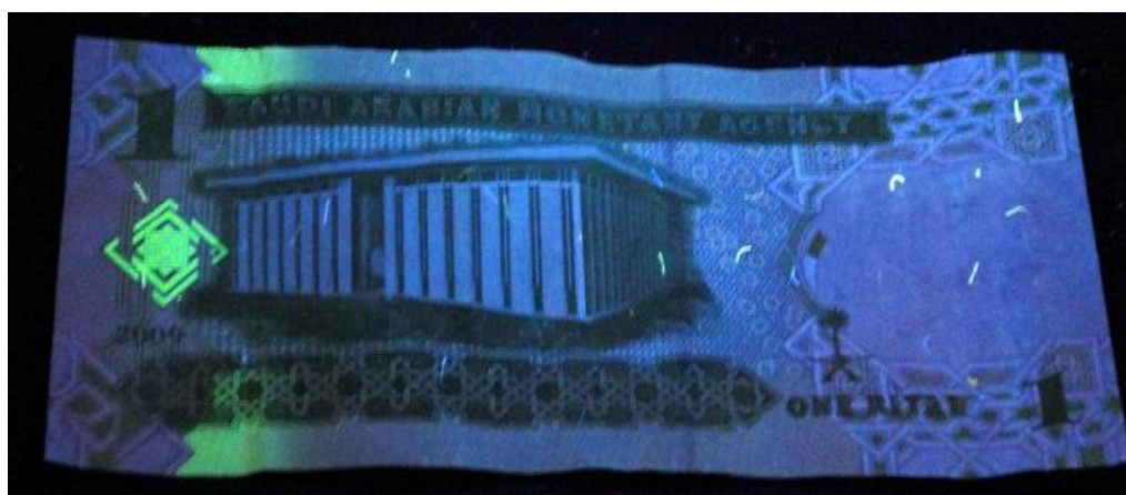
Figure 292: Paper banknote; One riyal (1 SAR) before treatment under UV radiation ( \lambda_2 = 336 \text{ nm} ) at 25^\circ\text{C} through UV radiation (back side).
