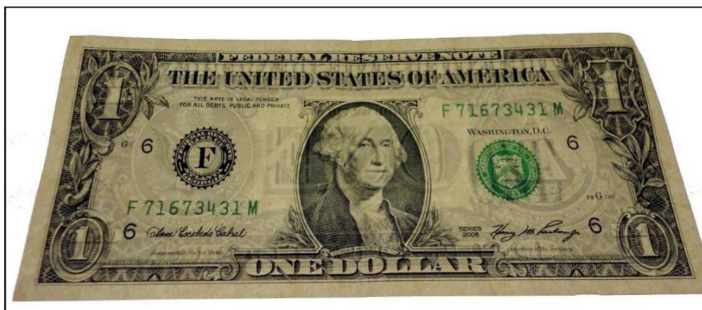
Figure 173: Paper banknote; one dollar (1US) after coating by 3 rd layer of 0.1% of Carboxymethyl cellulose (CMC) through transmitted light (front side).
