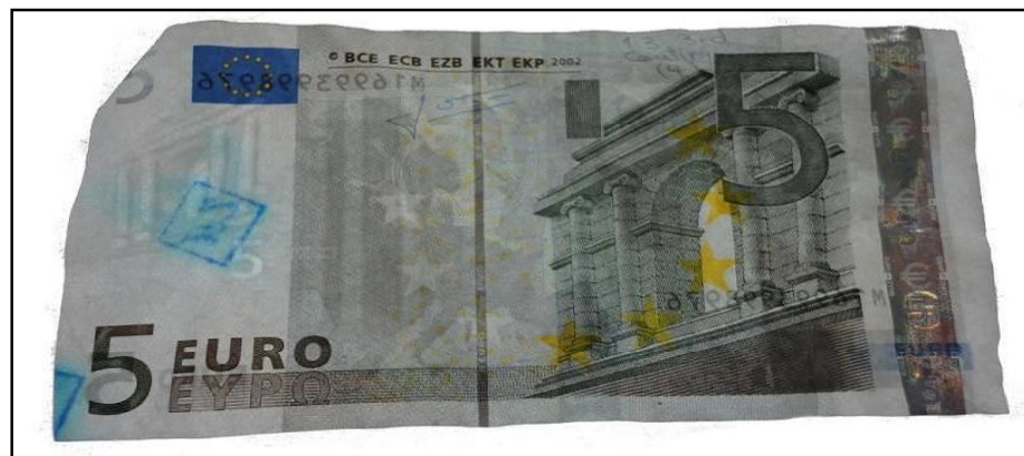
Figure 229: Paper banknote; five Euro (5 €) after coating by 3 rd layer of 1% carboxymethyl cellulose (CMC) through transmitted light (front side).
