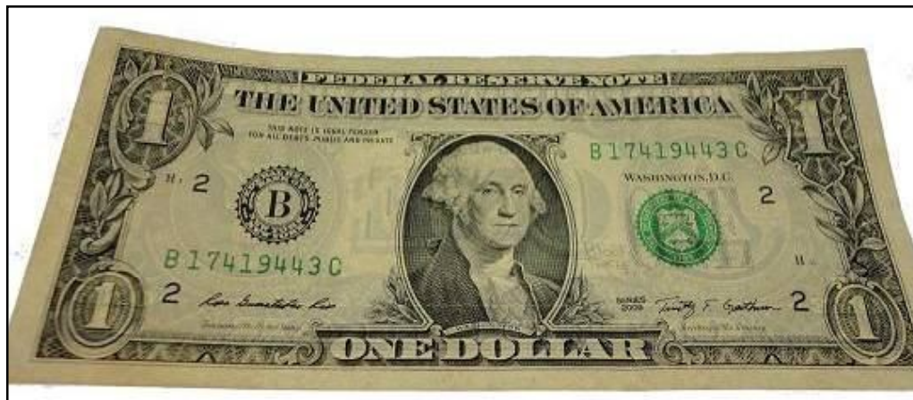
Figure 167: Paper banknote; One dollar (1U$) before treatment after thermal ageing at 140 °C through transmitted light (front side).
