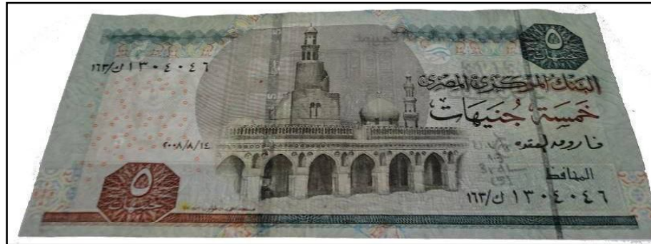
Figure 129: Paper banknote; Egyptian five pounds (5 EGP) after coating by 3 rd layer of 0.1% of carboxymethyl cellulose (CMC) under UV radiation ( \lambda_1 = 256 \text{ nm} ) at 25 °C through transmitted light (front side).
