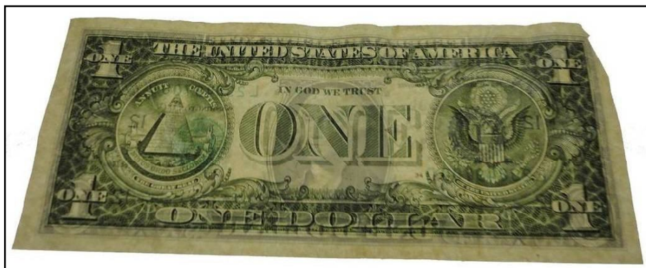
Figure 174: Paper banknote; one dollar (1U$) after coating by 3 rd layer of 0.1% of Carboxymethyl cellulose (CMC) through transmitted light (back side).
