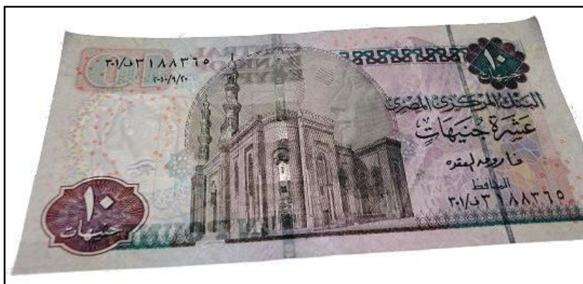
Figure 145: Paper banknote; Egyptian ten pounds (10 EGP) before treatment under UV radiation ( \lambda_1 = 256\text{ nm} ) at 25^{\circ}\text{C} through transmitted light (front side).
