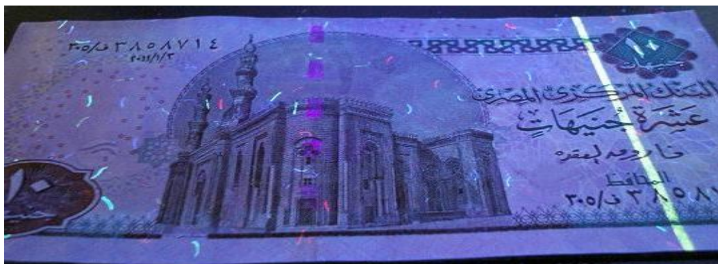
Figure 261: Paper banknote; Egyptian ten pounds (10 EGP) after coating by 3 rd layer of 1% of carboxymethyl cellulose (CMC) through UV radiation (front side).
