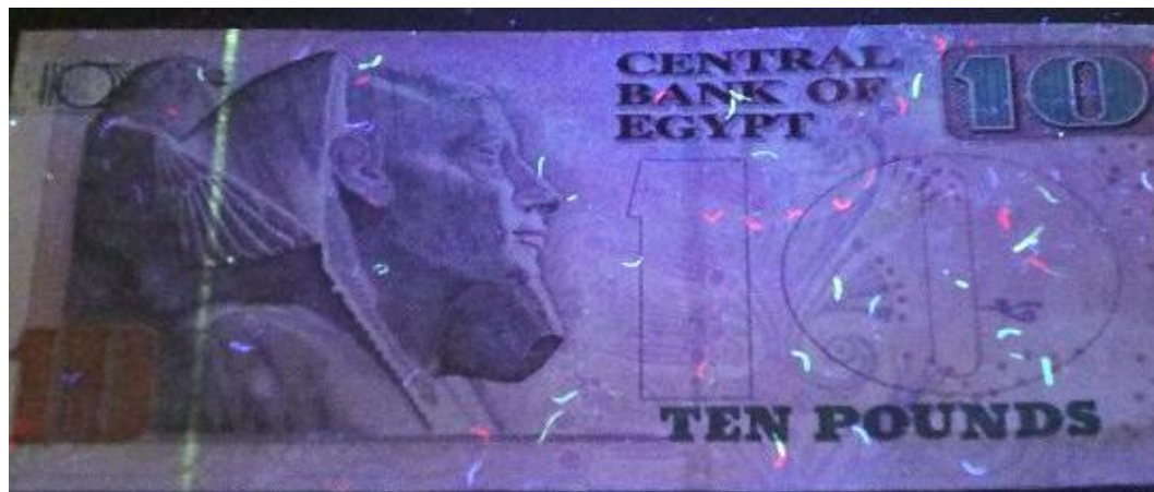
Figure (268): Paper banknote; Egyptian ten pounds (10 EGP) after coating by 3 rd layer of 1% of carboxymethyl cellulose (CMC) under UV radiation ( \lambda_2 = 336 \text{ nm} ) at 25 o C through UV radiation (back side).
