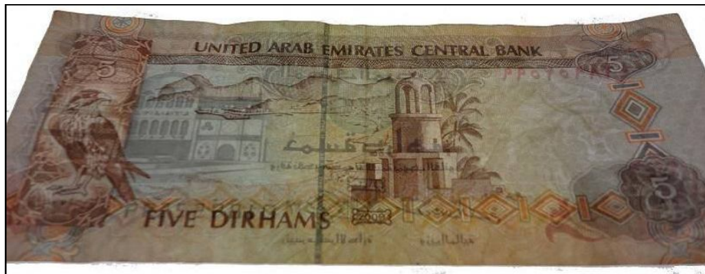
Figure 220: Paper banknote; five Dirhams (5 AED) after coating by 3 rd layer of 1% carboxymethyl cellulose (CMC) of 1% under UV radiation ( \lambda_2 = 336 nm) through transmitted light (back side).
