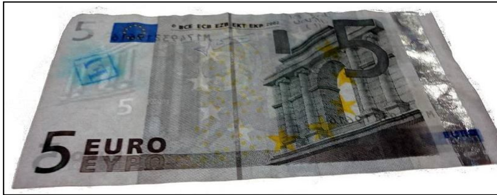
Figure 233: Paper banknote; five Euro (5 €) after coating by 3 rd layer of 1% carboxymethyl cellulose (CMC) under UV radiation ( \lambda_1 = 256 \text{ nm} ) at 25 0 C through transmitted light (front side).
