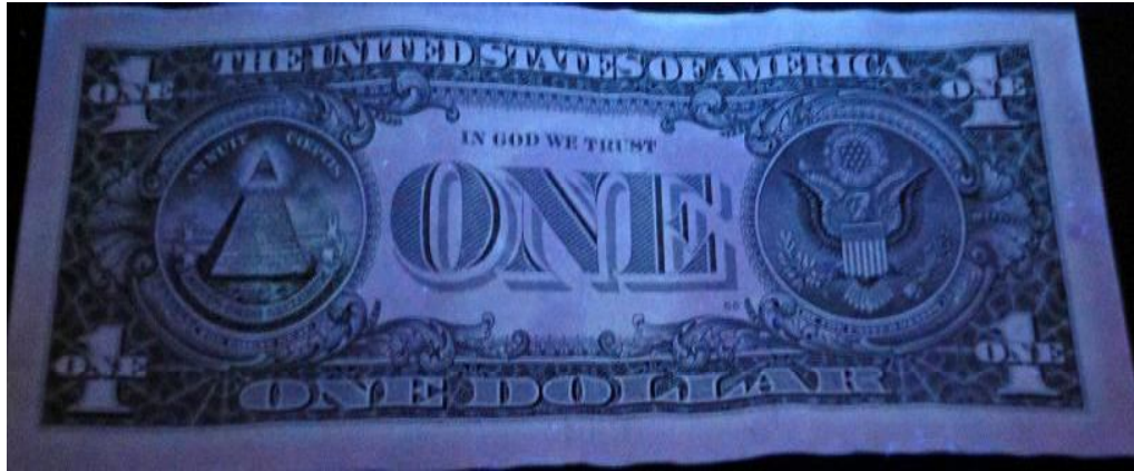
Figure (272): Paper banknote; One dollar (1U$) before treatment after thermal ageing at 140^{\circ}\text{C} through UV radiation (back side).
