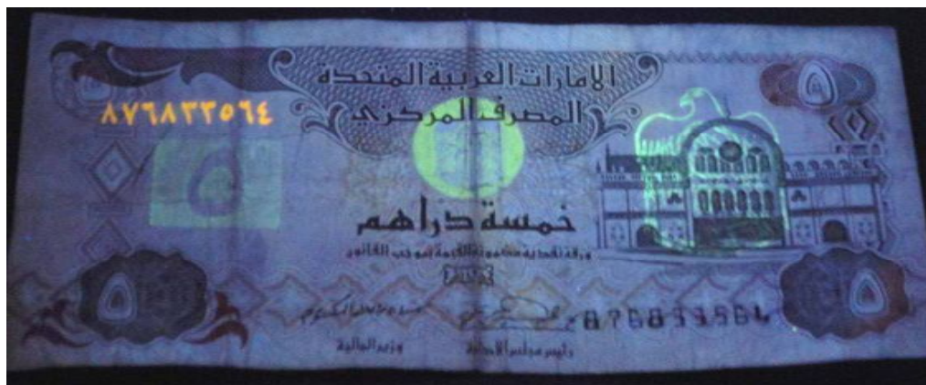
Figure 311: Paper banknote; 5 Dirham "AED" after coating by 3 rd layer of 1% of carboxymethyl cellulose (CMC) after thermal ageing at 140 °C through UV radiation (front side).
