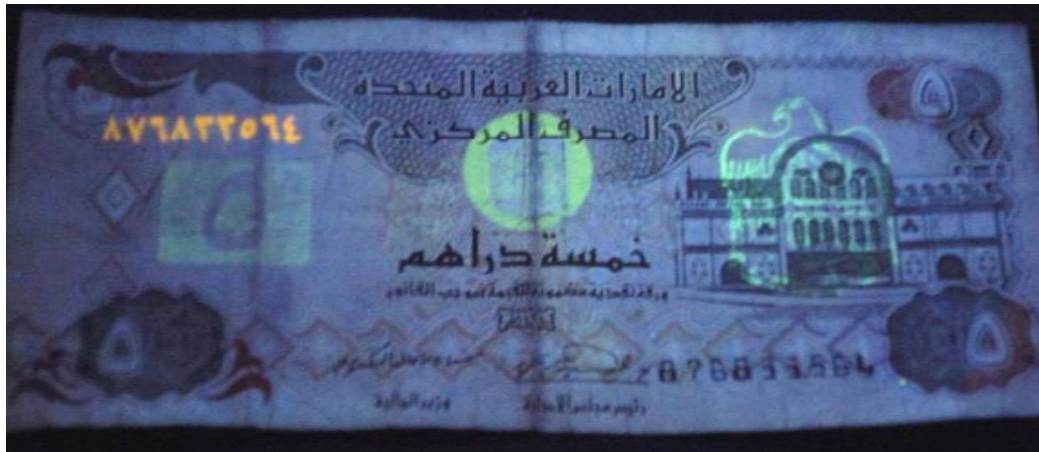
Figure 309: Paper banknote; 5 Dirham "AED" after coating by 3 rd layer of 1% of carboxymethyl cellulose (CMC) through UV radiation (front side).
