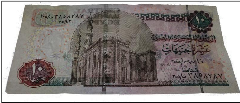
Figure 153: Paper banknote; Egyptian ten pounds (10 EGP) after coating by 3 rd layer of 0.1% of carboxymethyl cellulose (CMC) under UV radiation ( \lambda_1 = 256 \text{ nm} ) at 25 °C through transmitted light (front side)
