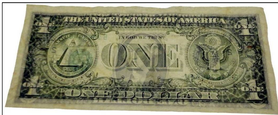
Figure 176: Paper banknote; one dollar (1U$) after coating by 3 rd layer of 0.1% of Carboxymethyl cellulose (CMC) after thermal ageing 140 °C through transmitted light (back side).
