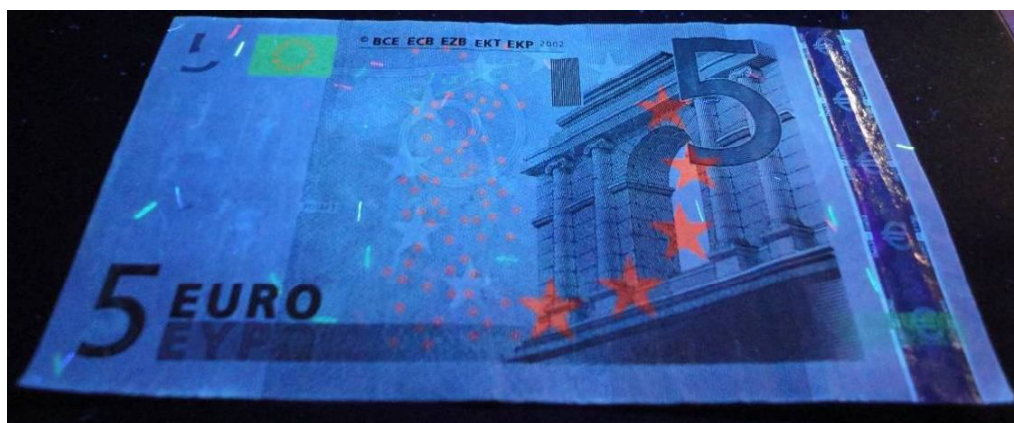
Figure 321: Paper banknote; 5 Euro "€" before treatment under UV radiation ( \lambda_1 = 256 nm) at 25^{\circ}\text{C} through UV radiation (front side)
