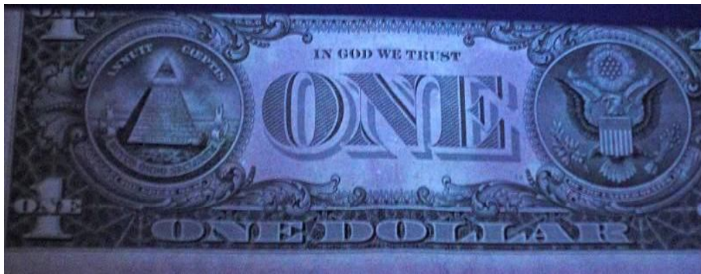
Figure 278: Paper banknote; One dollar (1U$) after coating by 3 rd layer of 1% of carboxymethyl cellulose (CMC) through UV radiation (back side).
