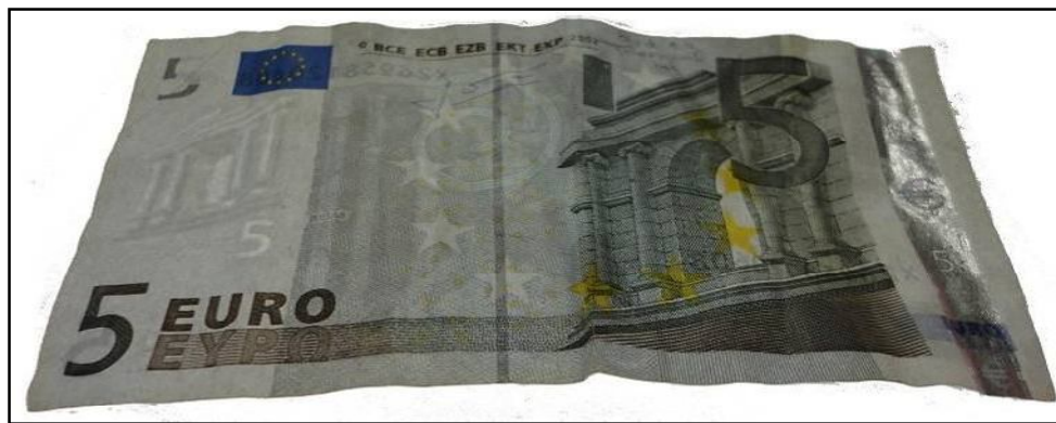
Figure 231: Paper banknote; five Euro (5 €) after coating by 3 rd layer of 1% carboxymethyl cellulose (CMC) after thermal ageing at 140 0 C through transmitted light (front side)
