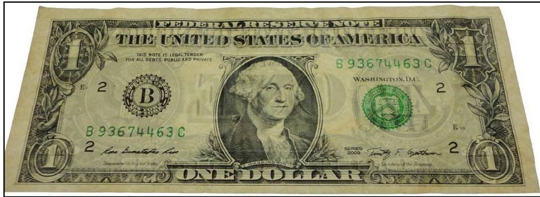
Figure 183: Paper banknote; one dollar (1U$) after coating by 3 rd layer of 1% of Carboxymethyl cellulose (CMC) after thermal ageing 140 °C through transmitted light (front side).
