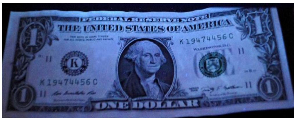
Figure 279: Paper banknote; One dollar (1U$) after coating by 3 rd layer of 1% of carboxymethyl cellulose (CMC) after thermal ageing at 140 °C through UV radiation (front side).
