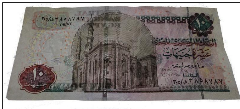
Figure 157: Paper banknote; Egyptian ten pounds (10 EGP) after coating by 3 rd layer of 1% of carboxymethyl cellulose (CMC) through transmitted light (front side).
