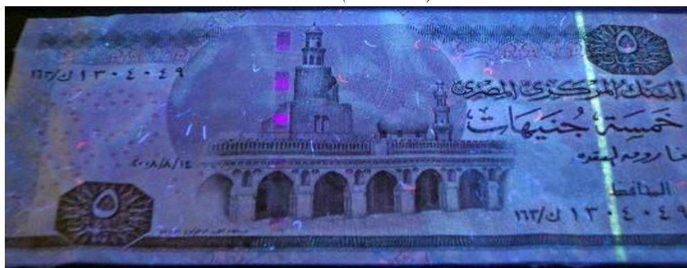
Figure 249: Paper banknote; Egyptian five pounds (5 EGP) after coating by 3 rd layer of 1% of carboxymethyl cellulose (CMC) under UV radiation ( \lambda_1 = 256 \text{ nm} ) at 25 °C through UV radiation (front side)
