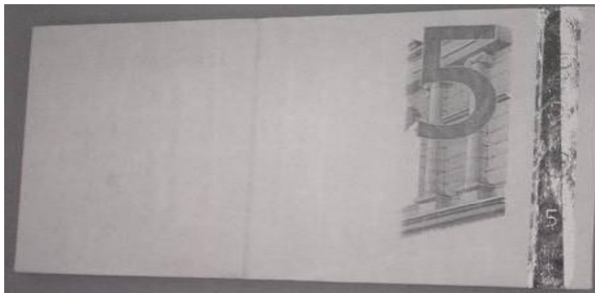
Figure 423: Paper banknote; 5 Euro "€" after coating by 3 rd layer of 1% of carboxymethyl cellulose (CMC) after thermal ageing at 140 °C through IR radiation (front side).
