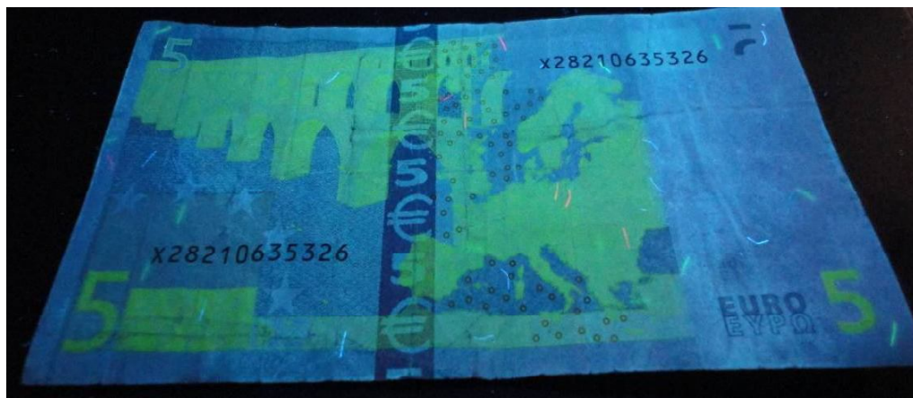
Figure 328: Paper banknote; 5 Euro "€" after coating by 3 rd layer of 1% of carboxymethyl cellulose (CMC) after thermal ageing at 140 0 C through UV radiation (back side).
