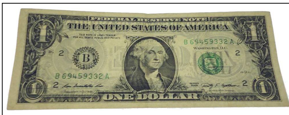
Figure 185: Paper banknote; one dollar (1U$) after coating by 3 rd layer of 1 % of Carboxymethyl cellulose (CMC) under UV radiation ( \lambda_1 = 256 \text{ nm} ) through transmitted light (front side).
