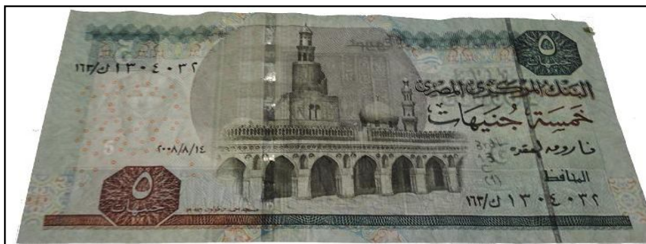
Figure 135: Paper banknote; Egyptian five pounds (5 EGP) after coating by 3 rd layer of 1% of carboxymethyl cellulose (CMC) after thermal ageing at 140 0 C through transmitted light (front side).
