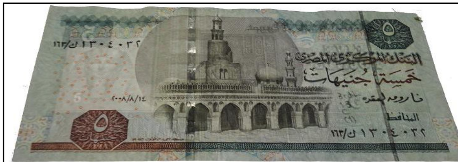
Figure 139: Paper banknote; Egyptian five pounds (5 EGP) after coating by 3 rd layer of 1% of carboxymethyl cellulose (CMC) under UV radiation ( \lambda_2 = 336 nm) through transmitted light (front side).
