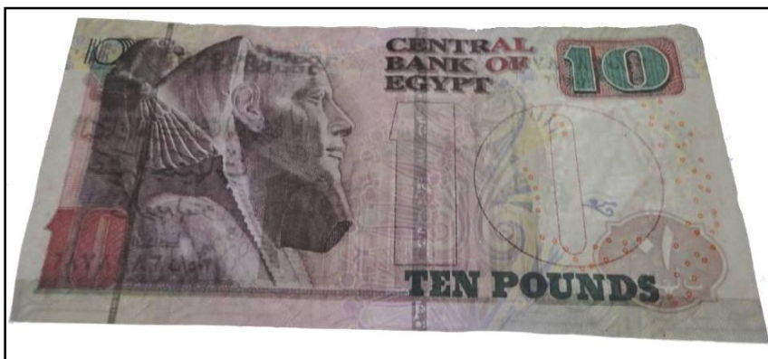
Figure 144: Paper banknote; Egyptian ten pounds (10 EGP) before treatment after thermal ageing at 140^{\circ}\text{C} through transmitted light (back side).
