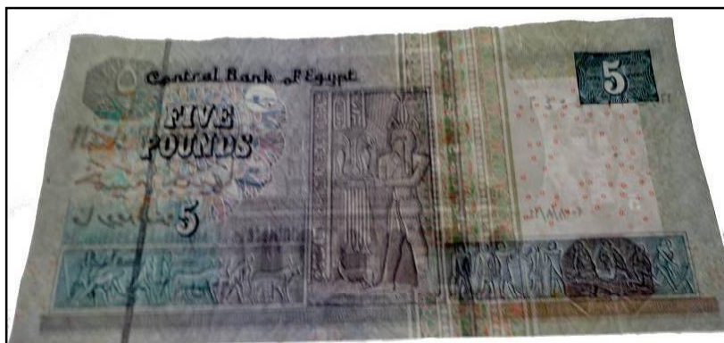
Figure 126: Paper banknote; Egyptian five pounds (5 EGP) after coating by 3 rd layer of 0.1% of carboxymethyl cellulose (CMC) through transmitted light (back side).
