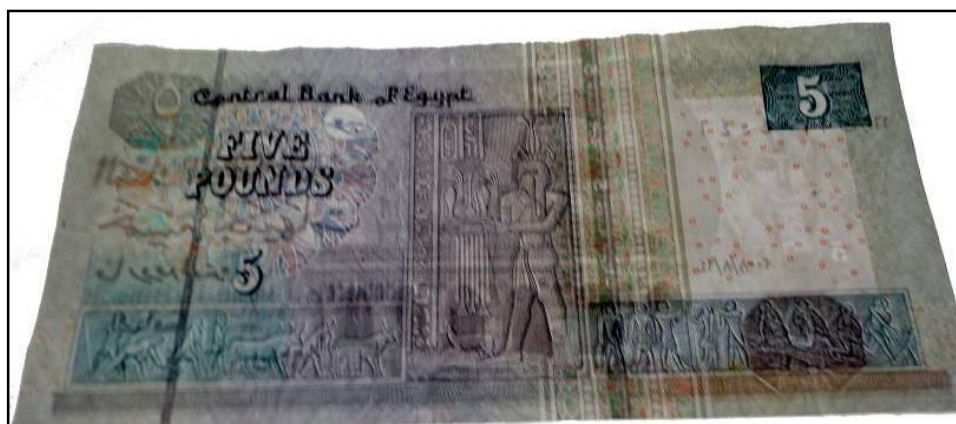
Figure 136: Paper banknote; Egyptian five pounds (5 EGP) after coating by 3 rd layer of 1% of carboxymethyl cellulose (CMC) after thermal ageing at 140 0 C through transmitted light (back side).
