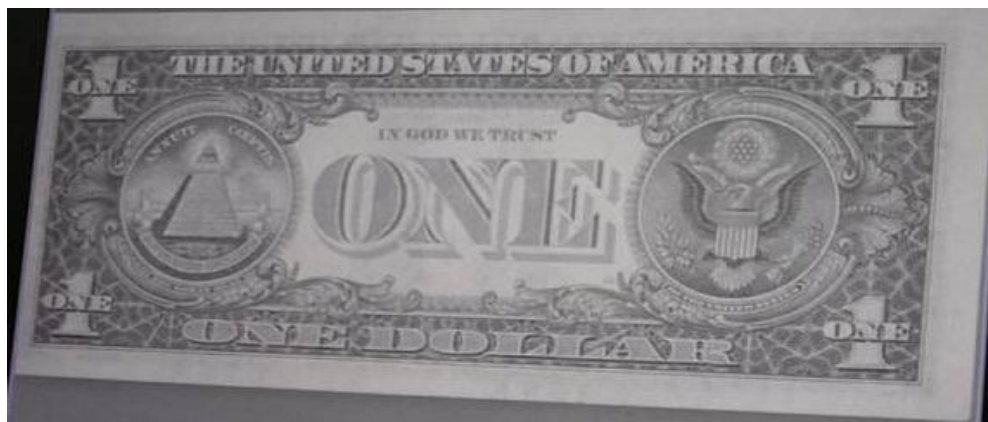
Figure 368: Paper banknote; One dollar (1U$) before treatment after thermal ageing at 140^{\circ}\text{C} through IR radiation (back side).
