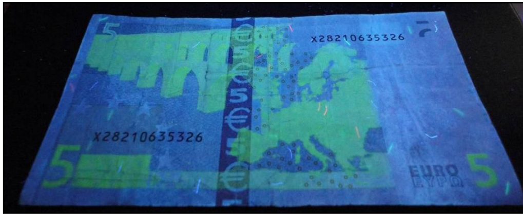
Figure 330: Paper banknote; 5 Euro "€" after coating by 3 rd layer of 1% of carboxymethyl cellulose (CMC) under UV radiation ( \lambda_1 = 256 \text{ nm} ) at 25 0 C through UV radiation (back side)
