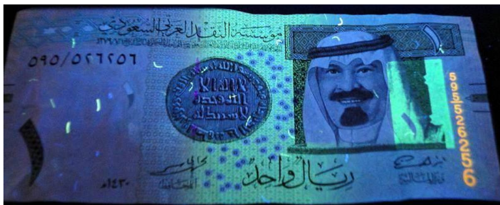
Figure 291: Paper banknote; One riyal (1 SAR) before treatment under UV radiation ( \lambda_2 = 336 \text{ nm} ) at 25^\circ\text{C} through UV radiation (front side).
