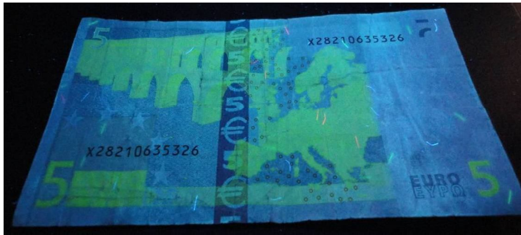
Figure 332: Paper banknote; 5 Euro "€" after coating by 3 rd layer of 1% of carboxymethyl cellulose (CMC) under UV radiation ( \lambda_2 = 336 \text{ nm} ) at 25 o C through UV radiation (back side).
