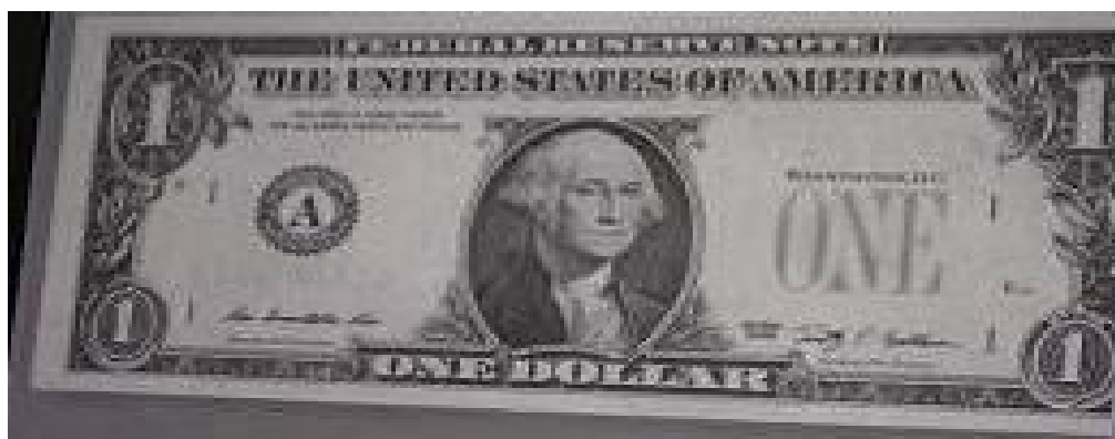
Figure 375: Paper banknote; One dollar (1U$) after coating by 3 rd layer of 1% of carboxymethyl cellulose (CMC) after thermal ageing at 140 °C through IR radiation (front side).
