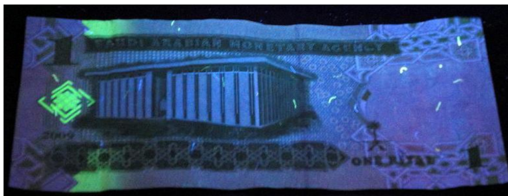
Figure (298): Paper banknote; One riyal (1 SAR) after coating by 3 rd layer of 1% of carboxymethyl cellulose (CMC) under UV radiation ( \lambda_1 = 256 \text{ nm} ) at 25 °C through UV radiation (back side).
