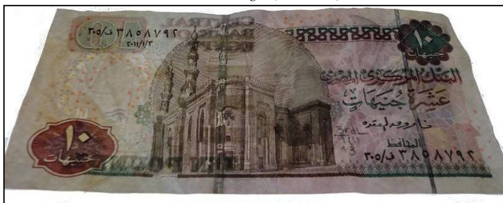
Figure 163: Paper banknote; Egyptian ten pounds (10 EGP) after coating by 3 rd layer of 1% of carboxymethyl cellulose (CMC) under UV radiation ( \lambda_2 = 336 nm) through transmitted light (front side).
