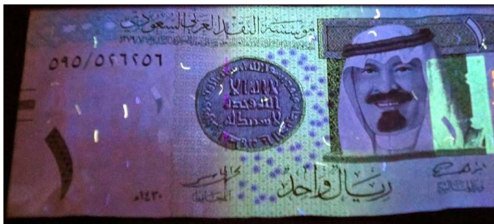
Figure 289: Paper banknote; One riyal (1 SAR) before treatment under UV radiation ( \lambda_1 = 256 \text{ nm} ) at 25 °C through UV radiation (front side)
