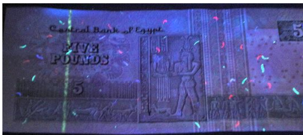
Figure 252: Paper banknote; Egyptian five pounds (5 EGP) after coating by 3 rd layer of 1% of carboxymethyl cellulose (CMC) under UV radiation ( \lambda_2 = 336 \text{ nm} ) at 25 0 C through UV radiation (back side).
