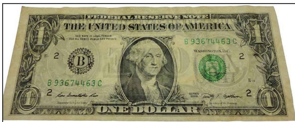
Figure 175: Paper banknote; one dollar (1U$) after coating by 3 rd layer of 0.1% of Carboxymethyl cellulose (CMC) after thermal ageing 140 °C through transmitted light (front side).
