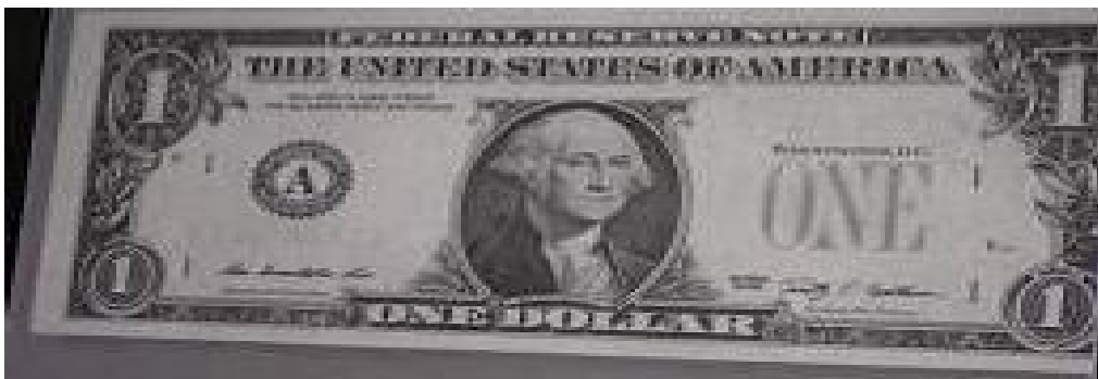
Figure 379) Paper banknote; One dollar (1U$) after coating by 3 rd layer of 1% of carboxymethyl cellulose (CMC) under IR radiation ( \lambda_2 = 336 \text{ nm} ) at 25 o C through IR radiation (front side).
