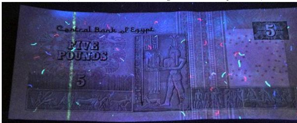
Figure 244: Paper banknote; Egyptian five pounds (5 EGP) before treatment under UV radiation ( \lambda_2 = 336 \text{ nm} ) at 25^\circ\text{C} through UV radiation (back side).
