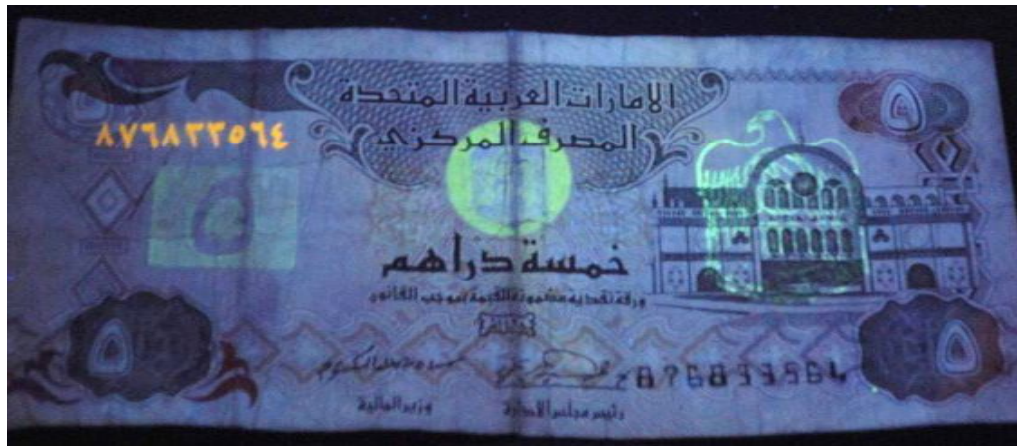
Figure 303: Paper banknote; 5 Dirham "AED" before treatment after thermal ageing at 140^{\circ}\text{C} through UV radiation (front side).
