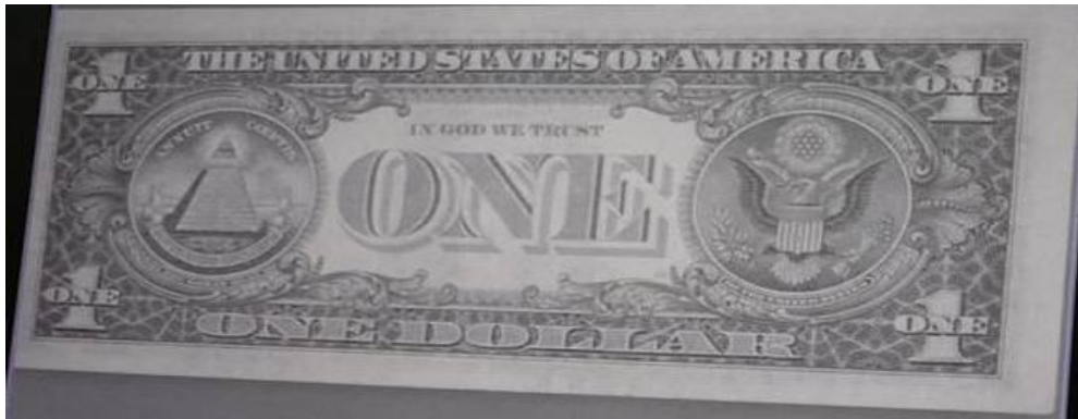
Figure 378: Paper banknote; One dollar (1U$) after coating by 3 rd layer of 1% of carboxymethyl cellulose (CMC) under IR radiation ( \lambda_1 = 256 \text{ nm} ) at 25 o C through IR radiation (back side).
