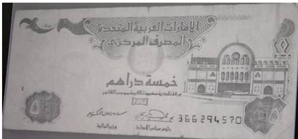
Figure 407: Paper banknote; 5 Dirham "AED" after coating by 3 rd layer of 1% of carboxymethyl cellulose (CMC) after thermal ageing at 140 °C through IR radiation (front side).
