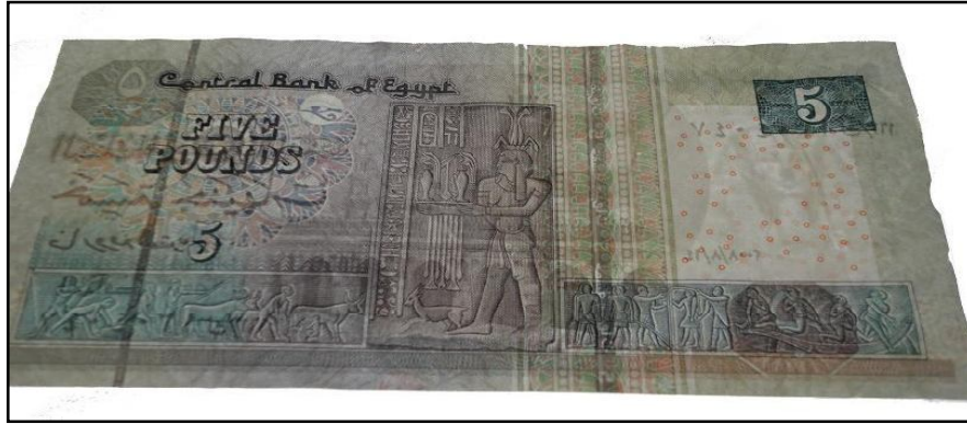
Figure 121: Paper banknote; Egyptian five pounds (5 EGP) before treatment after thermal ageing at 140^{\circ}\text{C} through transmitted light (back side).
