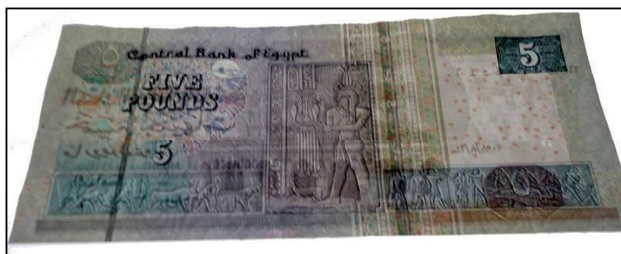
Figure 128: Paper banknote; Egyptian five pounds (5 EGP) after coating by 3 rd layer of 0.1% of carboxymethyl cellulose (CMC) after thermal ageing at 140 °C through transmitted light (back side).
