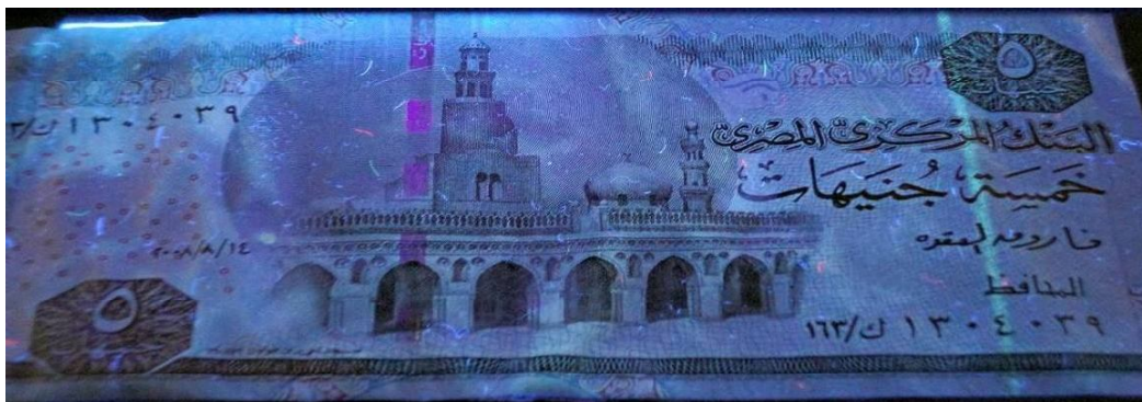
Figure 239: Paper banknote; Egyptian five pounds (5 EGP) before treatment after thermal ageing at 140 °C through UV radiation (front side).
