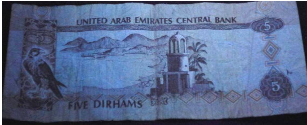
Figure 308: Paper banknote; 5 Dirham "AED" before treatment under UV radiation ( \lambda_2 = 336 \text{ nm} ) at 25^\circ\text{C} through UV radiation (back side).
