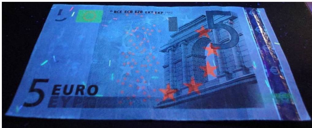
Figure 331: Paper banknote; 5 Euro "€" after coating by 3 rd layer of 1% of carboxymethyl cellulose (CMC) under UV radiation ( \lambda_2 = 336 \text{ nm} ) at 25 0 C through UV radiation (front side).
