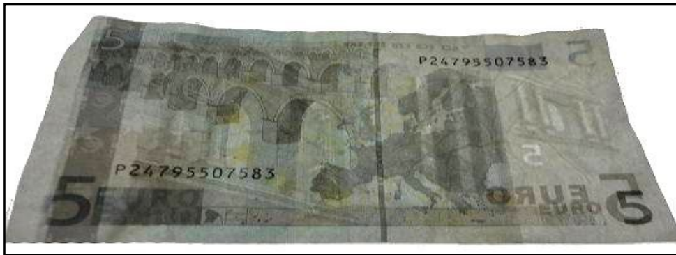
Figure 236: Paper banknote; five Euro (5 €) after coating by 3 rd layer of 1% carboxymethyl cellulose (CMC) under UV radiation ( \lambda_2 = 336 \text{ nm} ) at 25 0 C through transmitted light (back side).
