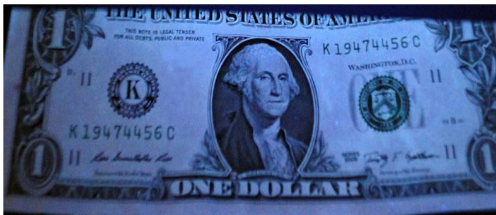
Figure 271: Paper banknote; One dollar (1US$) before treatment after thermal ageing at 140^{\circ}\text{C} through UV radiation (front side).
