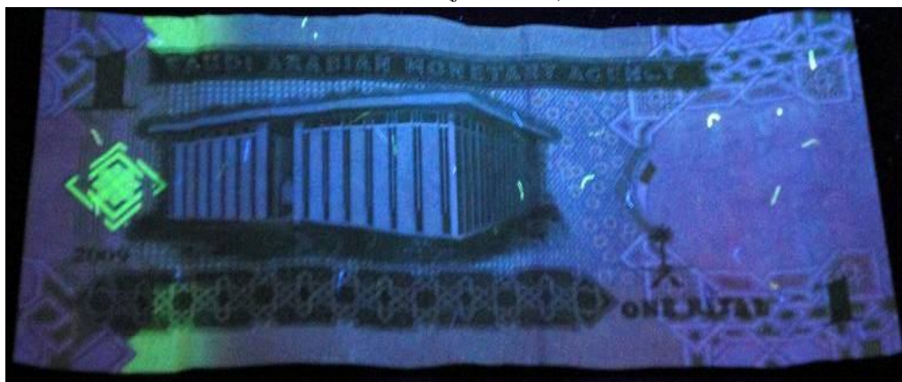
Figure 300: Paper banknote; One riyal (1 SAR) after coating by 3 rd layer of 1% of carboxymethyl cellulose (CMC) under UV radiation ( \lambda_2 = 336 \text{ nm} ) at 25 0 C through UV radiation (front side).
