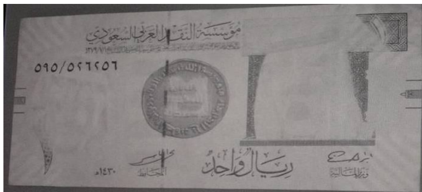
Figure 395: Paper banknote; One riyal (1 SAR) after coating by 3 rd layer of 1% of carboxymethyl cellulose (CMC) under IR radiation ( \lambda_2 = 336 \text{ nm} ) at 25 0 C through IR radiation (front side).
