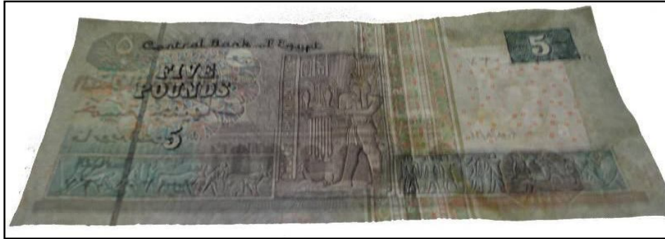
Figure 138: Paper banknote; Egyptian five pounds (5 EGP) after coating by 3 rd layer of 1% of carboxymethyl cellulose (CMC) under UV radiation ( \lambda_1 = 256 nm) through transmitted light (back side).
