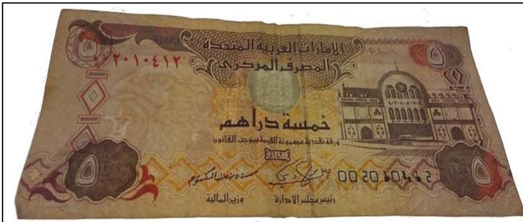
Figure 207: Paper banknote; five Dirhams (5 AED) before treatment after thermal ageing at 140 °C through transmitted light (front side).
