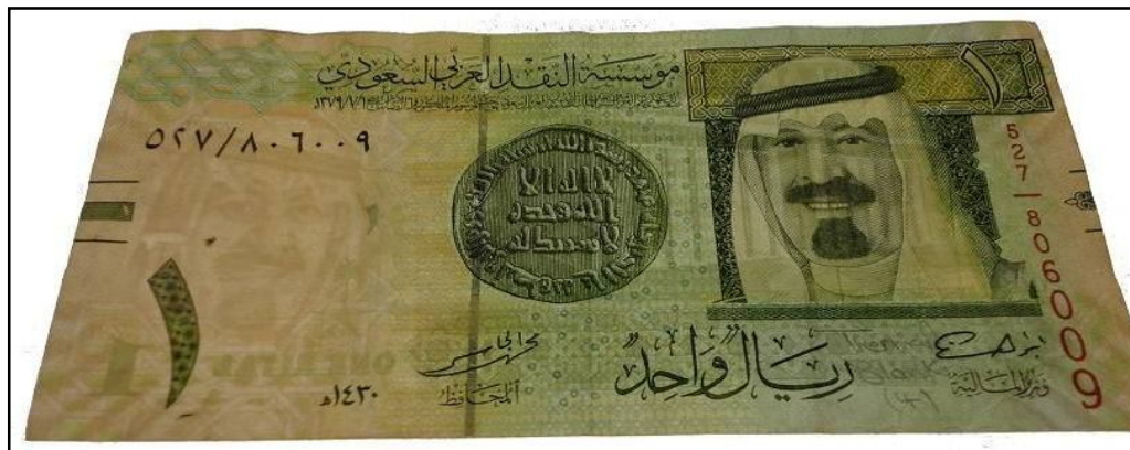
Figure 191: Paper banknote; one riyal (1 SAR) before treatment after thermal ageing at 140^{\circ}\text{C} through transmitted light (front side).
