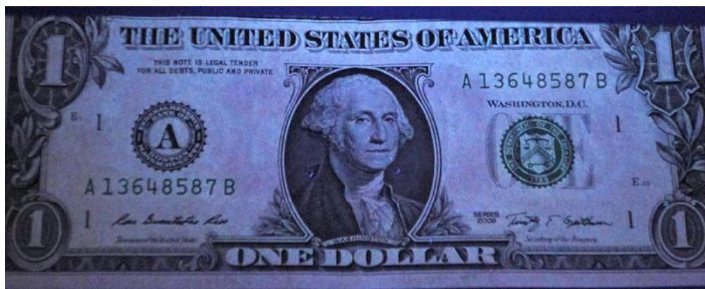
Figure 275: Paper banknote; One dollar (1U$) before treatment under UV radiation ( \lambda_2 = 336 \text{ nm} ) at 25^\circ\text{C} through UV radiation (front side).
