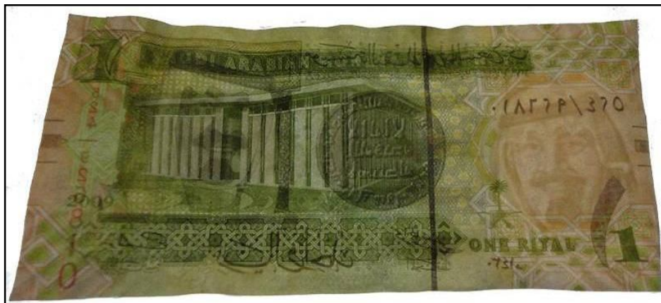
Figure 200: Paper banknote; one riyal (1 SAR) after coating by 3 rd layer of 1% carboxymethyl cellulose (CMC) after thermal ageing at 140 °C through transmitted light (front side).
