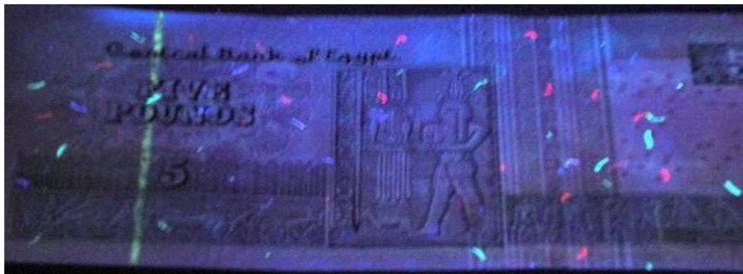
Figure 248: Paper banknote; Egyptian five pounds (5 EGP) after coating by 3 rd layer of 1% of carboxymethyl cellulose (CMC) after thermal ageing at 140 °C through UV radiation (back side).
