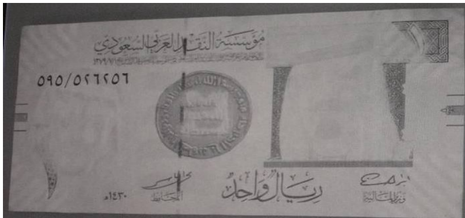
Figure 393: Paper banknote; One riyal (1 SAR) after coating by 3 rd layer of 1% of carboxymethyl cellulose (CMC) under IR radiation ( \lambda_1 = 256 \text{ nm} ) at 25 °C through IR radiation (front side).
