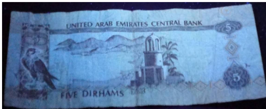
Figure 316: Paper banknote; 5 Dirham "AED" after coating by 3 rd layer of 1% of carboxymethyl cellulose (CMC) under UV radiation ( \lambda_2 = 336 \text{ nm} ) at 25 0 C through UV radiation (back side).
