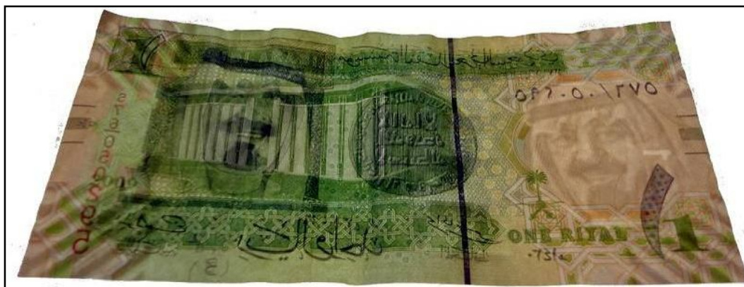
Figure 204: Paper banknote; one Riyal (1 SAR) after coating by 3 rd layer of 1% of carboxymethyl cellulose (CMC) under UV radiation ( \lambda_2 = 336 \text{ nm} ) through transmitted light (back side).
