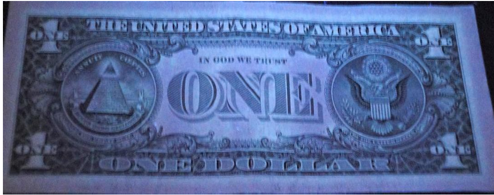
Figure 284: Paper banknote; One dollar (1U$) after coating by 3 rd layer of 1% of carboxymethyl cellulose (CMC) under UV radiation ( \lambda_2 = 336 \text{ nm} ) at 25 o C through UV radiation (back side).
