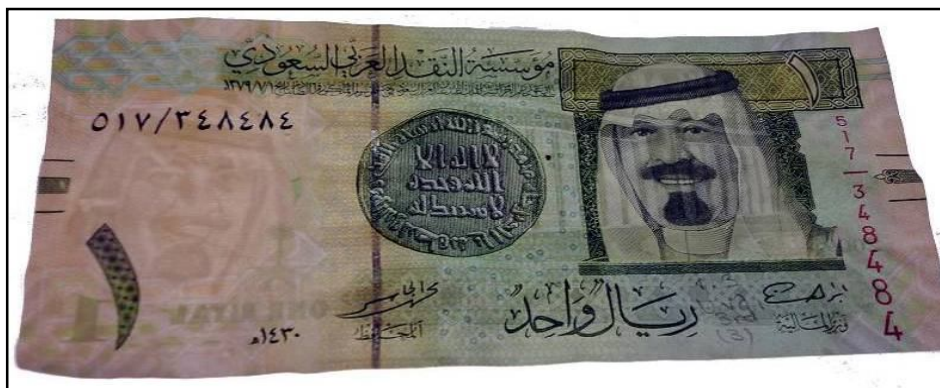
Figure 201: Paper banknote; one riyal (1 SAR) after coating by 3 rd layer of 1% carboxymethyl cellulose (CMC) under UV radiation ( \lambda_1 = 256 nm) through transmitted light (front side).
