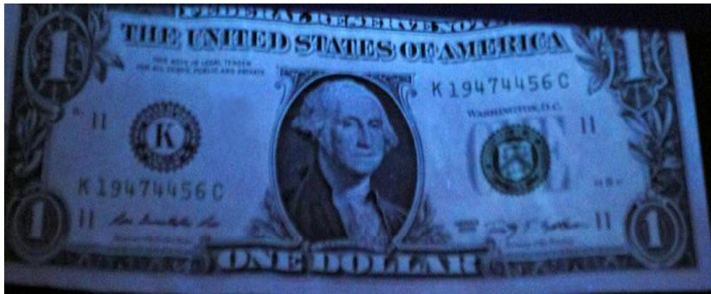
Figure 273: Paper banknote; One dollar (1U$) before treatment under UV radiation ( \lambda_1 = 256 \text{ nm} ) at 25^{\circ}\text{C} through UV radiation (front side).
