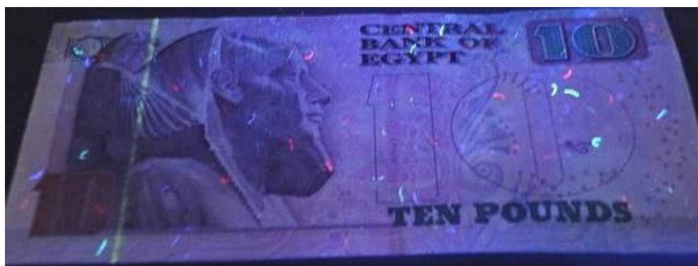
Figure 262: Paper banknote; Egyptian ten pounds (10 EGP) after coating by 3 rd layer of 1% of carboxymethyl cellulose (CMC) through UV radiation (back side).
