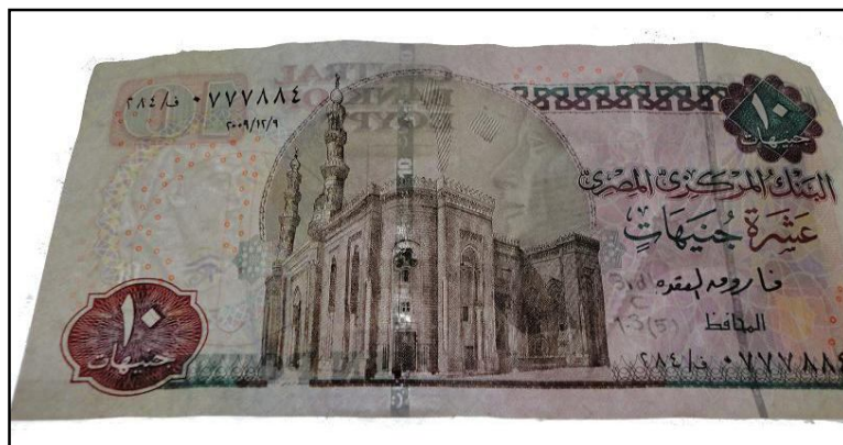
Figure 159: Paper banknote; Egyptian ten pounds (10 EGP) after coating by 3 rd layer of 1% of carboxymethyl cellulose (CMC) after thermal ageing at 140 °C through transmitted light (front side).
