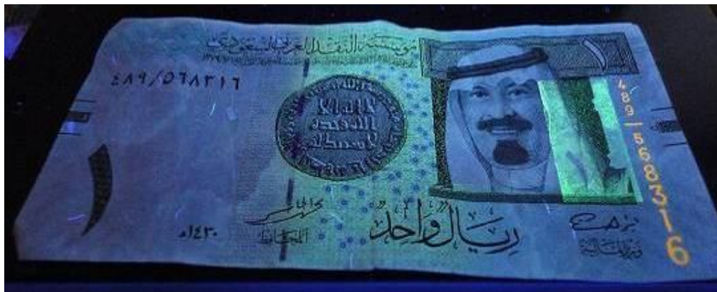
Figure (299): Paper banknote; One riyal (1 SAR) after coating by 3 rd layer of 1% of carboxymethyl cellulose (CMC) under UV radiation ( \lambda_2 = 336 \text{ nm} ) at 25 0 C through UV radiation (front side).
