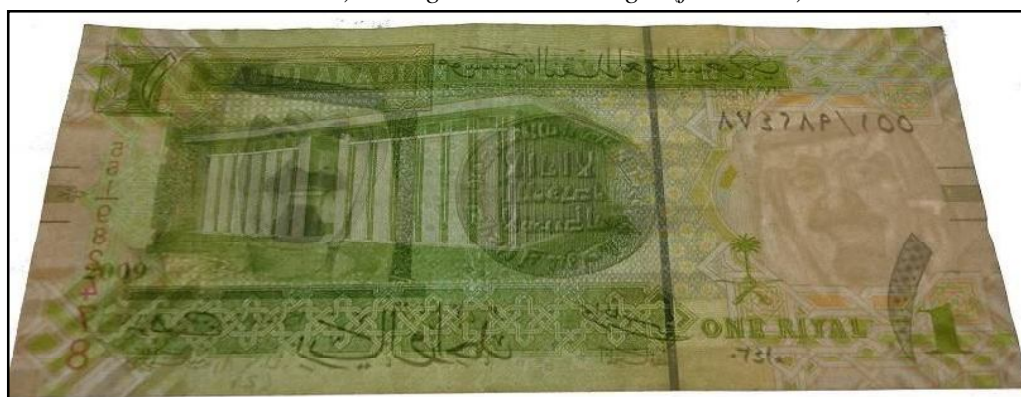
Figure 194: Paper banknote; one riyal (1 SAR) before treatment under UV radiation ( \lambda_1 = 256\text{ nm} ) through transmitted light (back side).
