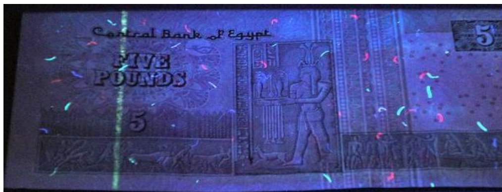
Figure 238: Paper banknote; Egyptian five pounds (5 EGP) before treatment through UV radiation (back side).
