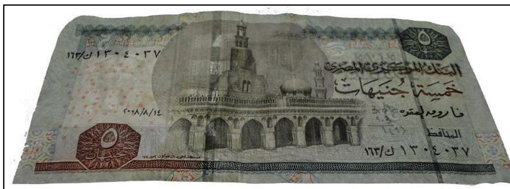
Figure 133: Paper banknote; Egyptian five pounds (5 EGP) after coating by 3 rd layer of 1% of carboxymethyl cellulose (CMC) through transmitted light (front side).
