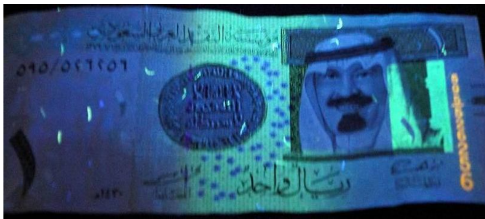
Figure 287: Paper banknote; One riyal (1 SAR) before treatment after thermal ageing at 140 °C through UV radiation (front side).
