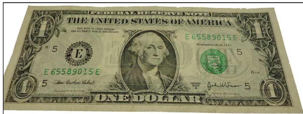
Figure 179: Paper banknote; one dollar (1U$) after coating by 3 rd layer of 0.1% of Carboxymethyl cellulose (CMC) under UV radiation ( \lambda_2 = 336 nm) through transmitted light (front side).
