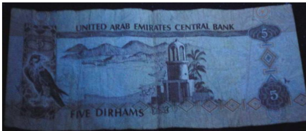
Figure 310: Paper banknote; 5 Dirham "AED" after coating by 3 rd layer of 1% of carboxymethyl cellulose (CMC) through UV radiation (back side).
