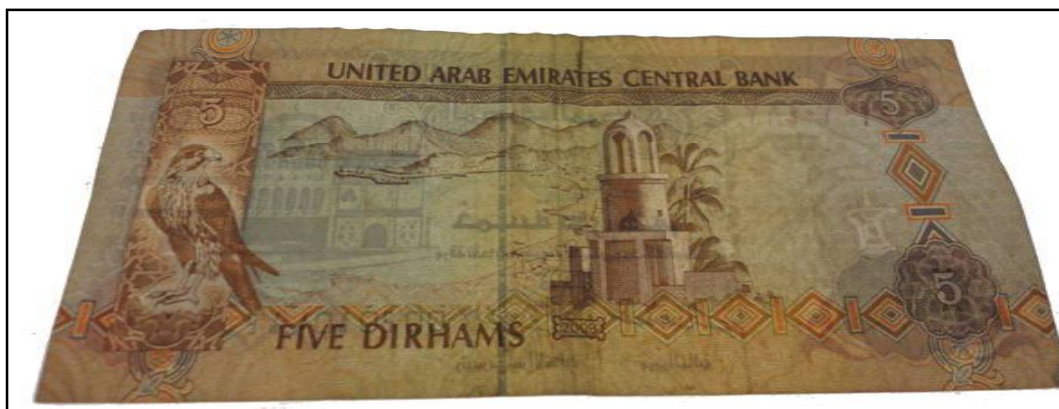
Figure 208: Paper banknote; five Dirhams (5 AED) before treatment after thermal ageing at 140 °C through transmitted light (back side)
