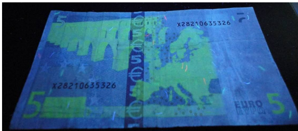
Figure 320: Paper banknote; 5 Euro "€" before treatment after thermal ageing at 140^{\circ}\text{C} through UV radiation (back side)
