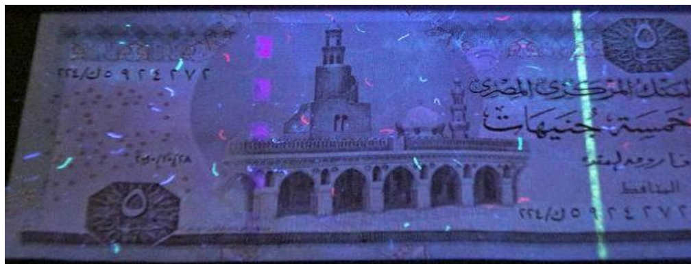
Figure 247: Paper banknote; Egyptian five pounds (5 EGP) after coating by 3 rd layer of 1% of carboxymethyl cellulose (CMC) after thermal ageing at 140 °C through UV radiation (front side).
