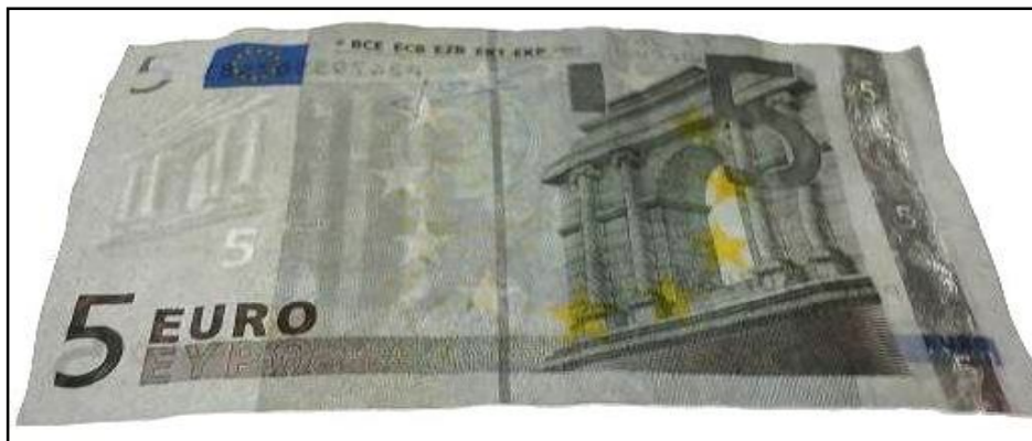
Figure 235: Paper banknote; five Euro (5 €) after coating by 3 rd layer of 1% carboxymethyl cellulose (CMC) under UV radiation ( \lambda_2 = 336 \text{ nm} ) at 25 0 C through transmitted light (front side).
