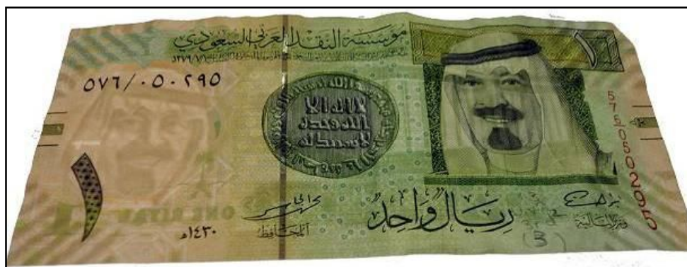
Figure 203: Paper banknote; one Riyal (1 SAR) after coating by 3 rd layer of 1% of carboxymethyl cellulose (CMC) under UV radiation ( \lambda_2 = 336 nm) through transmitted light (front side).
