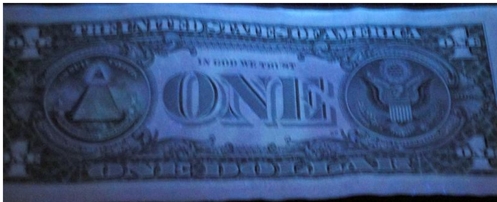
Figure 280: Paper banknote; One dollar (1U$) after coating by 3 rd layer of 1% of carboxymethyl cellulose (CMC) after thermal ageing at 140 °C through UV radiation (back side).
