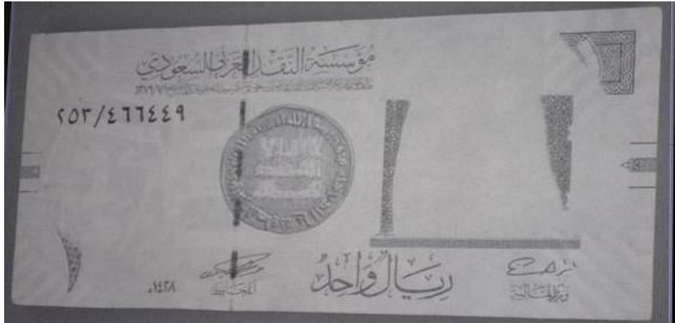
Figure 383: Paper banknote; One riyal (1 SAR) before treatment after thermal ageing at 140 °C through IR radiation (front side).
