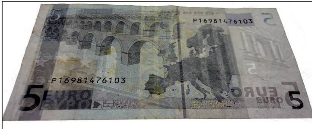
Figure 224: Paper banknote; five Euro (5 €) before treatment after thermal ageing at 140^{\circ}\text{C} through transmitted light (back side).
