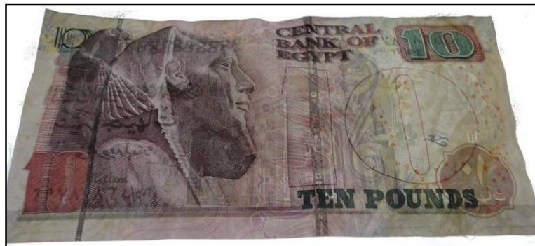
Figure 156: Paper banknote; Egyptian ten pounds (10 EGP) after coating by 3 rd layer of 0.1% of carboxymethyl cellulose (CMC) under UV radiation ( \lambda_2 = 336 \text{ nm} ) at 25 °C through transmitted light (back side).
