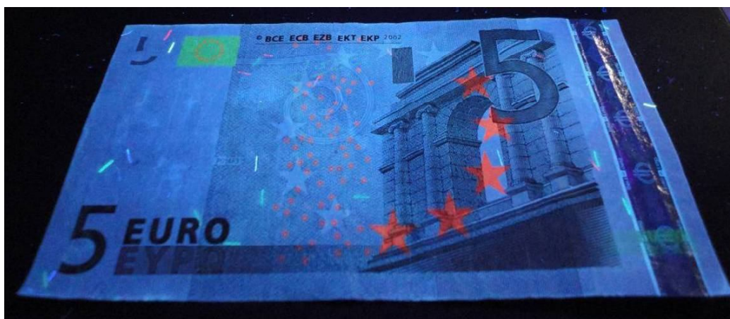
Figure 325: Paper banknote; 5 Euro "€" after coating by 3 rd layer of 1% of carboxymethyl cellulose (CMC) through UV radiation (front side)
