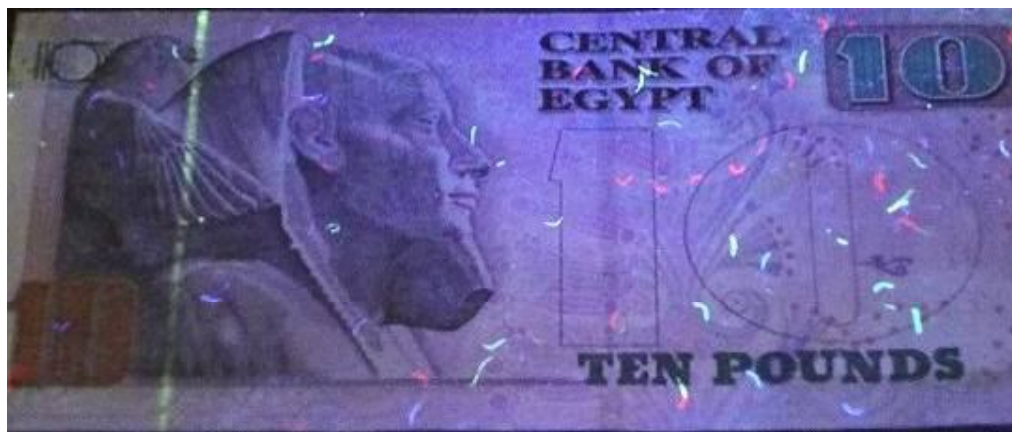
Figure 260: Paper banknote; Egyptian ten pounds (10 EGP) before treatment under UV radiation ( \lambda_2 = 336 \text{ nm} ) at 25^{\circ}\text{C} through UV radiation (back side).
