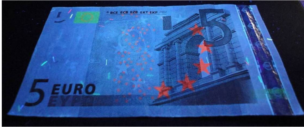
Figure 329: Paper banknote; 5 Euro "€" after coating by 3 rd layer of 1% of carboxymethyl cellulose (CMC) under UV radiation ( \lambda_1 = 256 \text{ nm} ) at 25 0 C through UV radiation (front side)
