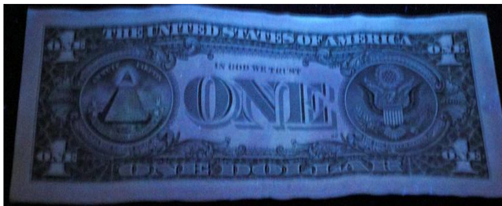
Figure 282: Paper banknote; One dollar (1U$) after coating by 3 rd layer of 1% of carboxymethyl cellulose (CMC) under UV radiation ( \lambda_1 = 256 \text{ nm} ) at 25 o C through UV radiation (back side).
