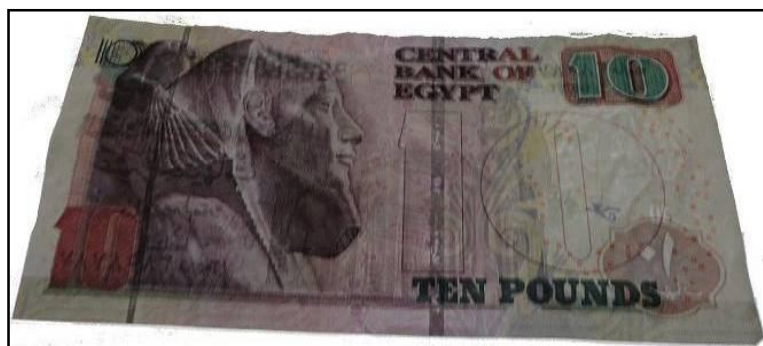
Figure 158: Paper banknote; Egyptian ten pounds (10 EGP) after coating by 3 rd layer of 1% of carboxymethyl cellulose (CMC) through transmitted light (back side).
