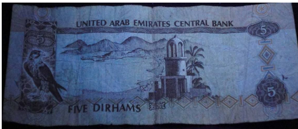
Figure 312: Paper banknote; 5 Dirham "AED" after coating by 3 rd layer of 1% of carboxymethyl cellulose (CMC) after thermal ageing at 140 °C through UV radiation (back side).
