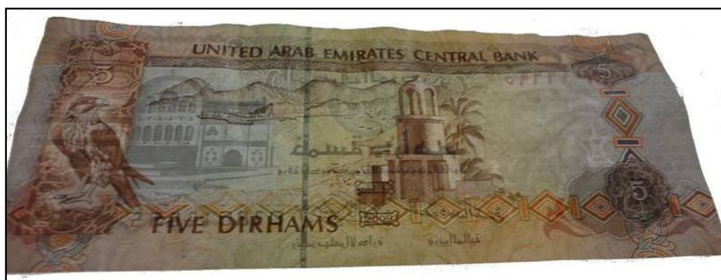
Figure 214: Paper banknote; five Dirhams (5 AED) after coating by 3 rd layer of 1% of carboxymethyl cellulose (CMC) through transmitted light (back side).
