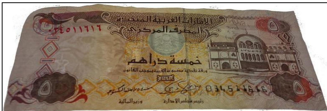
Figure 217: Paper banknote; five Dirhams (5 AED) after coating by 3 rd layer of 1% carboxymethyl cellulose (CMC) of 1% under UV radiation ( \lambda_1 = 256 nm) through transmitted light (front side)
