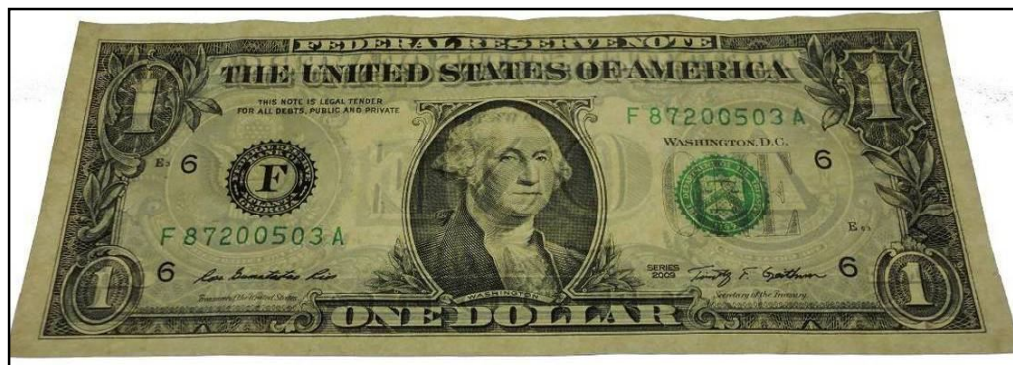
Figure 177: Paper banknote; one dollar (1U$) after coating by 3 rd layer of 0.1% of Carboxymethyl cellulose (CMC) under UV radiation ( \lambda_1 = 256 nm) through transmitted light (front side).
