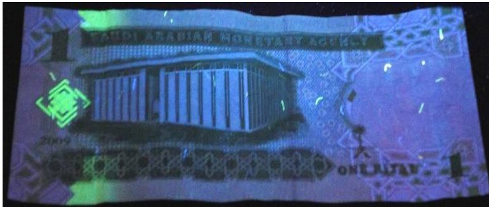
Figure 294: Paper banknote; One riyal (1 SAR) after coating by 3 rd layer of 1% of carboxymethyl cellulose (CMC) through UV radiation (back side).
