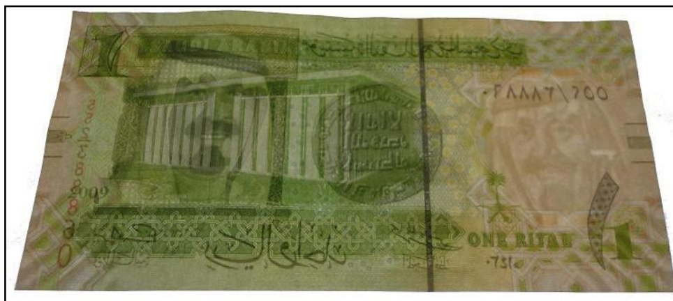
Figure 192: Paper banknote; one riyal (1 SAR) before treatment after thermal ageing at 140^{\circ}\text{C} through transmitted light (back side).
