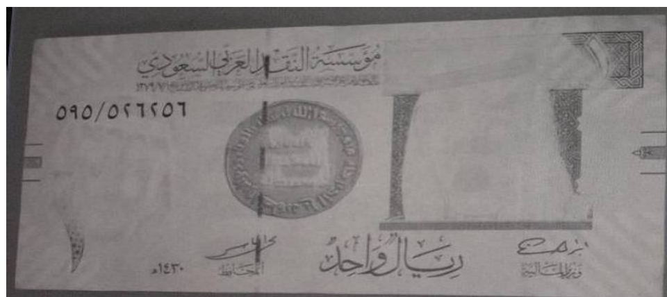
Figure 391: Paper banknote; One riyal (1 SAR) after coating by 3 rd layer of 1% of carboxymethyl cellulose (CMC) after thermal ageing at 140 °C through IR radiation (front side).
