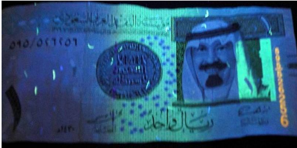
Figure 293: Paper banknote; One riyal (1 SAR) after coating by 3 rd layer of 1% of carboxymethyl cellulose (CMC) through UV radiation (front side)
