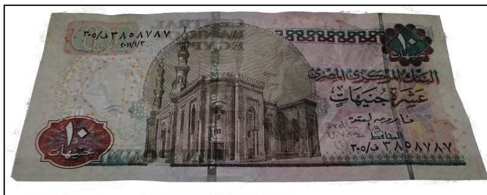
Figure 161: Paper banknote; Egyptian ten pounds (10 EGP) after coating by 3 rd layer of 1% of carboxymethyl cellulose (CMC) under UV radiation ( \lambda_1 = 256 nm) through transmitted light (front side).
