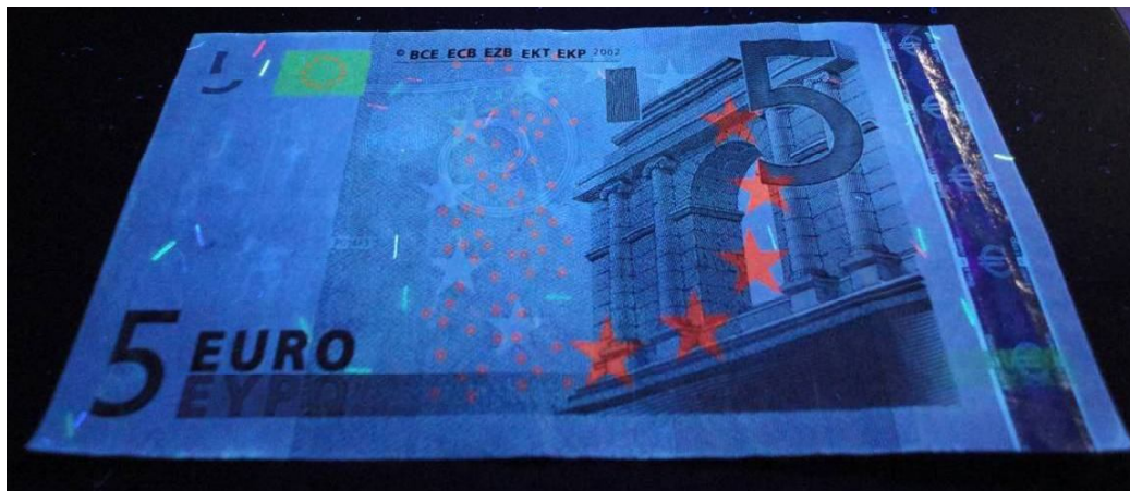
Figure 319: Paper banknote; 5 Euro "€" before treatment after thermal ageing at 140 °C through UV radiation (front side).
