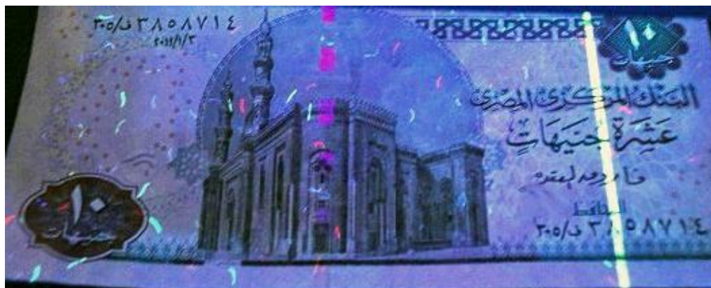
Figure 267: Paper banknote; Egyptian ten pounds (10 EGP) after coating by 3 rd layer of 1% of carboxymethyl cellulose (CMC) under UV radiation ( \lambda_2 = 336 \text{ nm} ) at 25 o C through UV radiation (front side).
