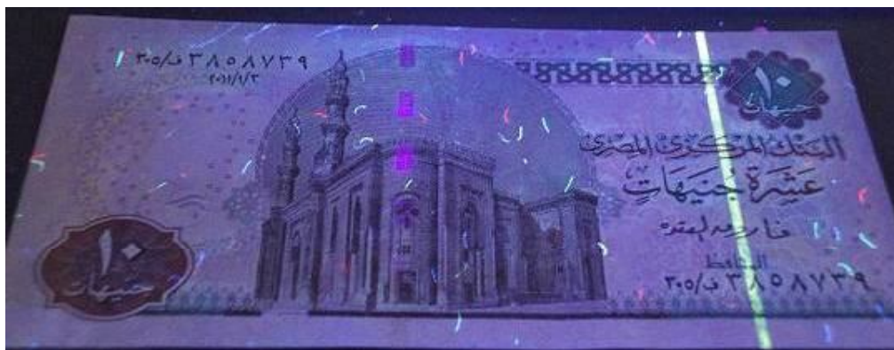
Figure 263: Paper banknote; Egyptian ten pounds (10 EGP) after coating by 3 rd layer of 1% of carboxymethyl cellulose (CMC) after thermal ageing at 140 °C through UV radiation (front side)
