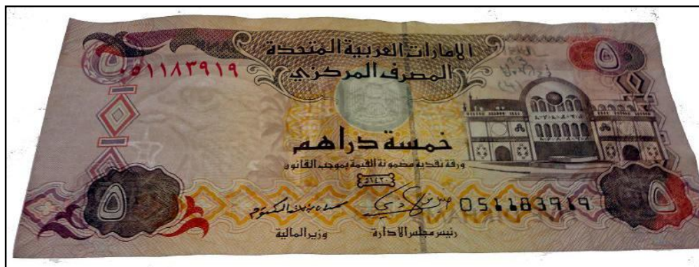
Figure 213: Paper banknote; five Dirhams (5 AED) after coating by 3 rd layer of 1% of carboxymethyl cellulose (CMC) through transmitted light (front side).
