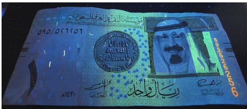
Figure 295: Paper banknote; One riyal (1 SAR) after coating by 3 rd layer of 1% of carboxymethyl cellulose (CMC) after thermal ageing at 140 °C through UV radiation (front side).
