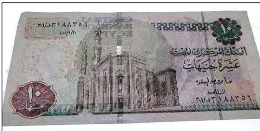
Figure 147: Paper banknote; Egyptian ten pounds (10 EGP) before treatment under UV radiation ( \lambda_2 = 336 \text{ nm} ) at 25^\circ\text{C} through transmitted light (front side)
