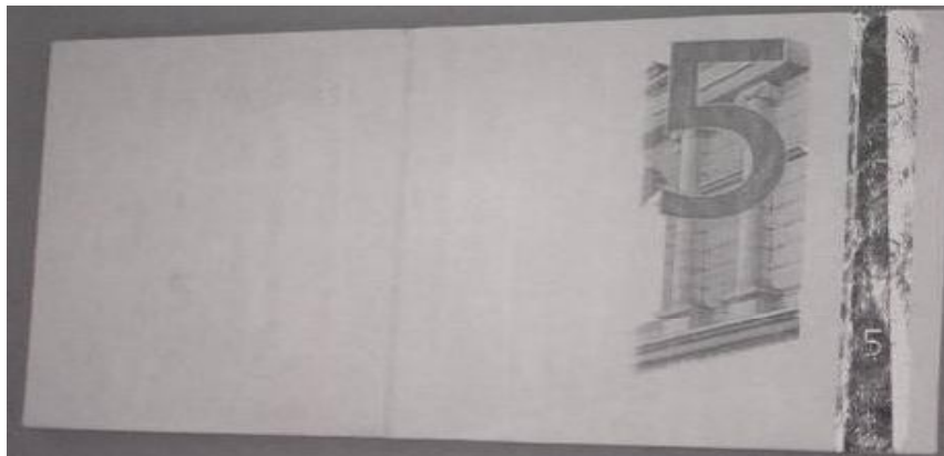
Figure 427: Paper banknote; 5 Euro "€" after coating by 3 rd layer of 1% of carboxymethyl cellulose (CMC) under IR radiation ( \lambda_2 = 336 \text{ nm} ) at 25 o C through IR radiation (front side).
