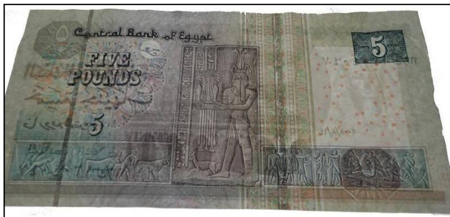
Figure 140: Paper banknote; Egyptian five pounds (5 EGP) after coating by 3 rd layer of 1% of carboxymethyl cellulose (CMC) under UV radiation ( \lambda_2 = 336 nm) through transmitted light (back side).
