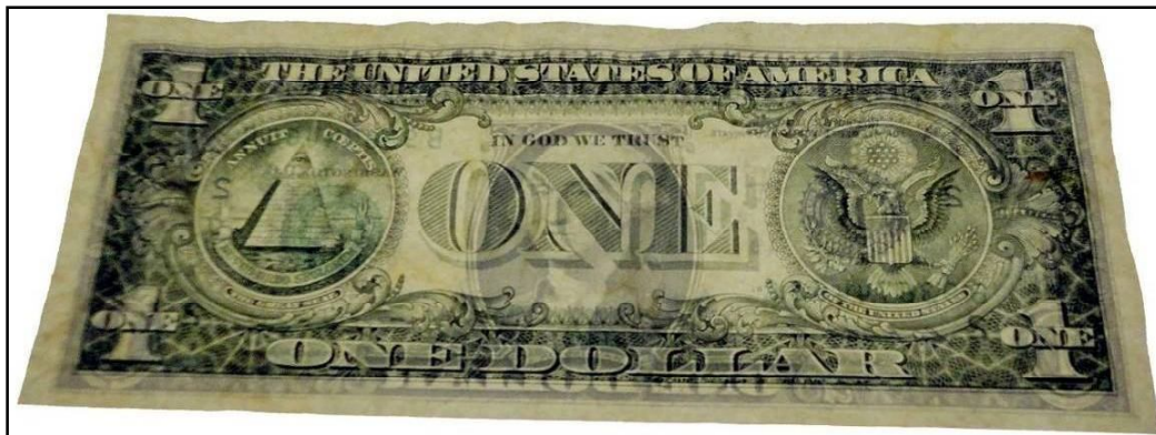
Figure 184: Paper banknote; one dollar (1U$) after coating by 3 rd layer of 1% of Carboxymethyl cellulose (CMC) after thermal ageing 140 °C through transmitted light (back side).
