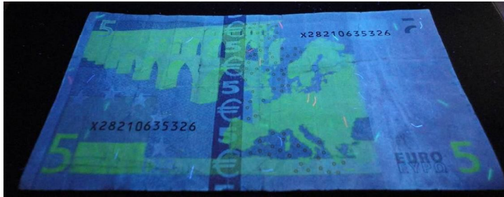
Figure 326: Paper banknote; 5 Euro "€" after coating by 3 rd layer of 1% of carboxymethyl cellulose (CMC) through UV radiation (back side)
