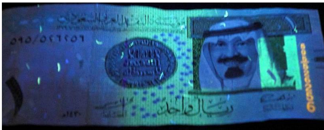
Figure 297: Paper banknote; One riyal (1 SAR) after coating by 3 rd layer of 1% of carboxymethyl cellulose (CMC) under UV radiation ( \lambda_1 = 256 \text{ nm} ) at 25 °C through UV radiation (front side).
