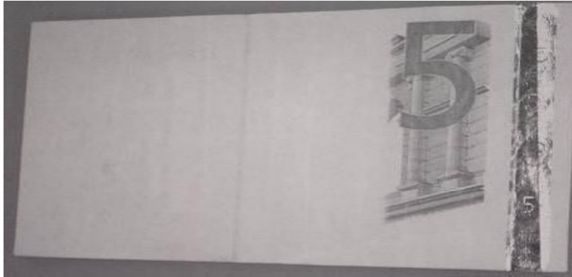
Figure 425: Paper banknote; 5 Euro "€" after coating by 3 rd layer of 1% of carboxymethyl cellulose (CMC) under IR radiation ( \lambda_1 = 256 \text{ nm} ) at 25 o C through IR radiation (front side).
