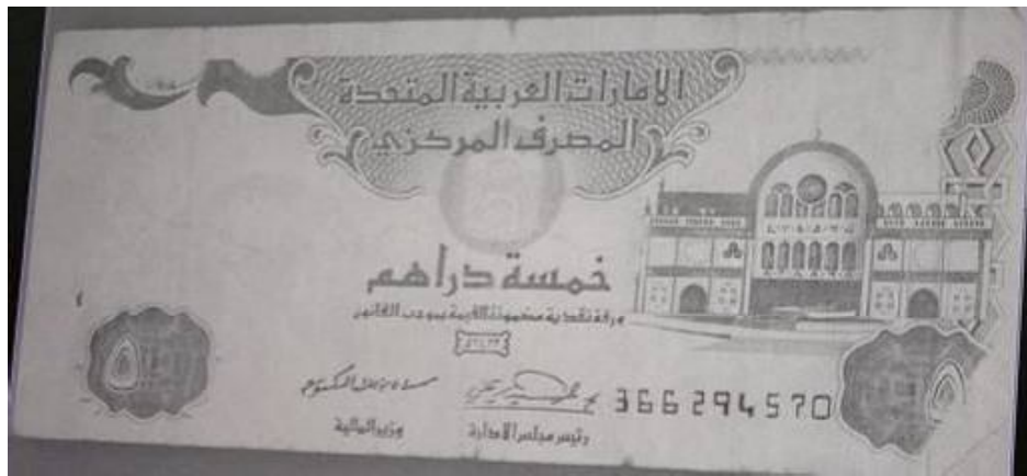
Figure 405: Paper banknote; 5 Dirham "AED" after coating by 3 rd layer of 1% of carboxymethyl cellulose (CMC) through IR radiation (front side).
