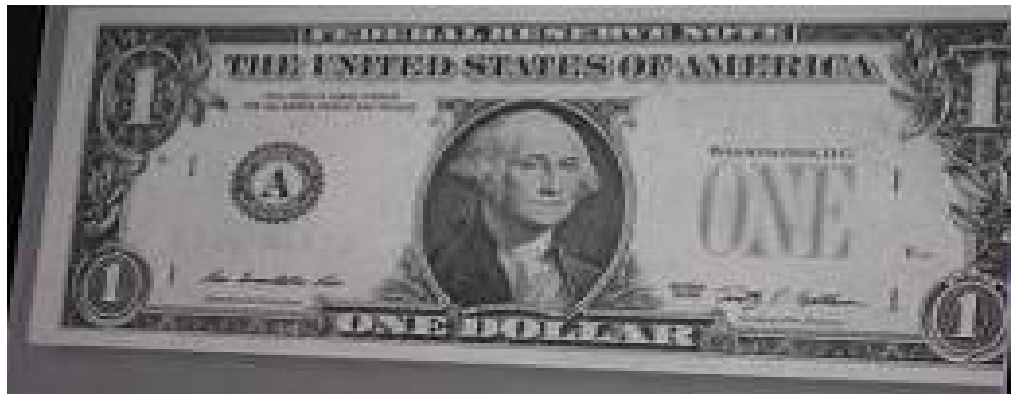
Figure 373: Paper banknote; One dollar (1U$) after coating by 3 rd layer of 1% of carboxymethyl cellulose (CMC) through IR radiation (front side).
