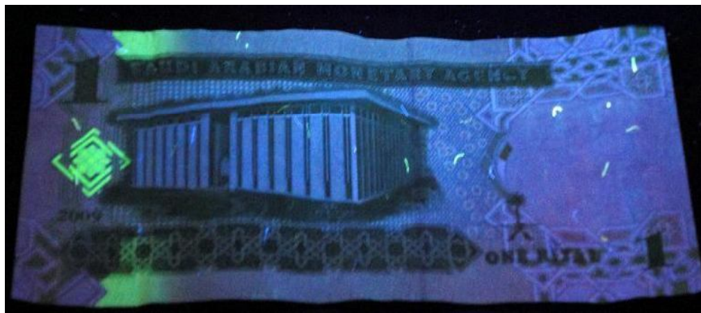
Figure 288: Paper banknote; One riyal (1 SAR) before treatment after thermal ageing at 140 °C through UV radiation (back side).
