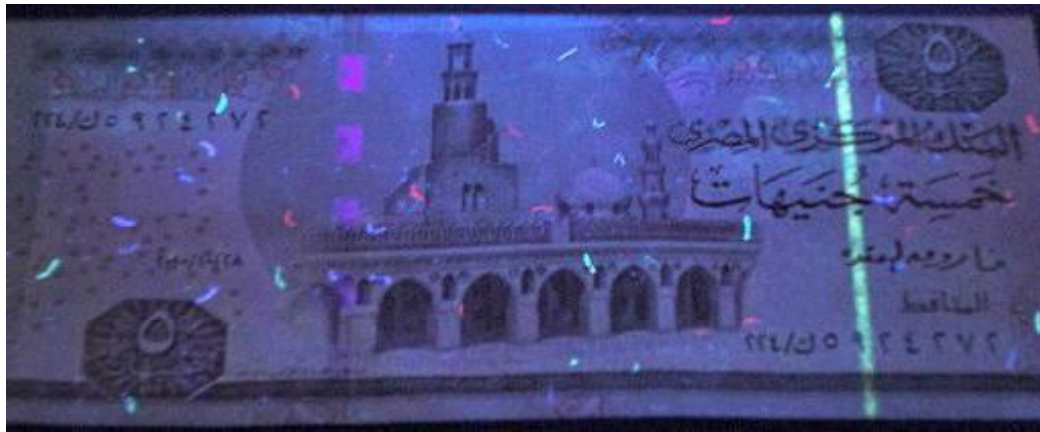
Figure 243: Paper banknote; Egyptian five pounds (5 EGP) before treatment under UV radiation ( \lambda_2 = 336 \text{ nm} ) at 25^\circ\text{C} through UV radiation (front side).
