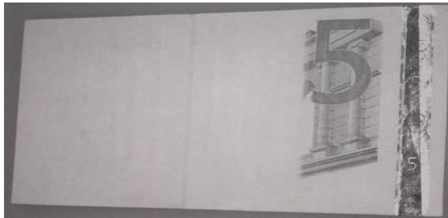
Figure 415: Paper banknote; 5 Euro "€" before treatment after thermal ageing at 140 °C through IR radiation (front side).
