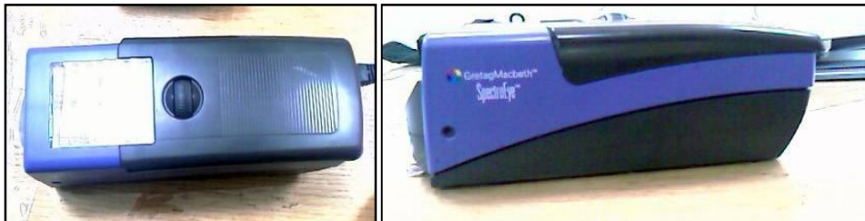
Figure 10: CIE L^*a^*b^* (Commission International d'Eclairage) (Colour Meter, Gretag Macbeth™ SpectroEye™)
