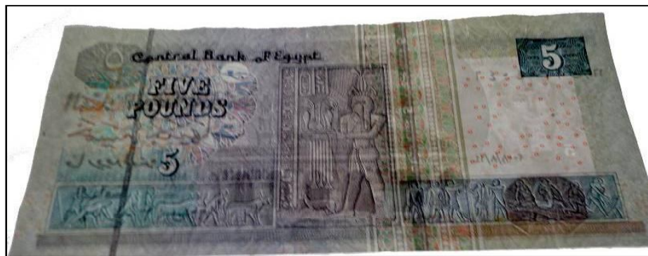
Figure 130: Paper banknote; Egyptian five pounds (5 EGP) after coating by 3 rd layer of 0.1% of carboxymethyl cellulose (CMC) under UV radiation ( \lambda_1 = 256 \text{ nm} ) at 25 °C through transmitted light (back side).
