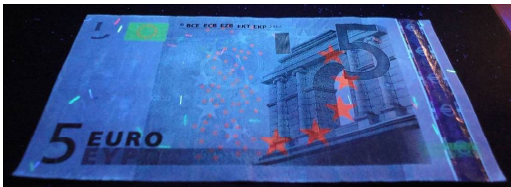
Figure (327): Paper banknote; 5 Euro "€" after coating by 3 rd layer of 1% of carboxymethyl cellulose (CMC) after thermal ageing at 140 0 C through UV radiation (front side)
