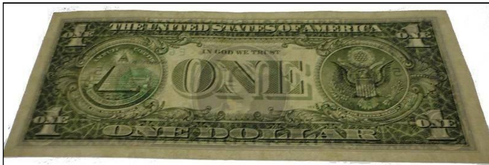
Figure 186: Paper banknote; one dollar (1U$) after coating by 3 rd layer of 1 % of Carboxymethyl cellulose (CMC) under UV radiation ( \lambda_1 = 256 nm) through transmitted light (back side).
