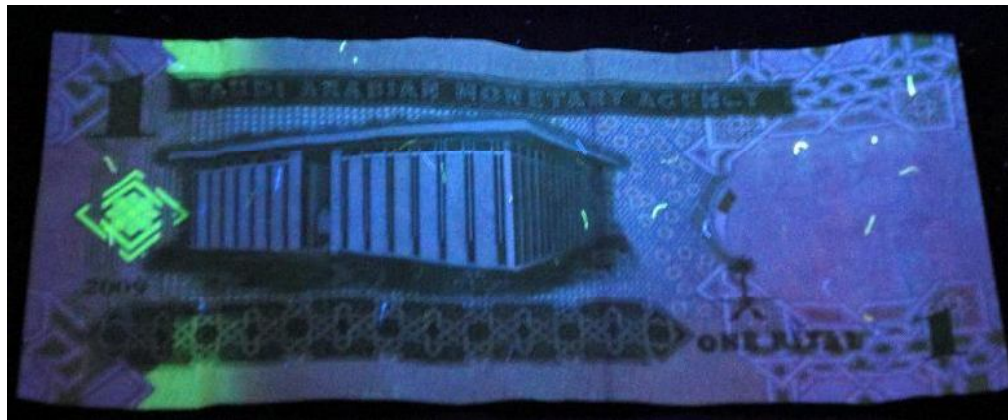
Figure 296: Paper banknote; One riyal (1 SAR) after coating by 3 rd layer of 1% of carboxymethyl cellulose (CMC) after thermal ageing at 140 °C through UV radiation (back side).
