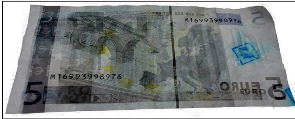
Figure 230: Paper banknote; five Euro (5 €) after coating by 3 rd layer of 1% carboxymethyl cellulose (CMC) through transmitted light (back side)
