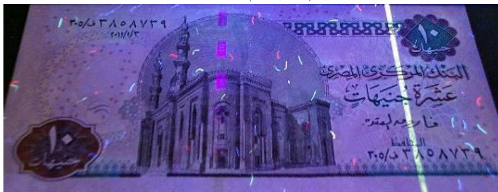
Figure 265: Paper banknote; Egyptian ten pounds (10 EGP) after coating by 3 rd layer of 1% of carboxymethyl cellulose (CMC) under UV radiation ( \lambda_1 = 256 \text{ nm} ) at 25 °C through UV radiation (front side).
