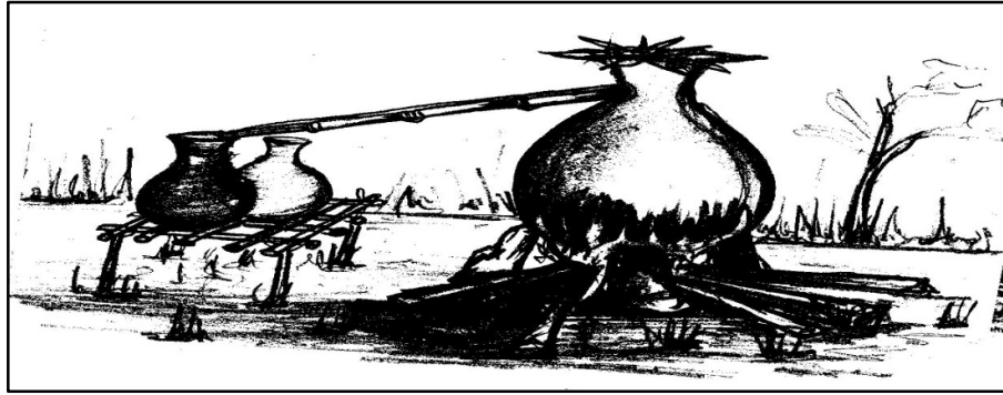
Figure 1: Traditional Pot-Still Distillation Apparatus
