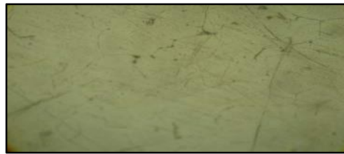
Figure 1: Optical Microscope image of matrix material Al7075 with 100X magnification.
