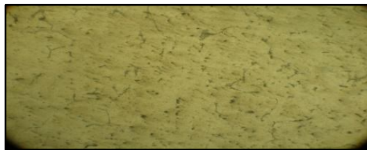
Figure 2: Optical Microscope image of 2.5% SiC and Ni particulate reinforced Al7075
