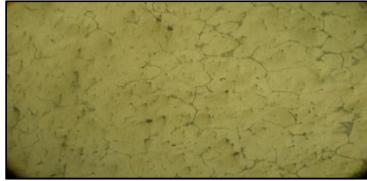
Figure 5: Optical Microscope image of 10% SiC and Ni particulate reinforced Al7075
