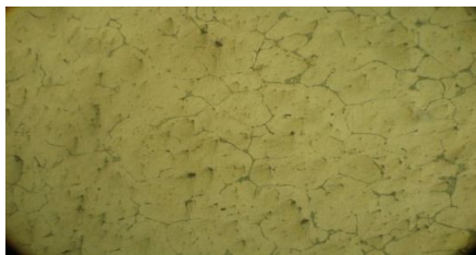
Plate 9: Optical Microscope image of 10% SiC and Ti particulate reinforced Al (6061) composite at 100X magnification.
