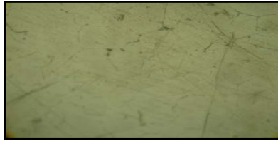
Plate 5: Optical Microscope image of unreinforced Al (6061) alloy at 100X magnification
