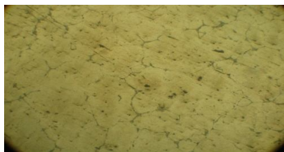
Plate 8: Optical Microscope image of 7.5% SiC and Ti particulate reinforced Al (6061) composite at 100X magnification.
