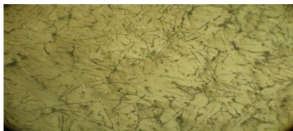
Plate 7: Optical Microscope image of 5% SiC and Ti particulate reinforced Al (6061) composite at 100X magnification.
