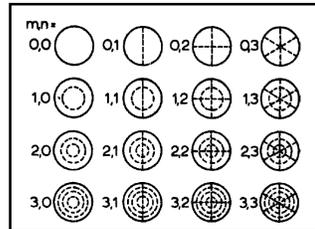
Figure 4: Wavenumbers of circular plate vibration
