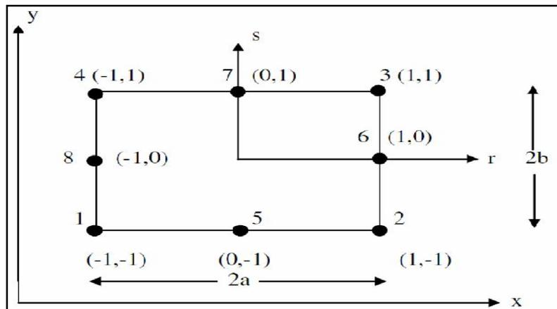
Figure 1: Eight noded rectangular element
