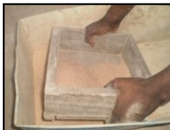
Plate 1: The cyber dust being sieved into fine particles
