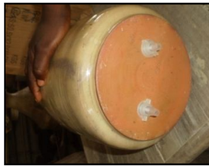
Plate 37: The screw that holds the filter candles to the receptacle
