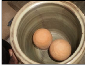
Plate 36: A picture of the two filter candles fixed inside the upper chamber of the receptacle
