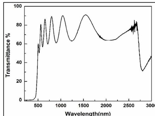
Figure 4: Transmittance spectra of ZnSe thin film
