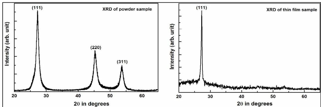
Figure 1: XRD of the synthesized powder sample and the prepared thin film sample
