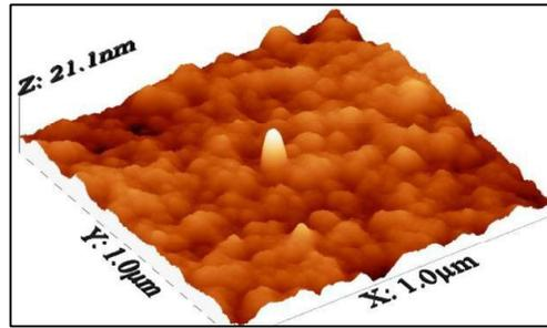
Figure 3: AFM image of ZnSe thin film sample.
