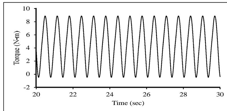
Figure 9: Torque value for unsteady CFD simulation of 3-bladed single stage VAWT
