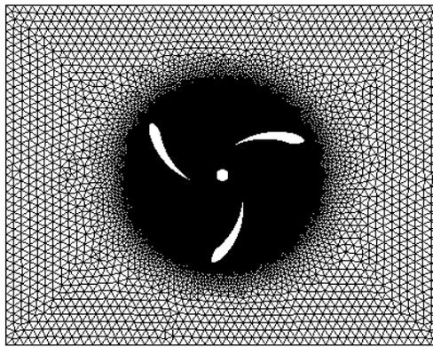
Figure 3: Meshing of the model in Gambit.
