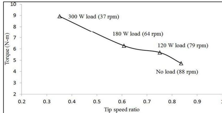
Figure 5: The effect of load on torque data for single stage VAWT at wind speed 5.785 m/s
