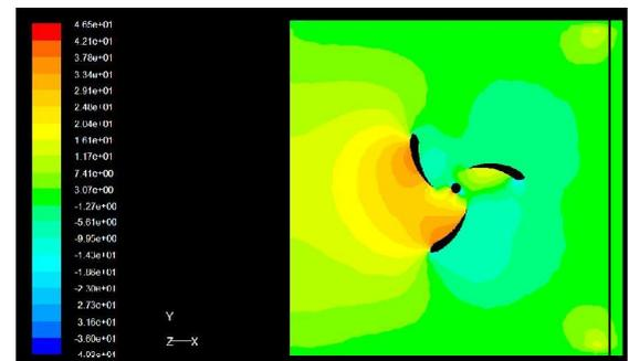
Figure7: Static pressure contours of turbine.
