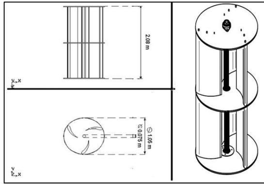
Figure2: Schematic diagram of the 3-bladed VAWT
