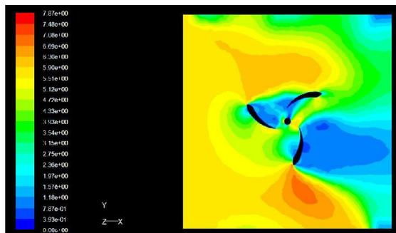
Figure6: Velocity magnitude contours of turbine.
