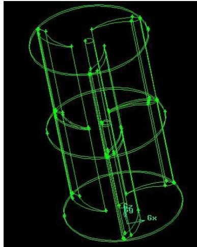
Figure1: 3D turbine model in Gambit
