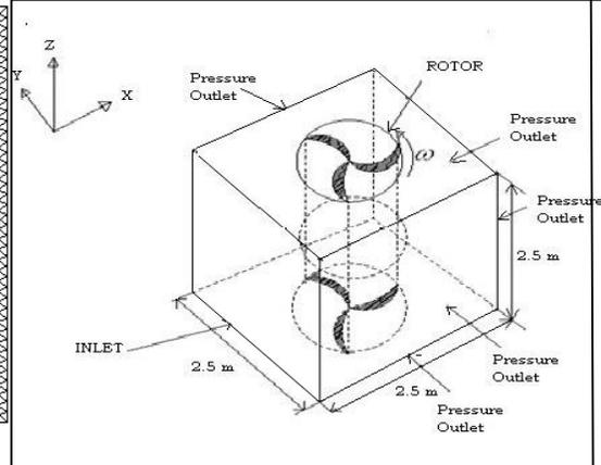
Figure 4: Boundary condition of the 3D model.
