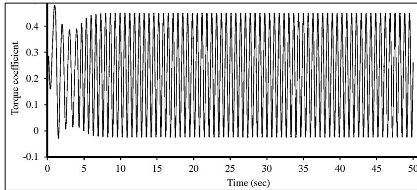
Figure 8: Torque coefficients for unsteady CFD simulation of 3-bladed single stage VAWT
