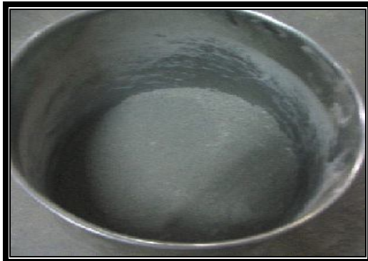
Figure 1: Dry Mixture Of RPC (Without Fibers)
