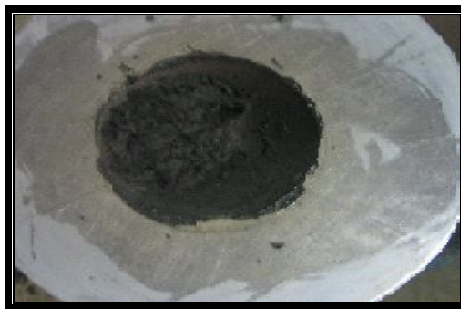
Figure 3: Flow Test Of RPC Mixture
