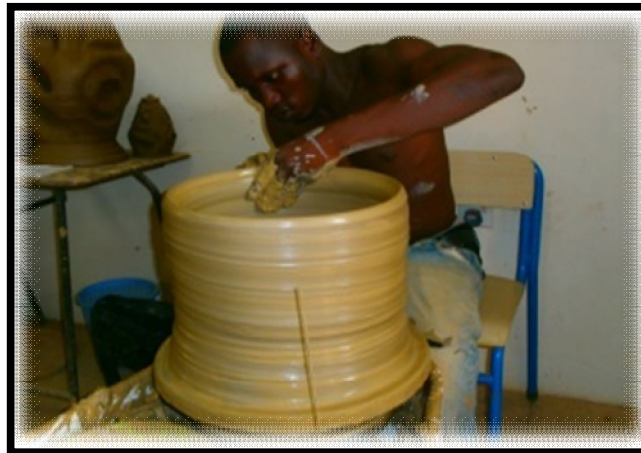
Figure 37: Pulling Of Clay To The Required Height
