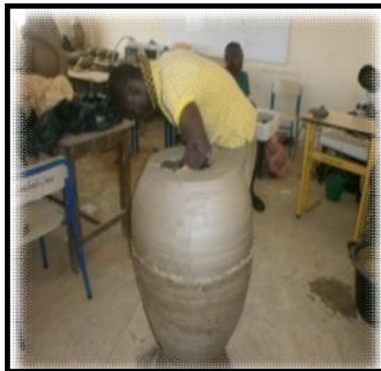
Figure 46: Cleaning Of Excess Slip After Joining With Foam
