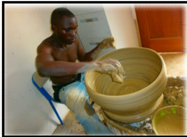
Figure 39: Cleaning Of The Shaped Clay With Foam To Prevent Cracking When Drying
