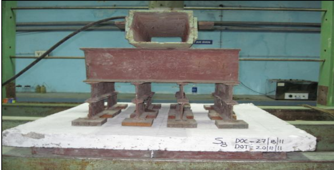
Figure 5: Test Setup for Simply Supported Condition
