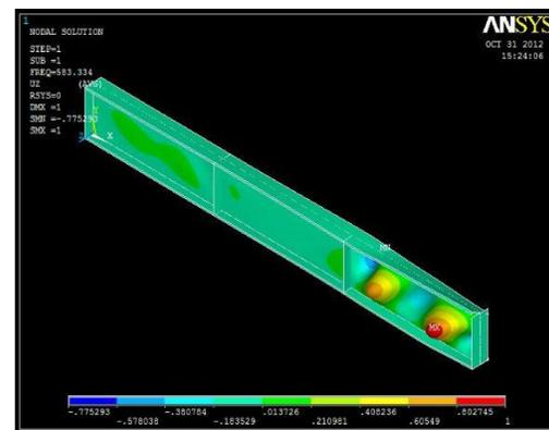
Figure12: Experimental Failure mode of TCWD5, Figure 13:FEA Deformation mode of TCWD5
