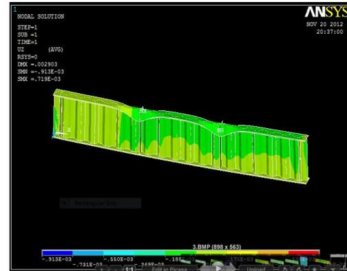
Figure10: Experimental Failure mode of TCWD4, Figure11:FEA Deformation mode of TCWD4
