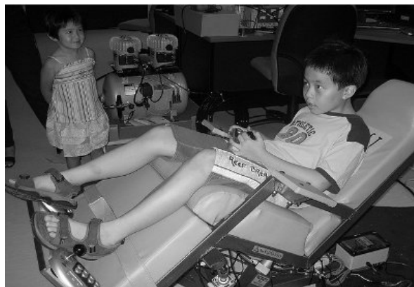
Figure 3 : An Active Chair used in the TRUST project, providing motion feedback and an immersive gateway into a fun rehabilitation experience.
