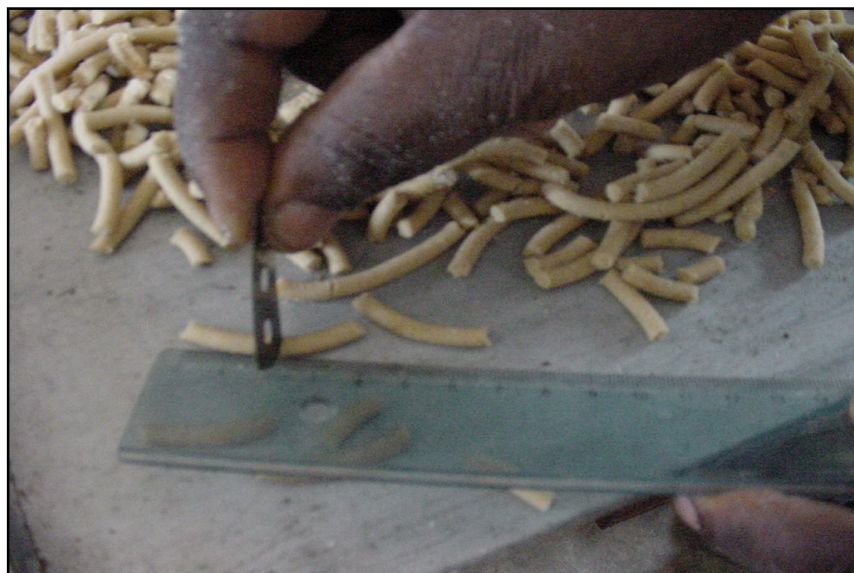
Plate 2: Cutting of strands into equal (2cm) cylindrical or pellet sizes with a rule
