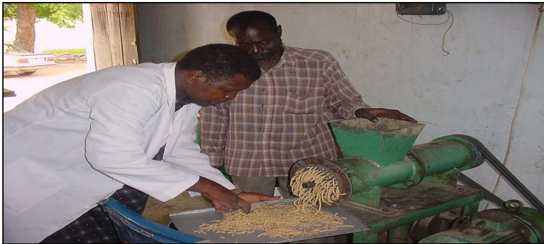
Plate 1: Pelleting of diets dough with PRODA made Pelletizer into oil-filmed galvanised tray.
