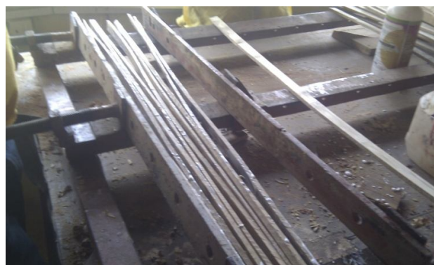
Figure11: clamps for lamination of bamboo with bamboo strips to be laminated
