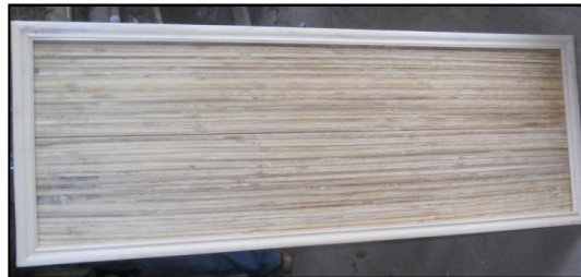
Figure15: First Sample of bambusa bambos floorboard
