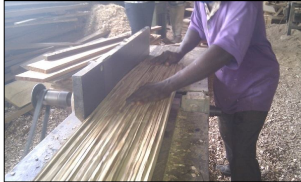
Figure 12: Laminated bamboo strips ready for planing
