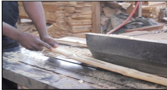
Figure 4: Splitting of bamboo
