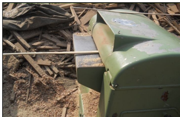
Figure 6: The planing of the bamboo strips
