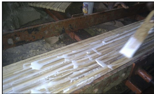
Figure 13: Refilling with the mixture of dursban 4e and poly vinyl acetate
