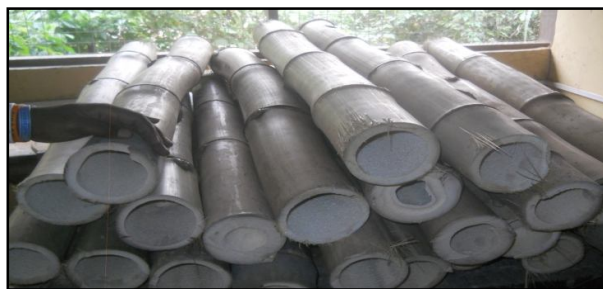
Figure3: Cross cut bamboo ready for splitting
