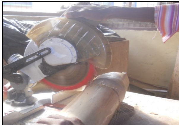
Figure 2: Cutting of the bamboo into lengths of 150cm
