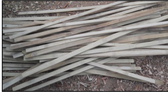
Figure 7: Planed bamboo strips
