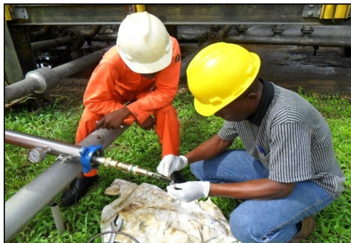
Figure 3: Scraping of biofilms from coupons.
