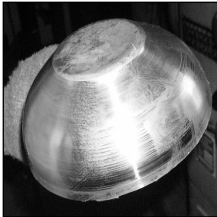
Figure 14: The Spun lower part
