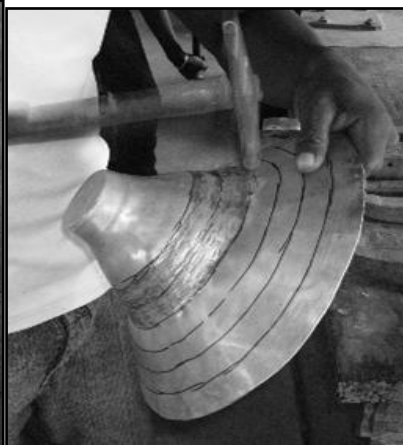
Figure 17: Raising the work on the stake
