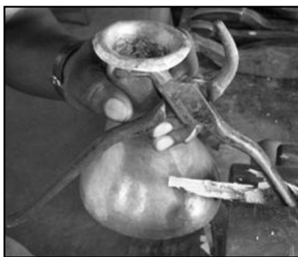
Figure 20: anti-clastically raising the edge
