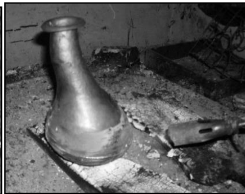
Figure 21: soldering the two parts together.
