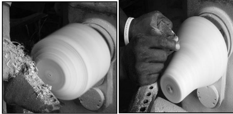
Figure 12: spinning the mould for the bottom Figure 13: the mould for the top part
