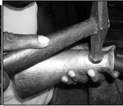
Figure 19: Planishing the work
