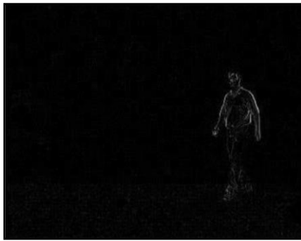
Figure 3(a): Absolute Frame Difference Between 1 st And 2 nd Frames
