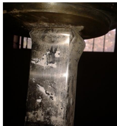
Figure 6 : It Was Observed Splitting Occurred At 1/3^{rd} From The Top
