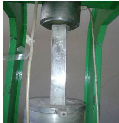
Figure 3: Infilled Steel Tube
