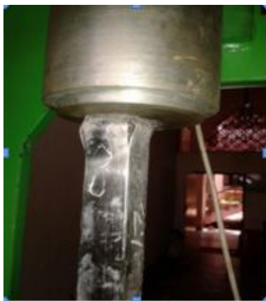
Figure 6 : It Was Observed Splitting Occurred At 1/3^{rd} From The Top
