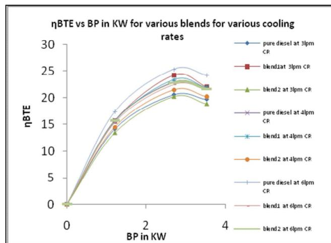
Figure 2: Hbte Vs BP In KW For Various Blends For Various Cooling Rates
