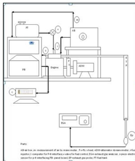
Figure 1: Block Diagram Of The Experimental Setup
