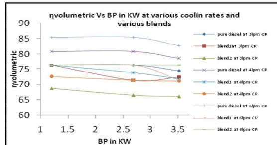
Figure 4: Hvolumetric Vs BP In Kw At Various Cooling Rates And Various Blends
