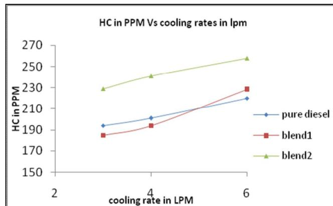
Figure 12: HC In PPM Vs Cooling Rates In Lpm
