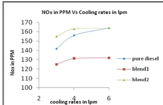
Figure 10: Nox In PPM Vs Cooling Rates In Lpm
