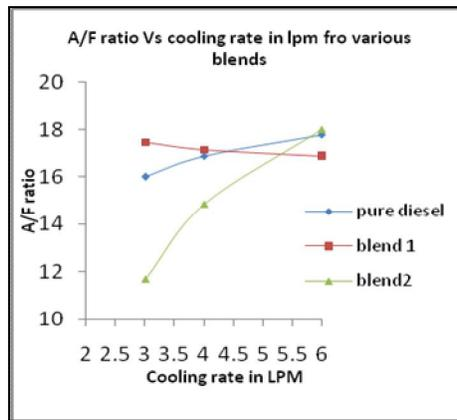
Figure 7: A/F Ratio Vs Cooling Rate In Lpm At Various Blends
