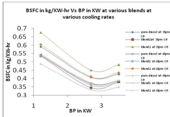
Figure 8: BSFC In Kg/KW-Hr Vs BP In KW At Various Blends At Various Cooling Rates
