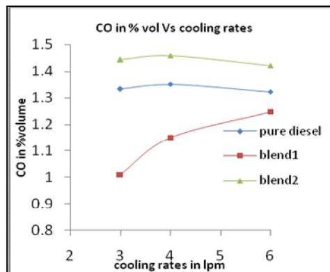
Figure 11: CO In % Vol Vs Cooling Rates
