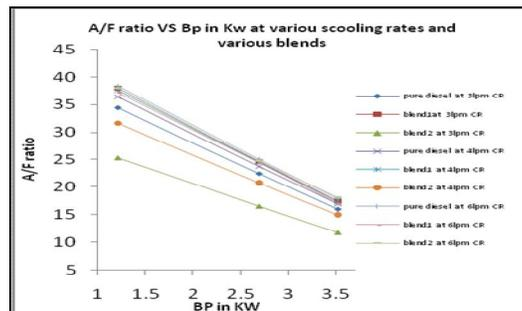
Figure 6: A/F Ratio VS Bp In Kw At Various Cooling Rates And Various Blends
