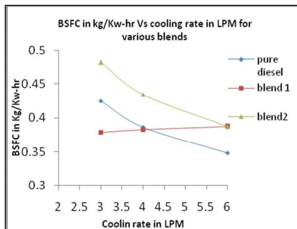
Figure 9: BSFC In Kg/Kw-Hr Vs Cooling Rate In LPM For Various Blends
