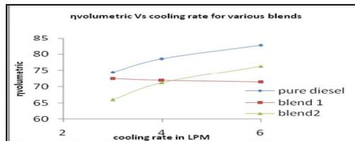
Figure 5: Hvolumetric Vs Cooling Rate For Various Blends
