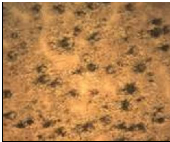
Figure 3: Photomicrograph Of Pearlitic Ductile Iron
