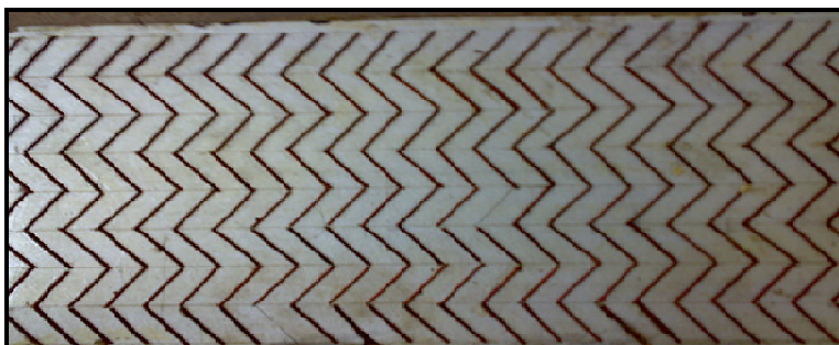
Figure 5(b): 2W Roughened Plate
