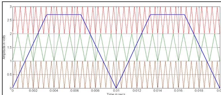
Figure 9: Unipolar Multicarrier Arrangement for VFPWM method with trapezoidal reference ( $m_a=0.9$ ,  $m_{f1}=20$ ,  $m_{f2}=40$ )
