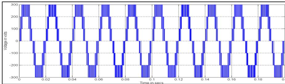
Figure 15 (a): Output Voltage generated by UMCCOPWM method with trapezoidal reference
