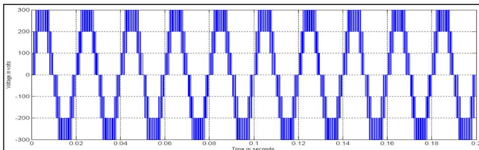
Figure 14 (a): Output Voltage generated by UMCCOPWM method with sine reference
