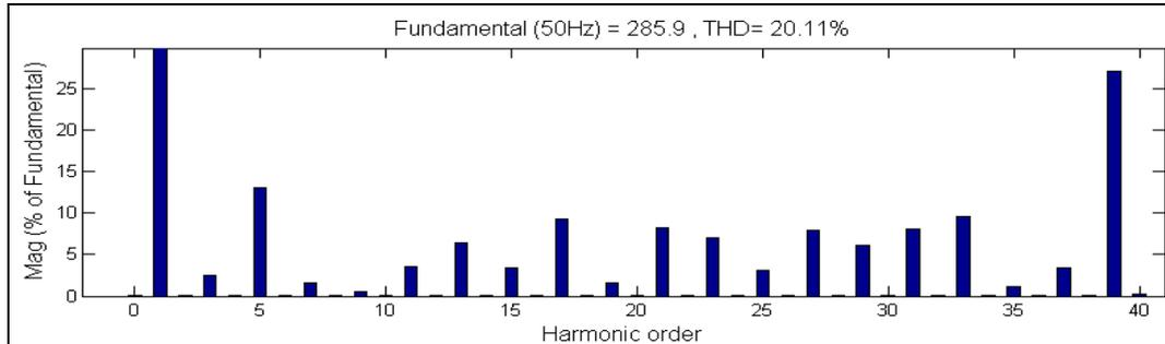
Figure 17 (b): FFT Plot for output voltage of UMCVFPWM method with trapezoidal reference
