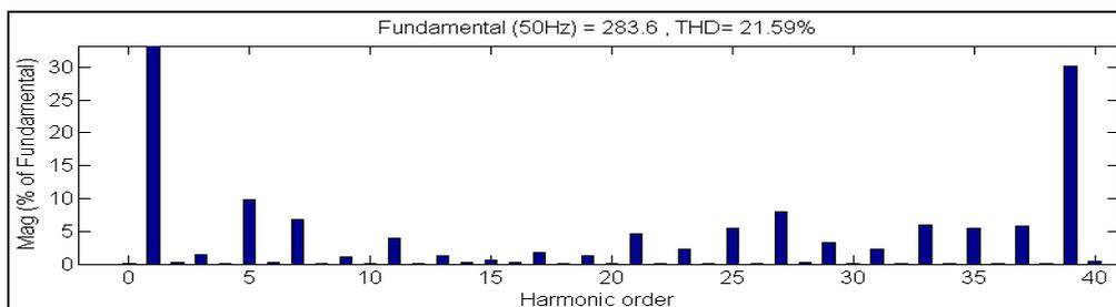
Figure 11 (b): FFT Plot for output voltage of UMCPDPWM method with trapezoidal reference
