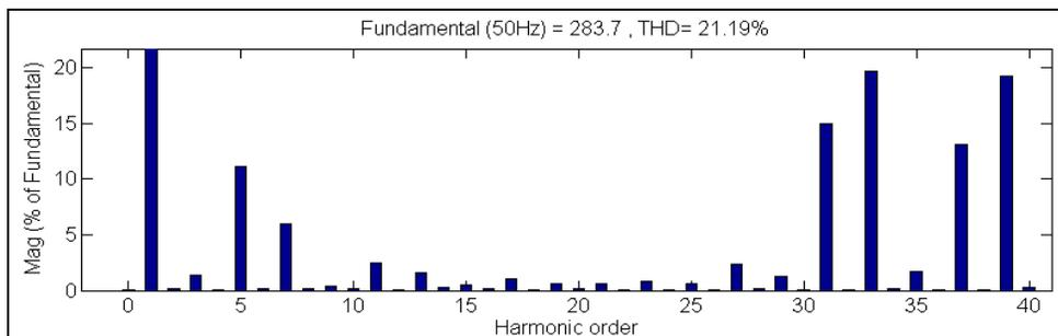
Figure 13 (b): FFT Plot for output voltage of UMCAPODPWM method with trapezoidal reference
