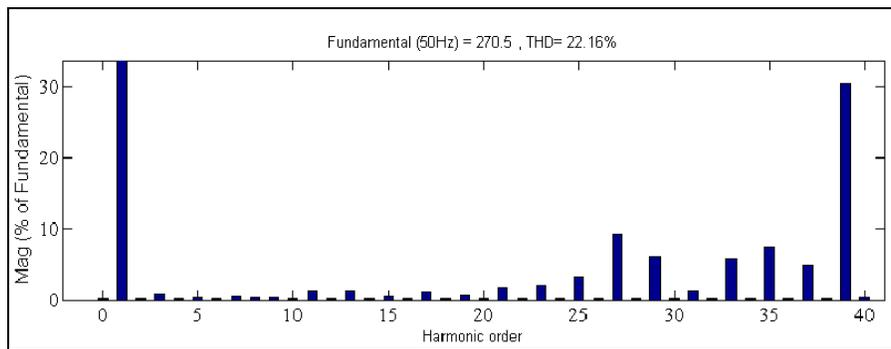
Figure 10 (b): FFT Plot for output voltage of UMCPDPWM method with sine reference
