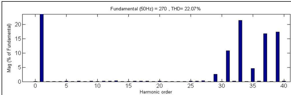
Figure 12 (b): FFT Plot for output voltage of UMCAPODPWM method with sine reference
