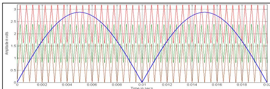
Figure 6: Unipolar Multicarrier Arrangement for COPWM method with sine reference ( $m_a=0.9$  and  $m_f=40$ )
