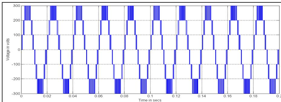
Figure 11 (a): Output Voltage generated by UMCPDPWM method with trapezoidal reference
