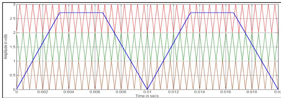
Figure 5: Unipolar Multicarrier Arrangement for APODPWM method with trapezoidal reference ( $m_a=0.9$  and  $m_f=40$ )
