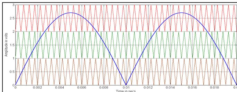
Figure 2: Unipolar Multicarrier Arrangement for PDPWM method with sinusoidal reference ( $m_a=0.9$  and  $m_f=40$ )
