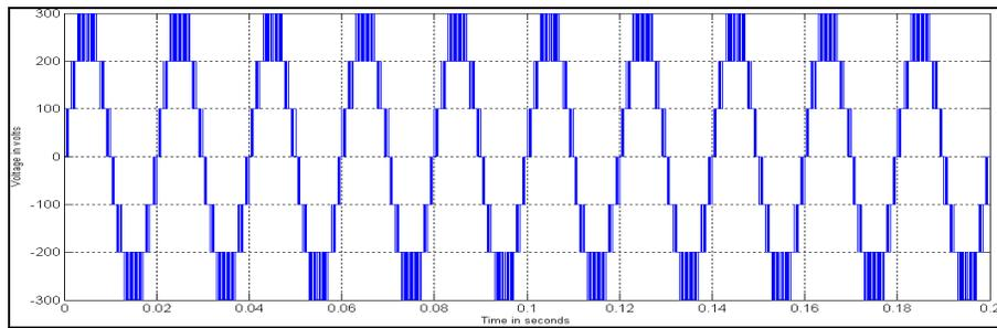
Figure 10 (a): Output Voltage generated by UMCPDPWM method with sine reference
