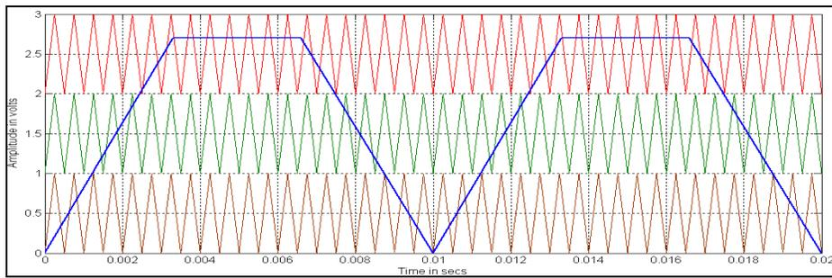
Figure 3: Unipolar Multicarrier Arrangement for PDPWM method with trapezoidal reference ( $m_a=0.9$  and  $m_f=40$ )
