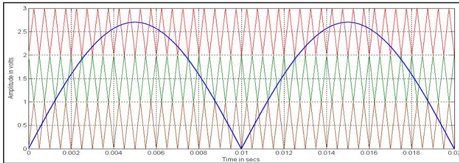
Figure 4: Unipolar Multicarrier Arrangement for APODPWM method with sine reference ( $m_a=0.9$  and  $m_f=40$ )
