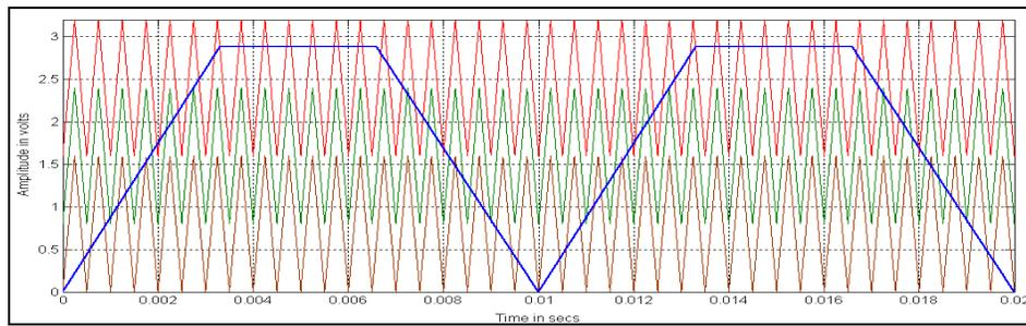
Figure 7: Unipolar Multicarrier Arrangement for COPWM method with trapezoidal reference ( $m_a=0.9$  and  $m_f=40$ )
