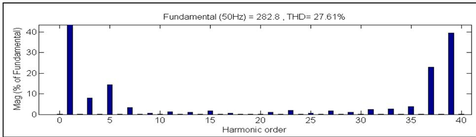
Figure 14 (b): FFT Plot for output voltage of UMCCOPWM method with sine reference
