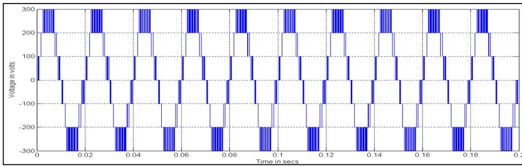
Figure 17 (a): Output Voltage generated by UMCVFPWM method with trapezoidal reference
