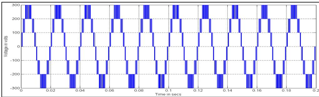
Figure 12 (a): Output Voltage generated by UMCAPODPWM method with sine reference
