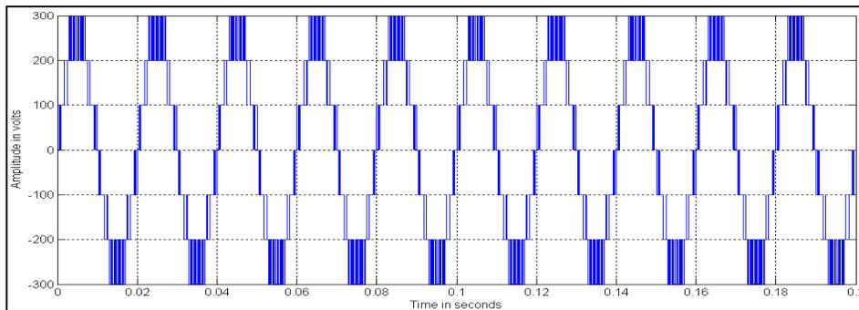
Figure 16 (a): Output Voltage generated by UMCVFPWM method with sine reference
