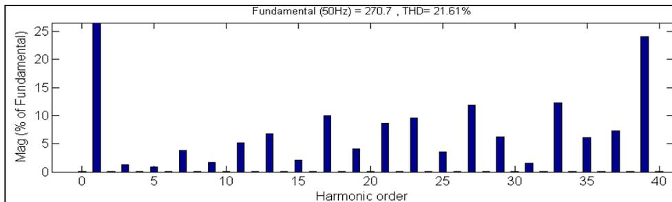
Figure 16 (b): FFT Plot for output voltage of UMCVFPWM method with sine reference
