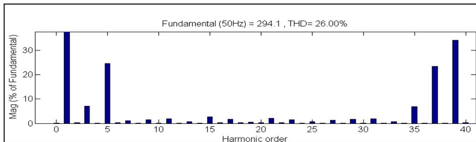
Figure 15 (b): FFT Plot for output voltage of UMCCOPWM method with trapezoidal reference
