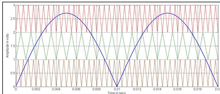
Figure 8: Unipolar Multicarrier Arrangement for VFPWM method with sine reference ( $m_a=0.9$ ,  $m_{f1}=20$ ,  $m_{f2}=40$ )
