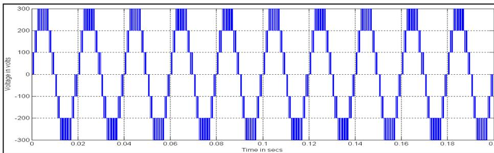
Figure 13 (a): Output Voltage generated by UMCAPODPWM method with trapezoidal reference
