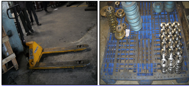
Figure 2: Pallet and Pallet Truck Can Be Used For Lighter Material Movement
