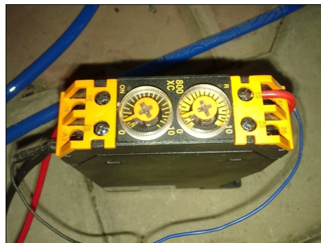
Figure 7: Timer relay circuit (controller)
