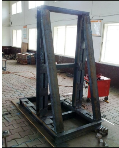
Figure 4.3: Reaction frame on base frame
