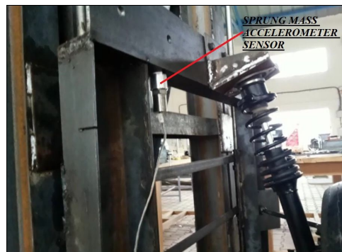
Figure 9: Sensor on sprung mass
