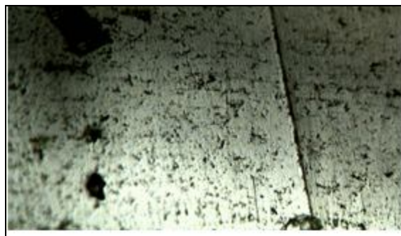
Figure 2: Metal Surface before action (non corroded) of 1M HCl acid
