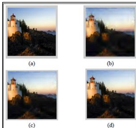
Figure 4: Figure showing (a) house image (b) Recons-trusted Image at 0.1bpp (c) Reconstructed Image at 0.25 bpp (d) Reconstructed Image at 0.5 bpp
