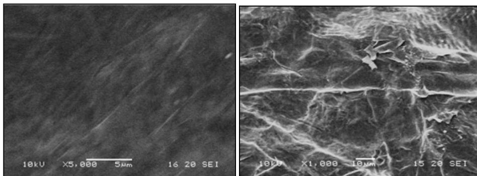
Figure 1: Scanning electron micrographs of (a) bare EG electrode, (b) DNA modified EG pellets
