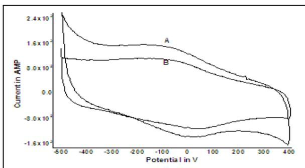
Figure 2: Cyclic voltammograms of cytochrome *c* in 0.1 M PBS of pH 7.0: (a) bare EG (b) DNA modified EG electrode
