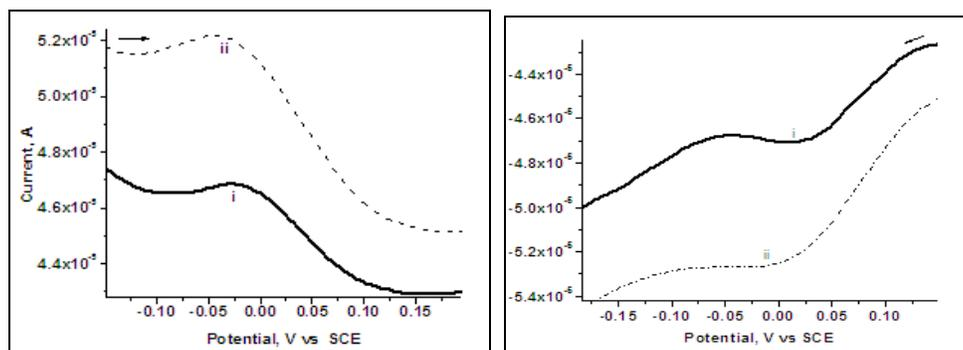
Figure 4: a) Anodic and b) Cathodic DPVs of 0.2 mM *cyt c* in 0.1M PBS of pH 7 On i) bare EG & ii) DNA modified exfoliated graphite electrode.
