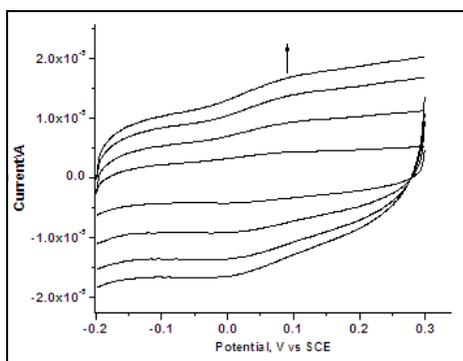
Figure 3: Cyclic voltammograms of 0.2 mM *cyt c* on DNA modified electrode with different concentrations of DNA (2, 4, 6, 8, 10  $\mu$ l) in 0.1 M PBS, pH 7.0, and scan rate: 50 mV/s
