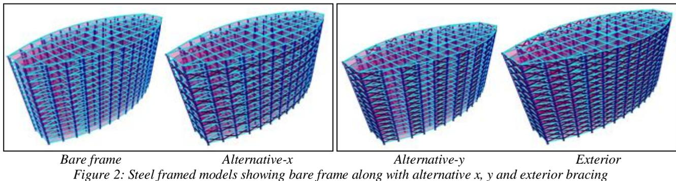
Figure 2: Steel framed models showing bare frame along with alternative x, y and exterior bracing
