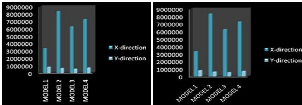
Figure 5: Graphical Representation of Stiffness of ISMB models
