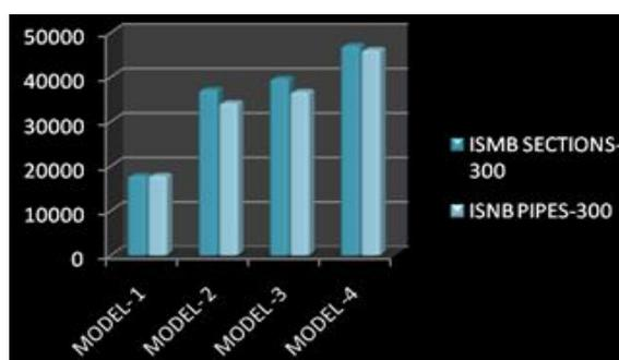
Figure 4: Design base shear of different bracing models (push-X)
