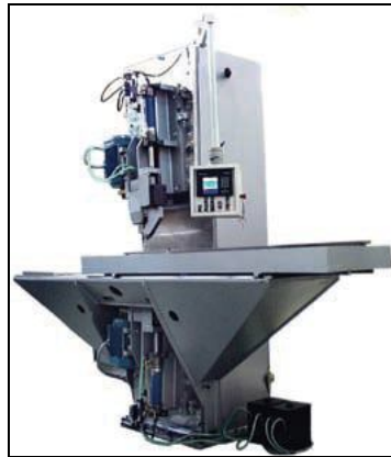
Figure 10: ESAB Super Stir unit at Tower automotive [6]
