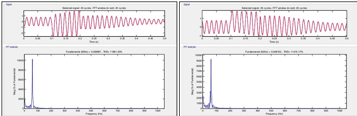
Figure 11: FFTs of the induction motor phase B phase to ground fault for phase B
