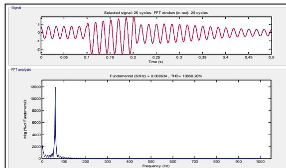
Figure 15: FFTs of the induction motor phase C phase to ground fault for phase C
