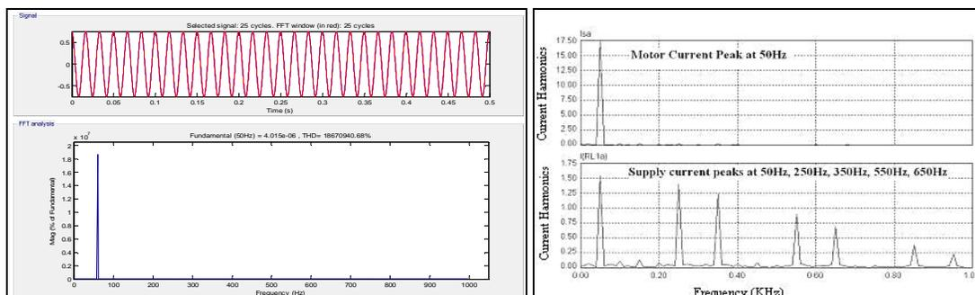
Figure 5: Magnitude vs Frequency plot of healthy induction motor for phase C.
