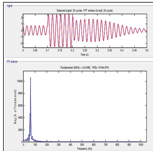
Figure 18: FFTs of the induction motor where all three phase ground fault for phase C
