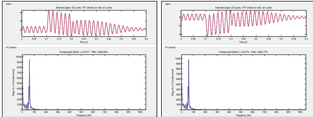
Figure 16: FFTs of the induction motor where all three phase ground fault for phase A
