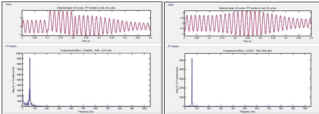
Figure 13: FFTs of the induction motor phase C phase to ground fault for phase A
