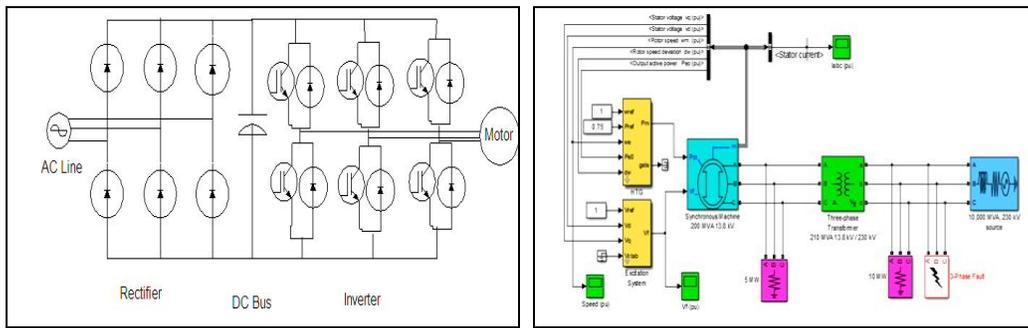
Figure 1: Block diagram of induction motor drive system
