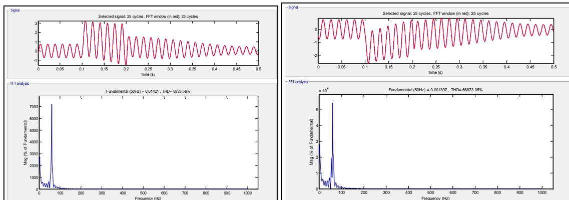
Figure 7: FFTs of the induction motor phase A phase to ground fault for phase A
