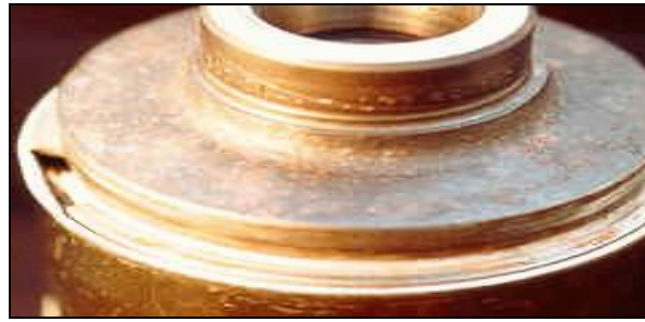
A ruptured welded neck flange
