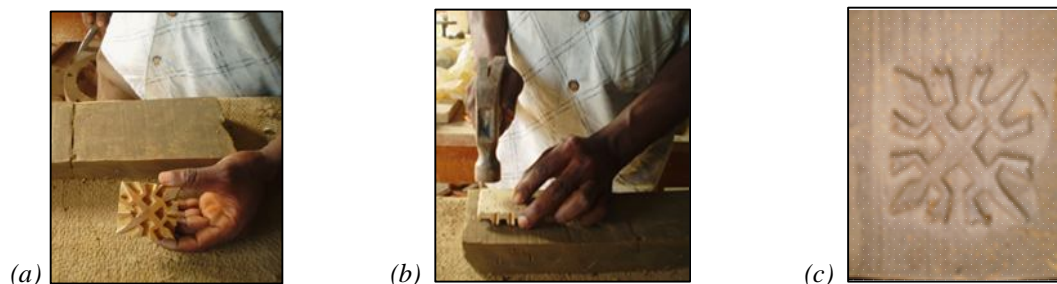
Figure 6: (a): Template for Embossment (b) Template been hammered on tile (c) Embossed symbol
