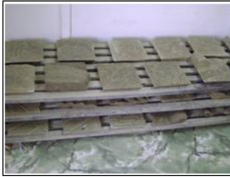
Figure 9: Fig.5: Drying of tile on shelves
