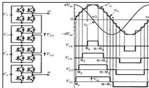
Figure 2: Single phase 9 level H-bridge inverter and switching strategies
