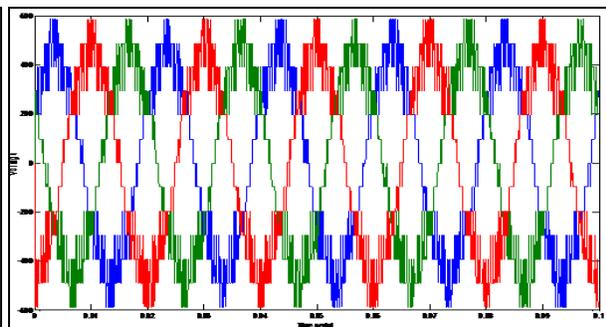
Figure 4: Output voltage of 9 level VSC
