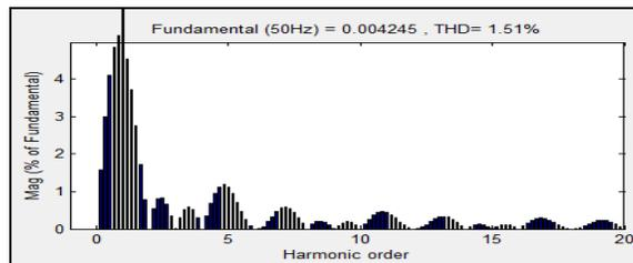
Figure 16: THD of output current (with 13-level STATCOM)
