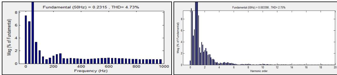
Figure 13: FFT analysis of power system without STATCOM
