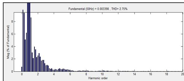
Figure 10: FFT analysis of multilevel STATCOM
