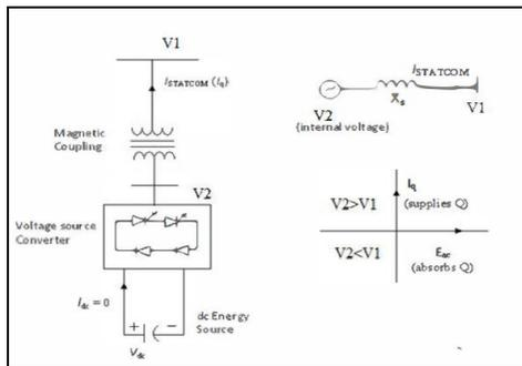
Figure 1: Schematic Configuration of STA COM
