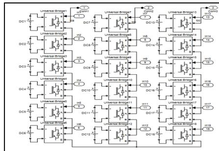
Figure 15: 13-Level Cascade H-Bridge multilevel Inverter
