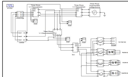
Figure 7: Simulink model of multilevel STATCOM
