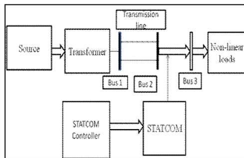
Figure 6: Block diagram of power system with STATCOM.
