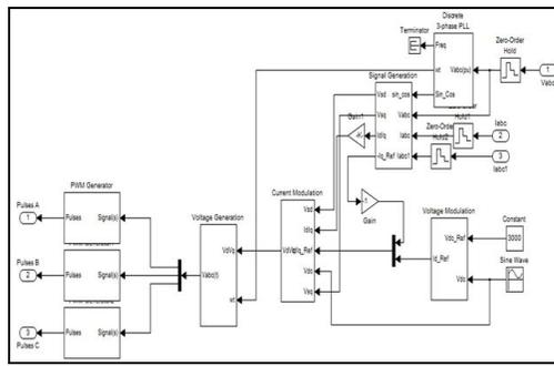
Figure 5: Simulation model of STATCOM Controller
