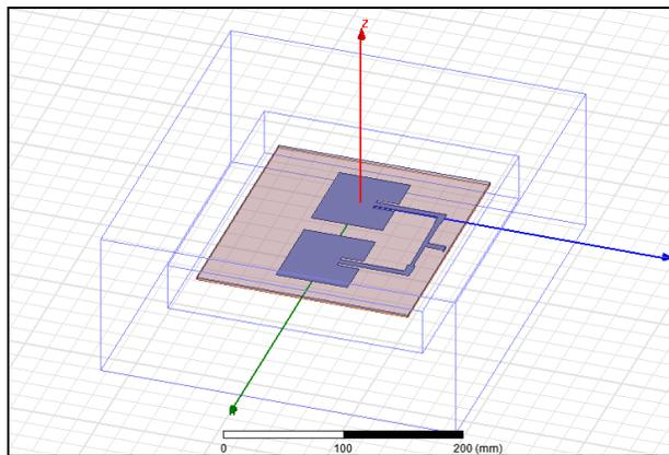
Figure 9: HFSS model of Inset fed linear rectangular patch array (1\*2)
