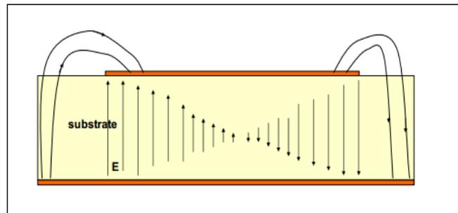
Fig. 2 Radiation mechanism of patch antenna
