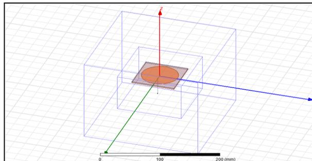
Figure 5: HFSS model for Probe-fed elliptical patch antenna
