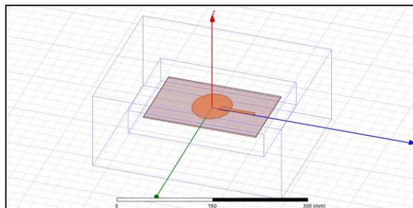
Figure 6: HFSS model for Inset-fed elliptical patch antenna
