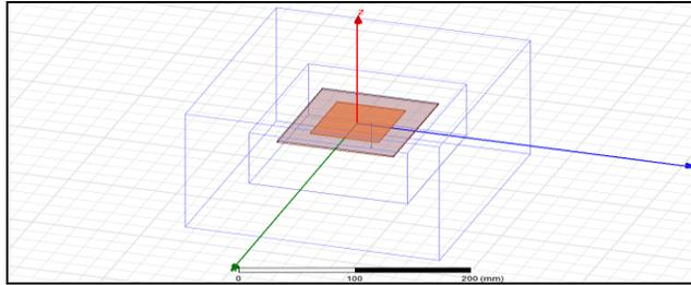
Figure 3: HFSS model for Probe-fed rectangular patch antenna
