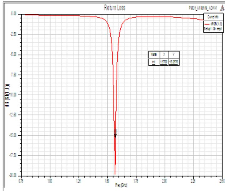
Figure 12: Return loss plot of inset fed rectangular patch antenna
