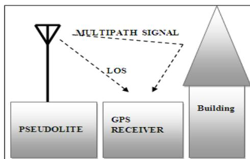
Figure1: Illustration of Multipath effect
