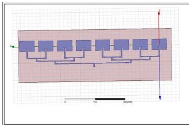
Figure 11: HFSS model of Inset fed linear rectangular patch array (1\*8)
