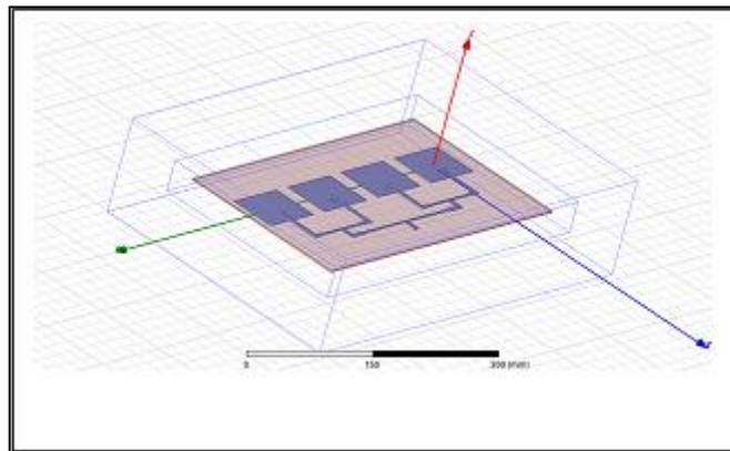
Fig .10 HFSS model of Inset fed linear rectangular patch array (1\*4)
