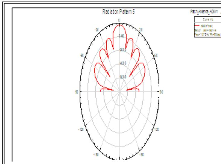
Figure 17: Radiation pattern for Inset-fed rectangular patch antenna at  $d=0.4\lambda$
