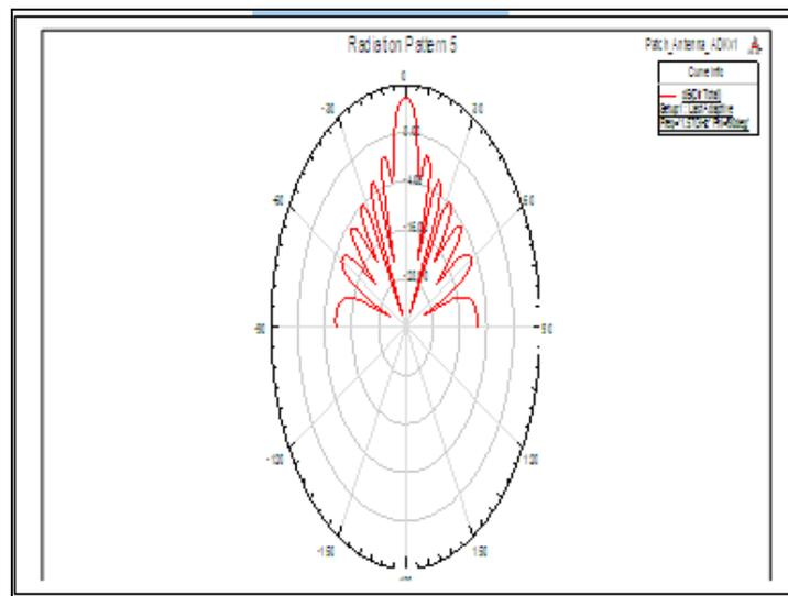
Fig .18 Radiation pattern for Inset-fed rectangular patch antenna at  $d=0.8\lambda$
