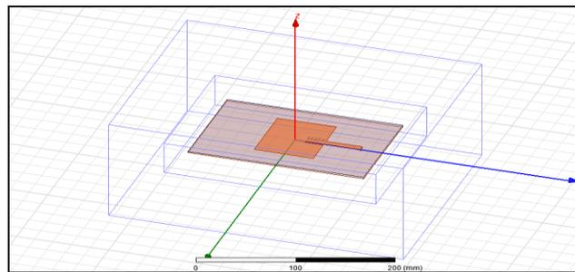
Figure 4: HFSS model for Inset-fed rectangular patch antenna
