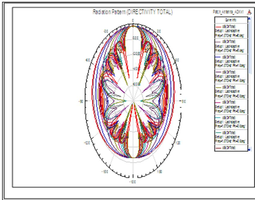
Figure 16: Directivity radiation pattern for N=8 for Inset-fed rectangular patch antenna
