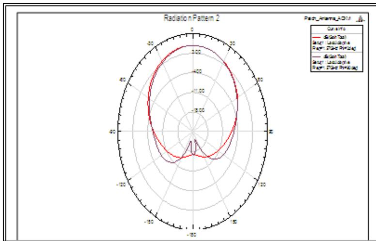
Figure 14: Gain radiation pattern for Inset-fed rectangular patch antenna
