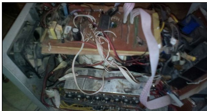
Figure 7: The constructed inverter-AVR circuit boards
