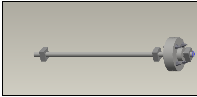
Figure 2: Solid model of flexible flange coupling and rotor shaft assembly for bent driven shaft at coupling end
