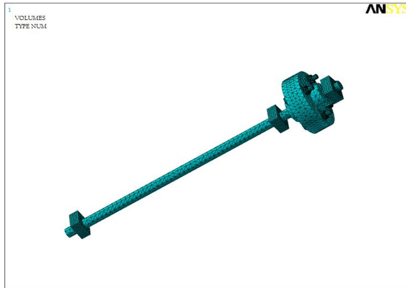
Figure 3: Meshed model of shaft coupling assembly
