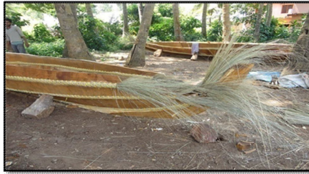
Figure 1: Representation of stitched boats showing X-pattern stitching in longitudinal and transverse direction.
