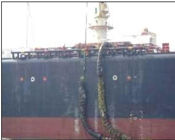
Figure 3: Hose Connection onboard tanker
