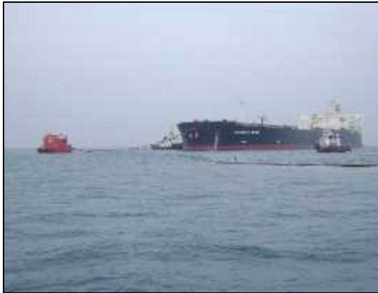
Figure 1: Tanker Mooring at SPM Tanker
