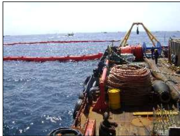
Figure 4: Deployment Oil Spill Containment Boom
