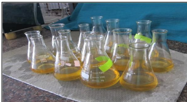
Figure 1: Diesel: Ethanol: EthylAcetate Microemulsions
