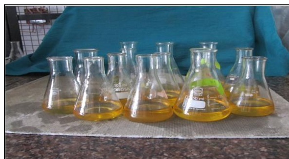
Figure 3: Diesel: Ethanol: Biodiesel Microemulsions
