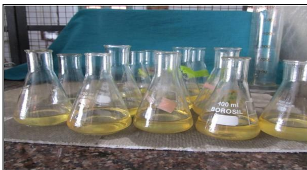
Figure 2: Diesel: Ethanol: 1-Octanol Microemulsions
