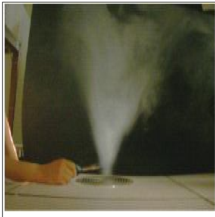
Figure 9: Smoke visualization of the airflow pattern from the swirl diffuser
