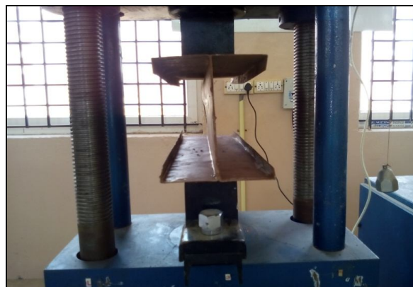
Figure 4: SPECIMEN 1-B-BLCS 142 without web holes
