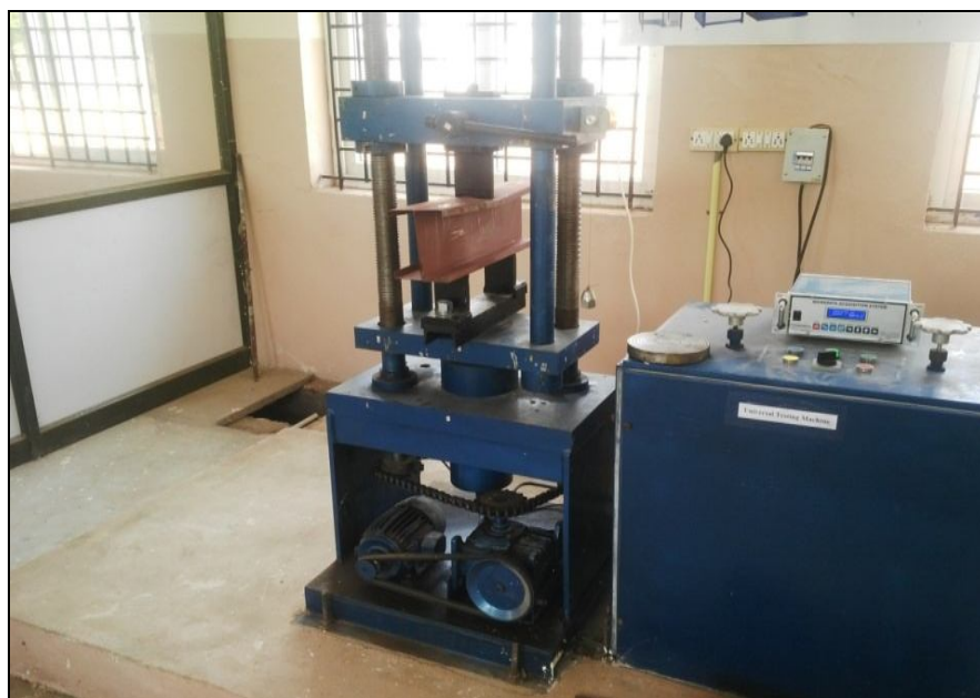
Figure 1: concentrated loading condition without web holes
