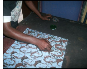
Figure 17: Scratching of fabric with broomsticks. Figure 18: Broomsticks with paste.
