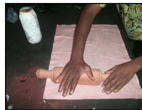
Figure 32: Rolling of fabric to effect transfer.
