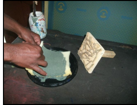
Figure 19: Twigs block with print paste. Figure 20: Printing with twigs block.
