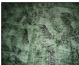
Figure 41: Printed fabric from brush printing technique.
