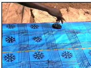
Figure 4a: a traditional Calabash stamping with Adinkra dye paste used for Adinkra cloth
