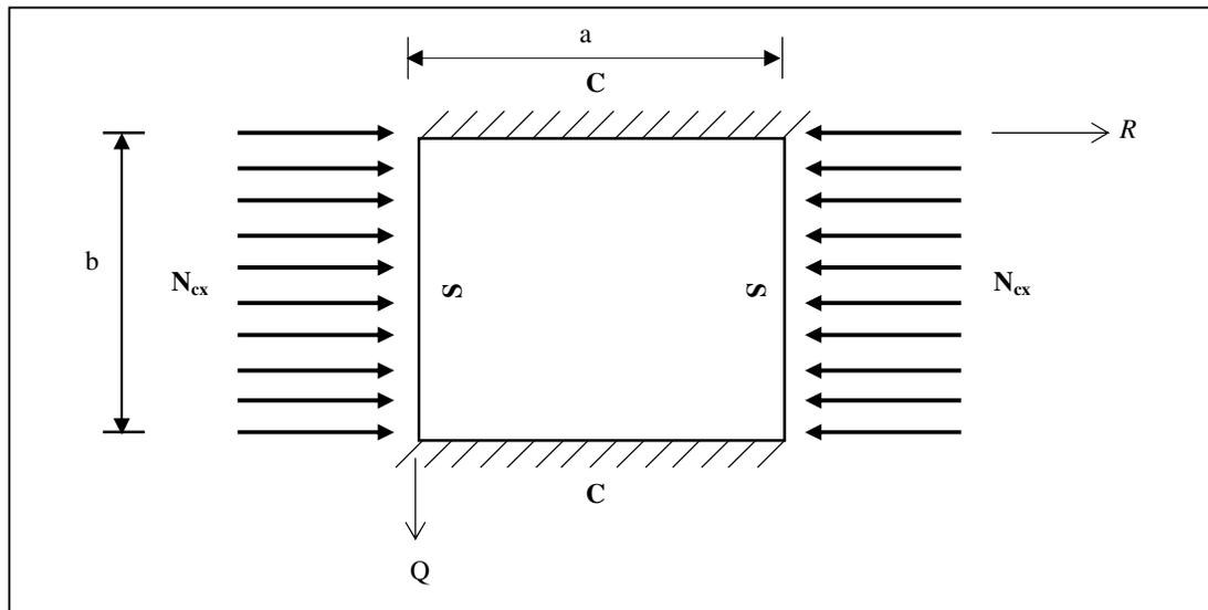
Figure 2: CSCS – Thin Rectangular Plate under Uniaxial Load
