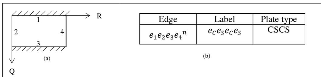
Figure 1: Procedure for naming plate with different edge conditions
