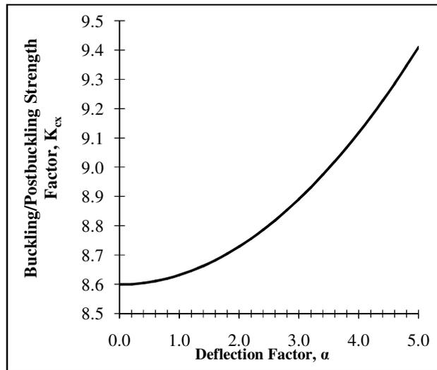
Figure 3: Buckling and Postbuckling Load Coefficient,  $K_{cx}$  and Deflection Factor,  $\alpha$  at aspect ratio of unity for CSCS – Plate
