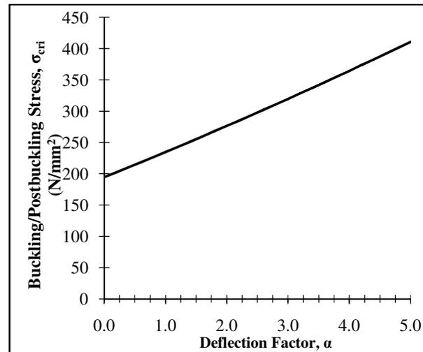
Figure 4: Buckling and postbuckling load critical yield/maximum stress,  $\sigma_{cri}$  and deflection Factor,  $\alpha$  at aspect ratio of unity for CSCS – Plate
