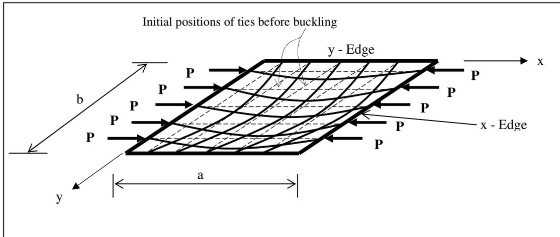
Figure 2: Post-buckling model of a thin plate under in-plane loads
