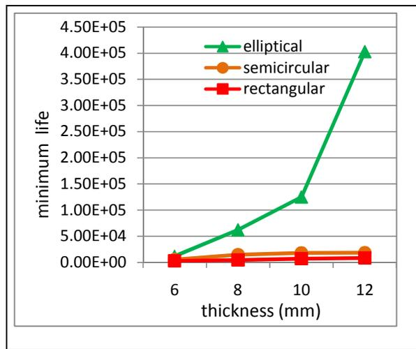
Figure 29: Fatigue life vs thickness for various exit geometry
