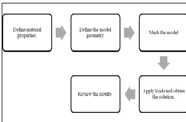
Figure 4: Flow Diagram of thermal analysis in ANSYS
