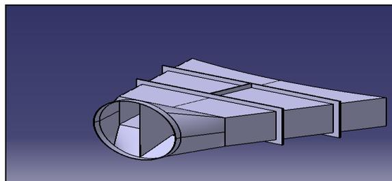
Figure 15: model of nozzle with stiffeners
