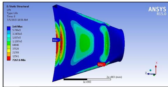
Figure 8: Fatigue life of nozzle made of Carbon steel (12 mm thickness)
