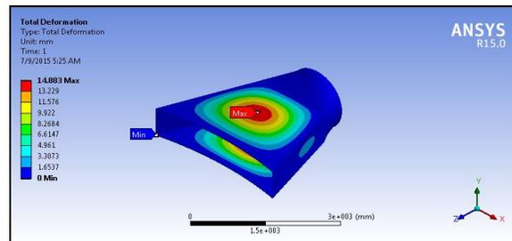
Figure 10: Deformation of nozzle with SS 309 S as material (12 mm thickness)
