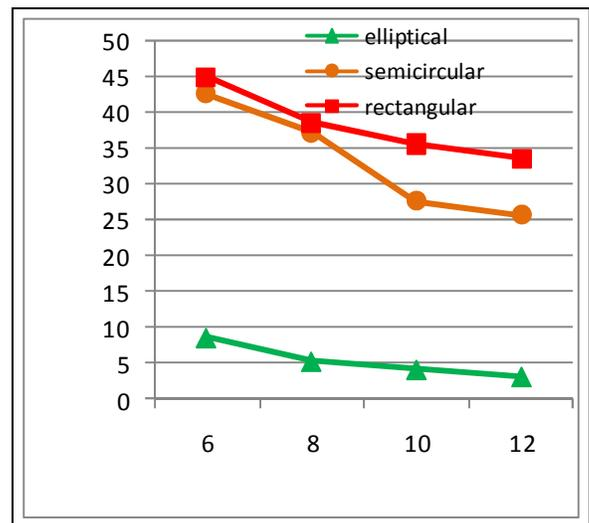
Figure 28: Deformation vs thickness for various exit geometry
