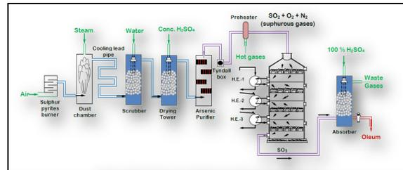
Figure 1: Manufacturing of Sulphuric acid by Contact process
