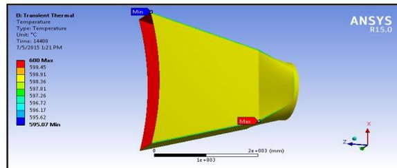
Figure 5: Temperature distribution of Nozzle made of Carbon steel (12mm thickness)
