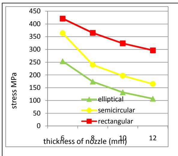
Figure 27: Stress vs thickness for various exit geometry
