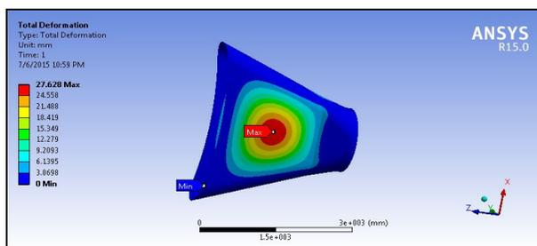
Figure 22: Deformation of nozzle with semicircular profile (8mm thickness)
