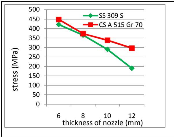
Figure 12: Maximum stress level vs thickness of nozzle
