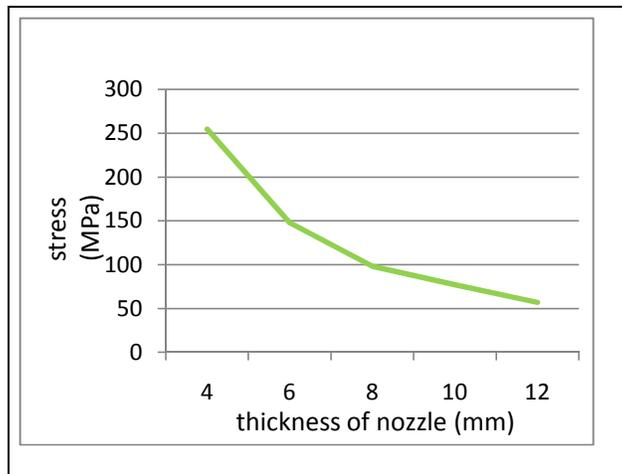
Figure 19: Maximum stress vs thickness of nozzle with stiffeners
