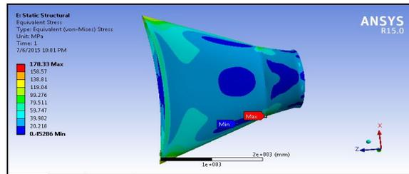
Figure 24: Stress distribution of nozzle of elliptical profile with 8mm thickness
