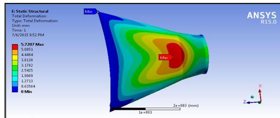
Figure 25: Deformation of nozzle of elliptical profile with 8mm thickness
