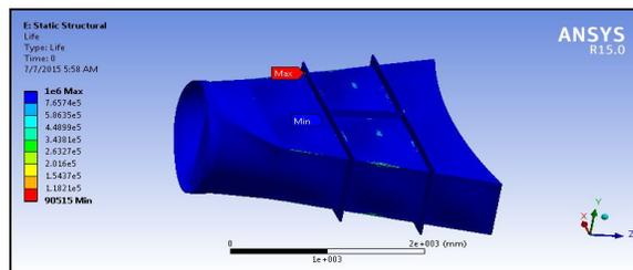
Figure 18: Fatigue life of nozzle with stiffeners (6mm thickness)
