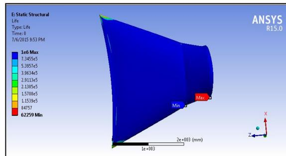
Figure 26: Fatigue life of nozzle of elliptical profile with 8mm thickness
