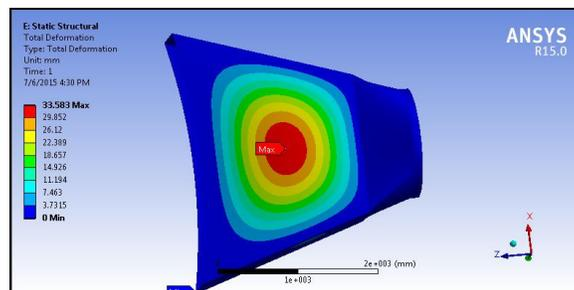
Figure 7: Deformation of nozzle made of carbon steel (12 mm thickness)
