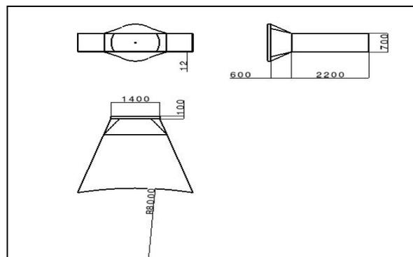
Figure 2: 2D drawing of nozzle
