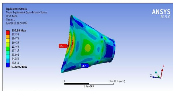
Figure 21: Stress distribution of nozzle with semicircular exit profile (8mm thickness)
