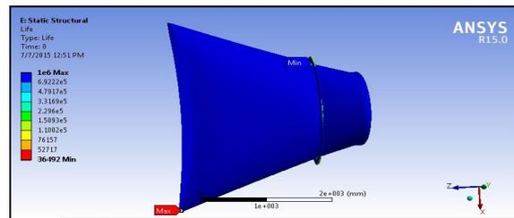
Figure 32: Fatigue life of nozzle of elliptical profile with stiffener (6mm thickness)
