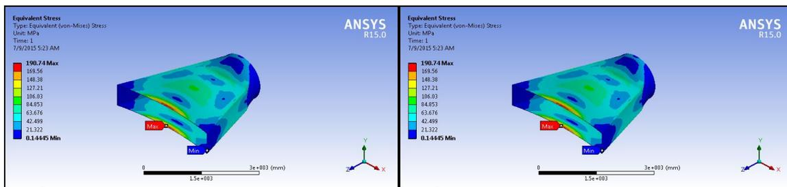
Figure 9: Stress distribution of nozzle with SS 309 S as material (12 mm thickness)
