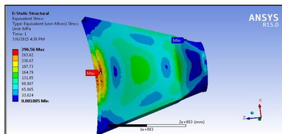
Figure 6: Stress distribution of nozzle made of carbon steel (12 mm thickness)
