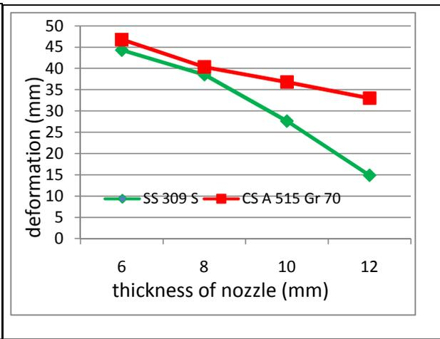
Figure 13: Deformation vs thickness of nozzle
