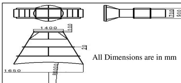
Figure 20: 2D Drawing of proposed model with stiffeners
