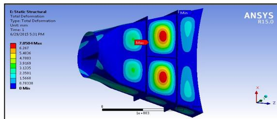
Figure 17: Deformation of nozzle with stiffeners (6mm thickness)
