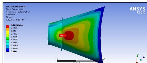
Figure 31: Deformation of nozzle of elliptical profile with stiffener (6mm thickness)
