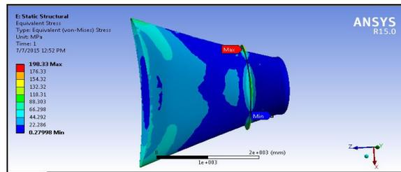
Figure 30: Stress distribution of nozzle of elliptical profile with stiffener (6mm thickness)
