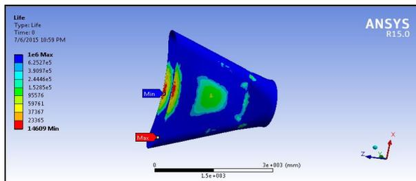
Figure 23: Fatigue life of nozzle with semicircular profile (8mm thickness)
