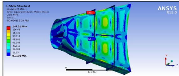
Figure 16: Stress distribution of nozzle with stiffeners (6mm thickness)
