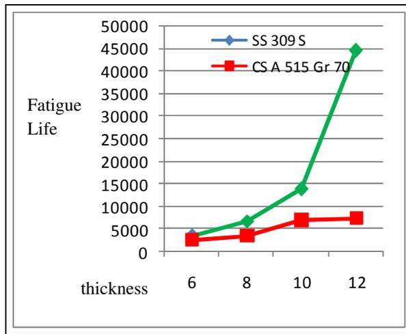
Figure 14: Fatigue life vs thickness of nozzle.
