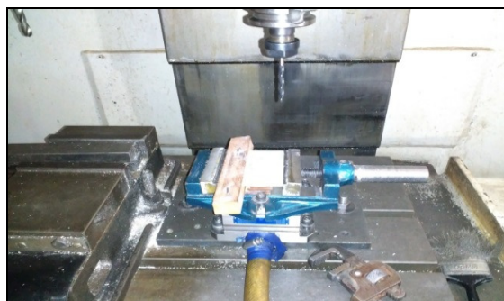
Figure 3: Dynamometer attached with work piece on the CNC drilling machine
