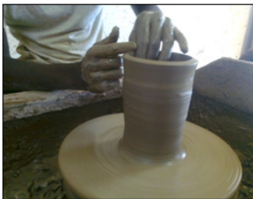
Figure 18: Pulling of height of the vase.
