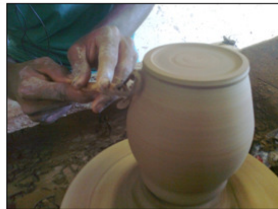
Figure 23: trimming of excess clay from the vase.
