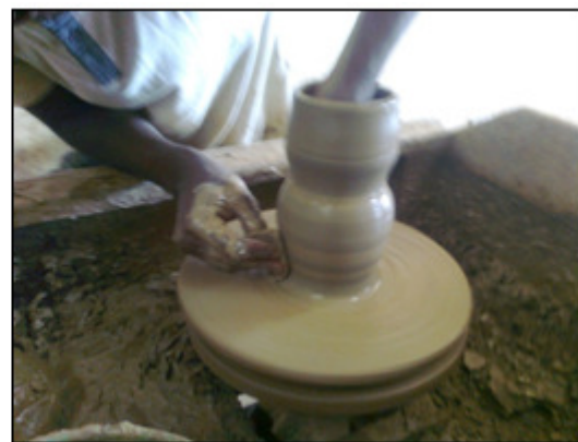
Figure 19: Initial shaping of the vase.
