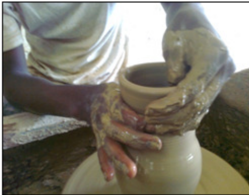
Figure 20: Final shaping of the clay vase.
