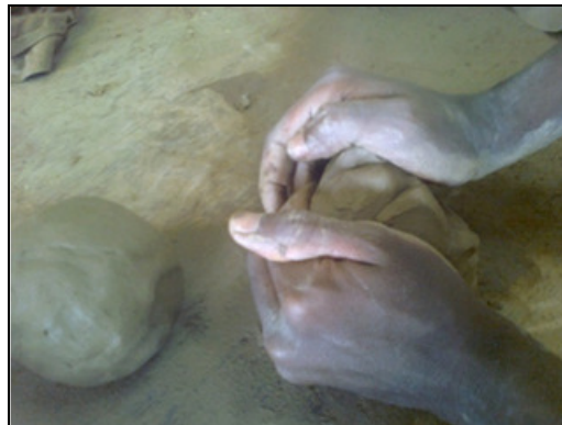
Figure 15: Kneading the clay into lumps.
