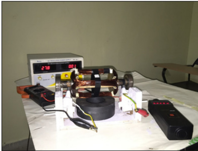
Figure 1: Constructional features of the prototype coreless DC motor and the test set-up
