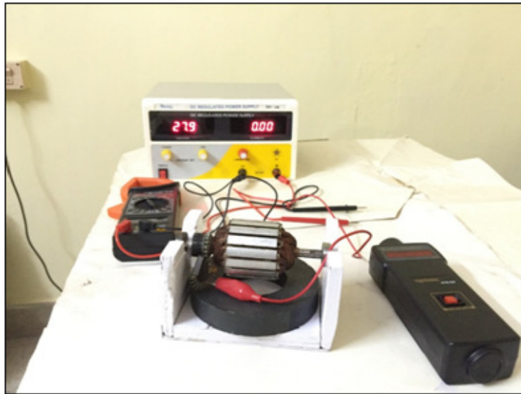
Figure 2: Cored PMDC motor used for comparative analysis of performance
