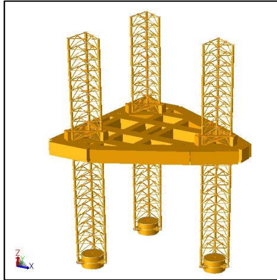
Figure 1: Three Dimensional FE Model of the Rig
